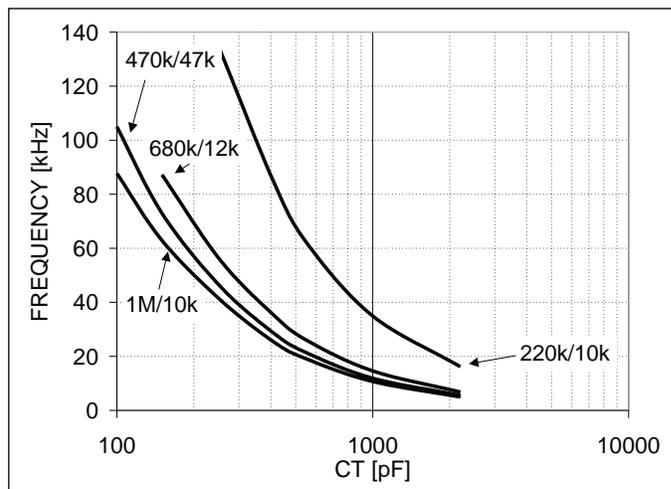
Figure 6. Frequency vs. CT vs. RT1 and RT2.
