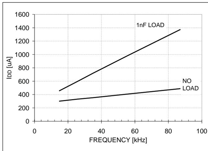
Figure 8. IDD vs. frequency RT1 = 680k, RT2 = 12k.
