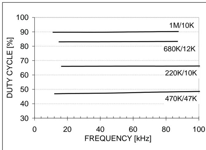
Figure 7. Duty cycle vs. frequency vs. RT1 / RT2.
