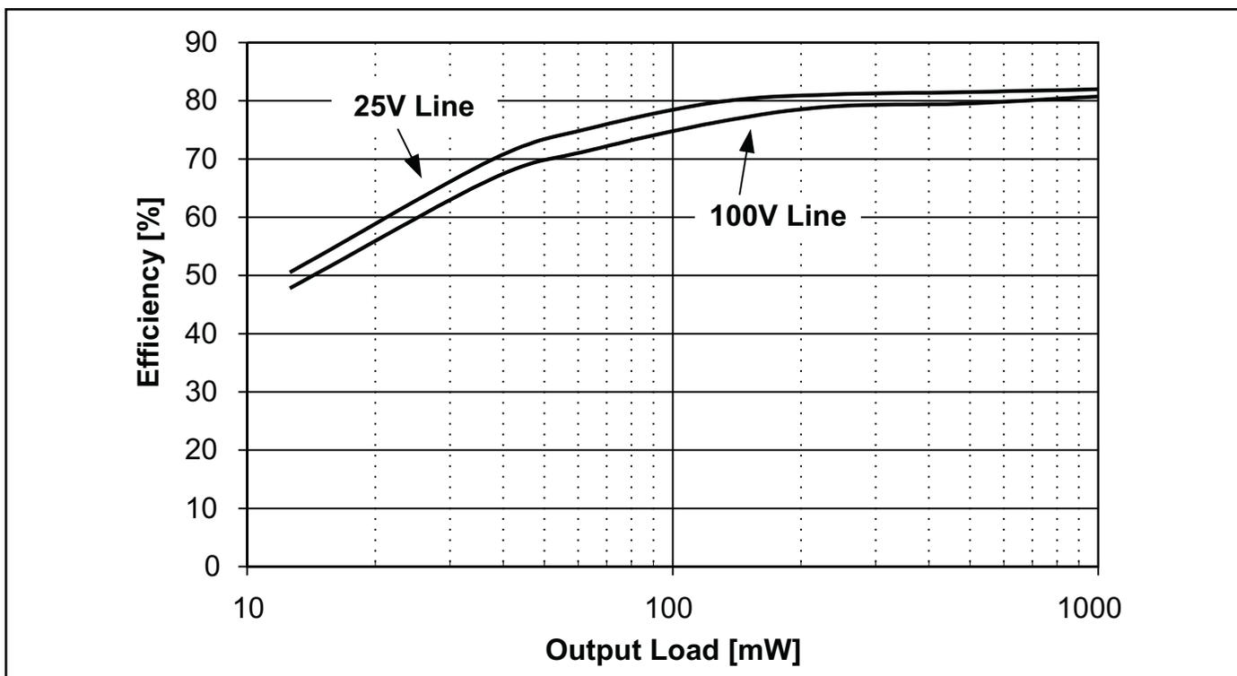
Figure 4. UCC3581 efficiency vs. line and load.
