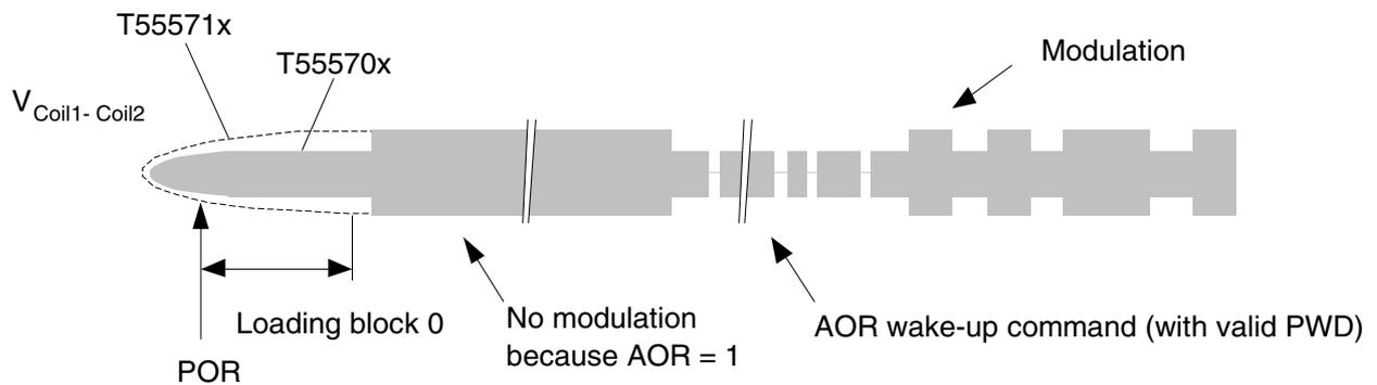
**Figure 13.** Coil Voltage after Programming of a Memory Block
