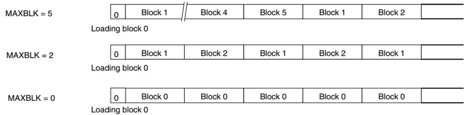
Every time the T5557 enters regular- or block-read mode, the first bit transmitted is a logical '0'. The data stream starts with block 1, bit 1, continues through MAXBLK, bit 32, and cycles continuously if in regular-read mode.
