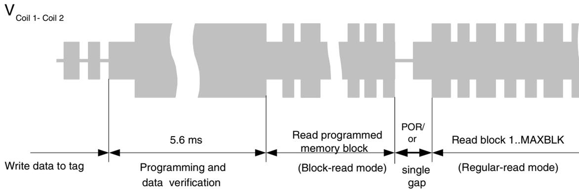
Figure 14. Anticollision Procedure Using AOR Mode
