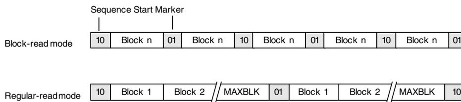
The T5557 sequence start marker is a special damping pattern, which may be used to synchronize the reader. The sequence start marker consists of two bits ('01' or '10') which are inserted as header before the first block to be transmitted if the bit 29 in extended mode is set. At the start of a new block sequence, the value of the two bits is inverted.
