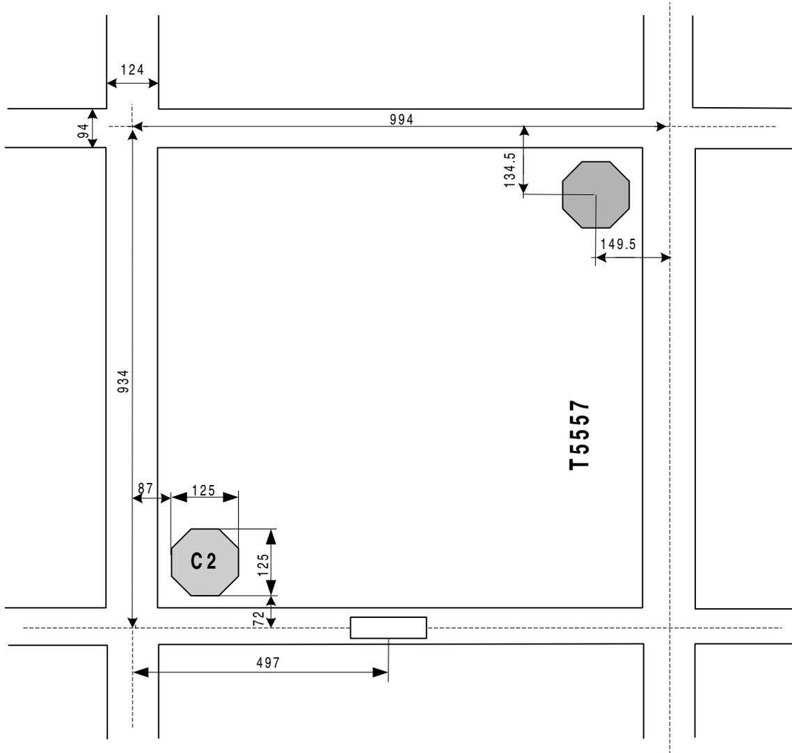
Figure 27. 4 Pad Flip-chip Version with 70 μm Solder Bumps
