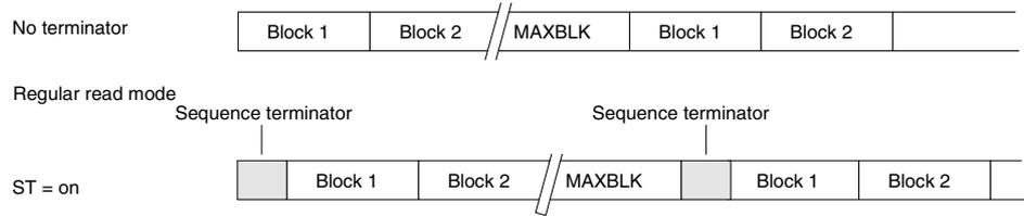
**Figure 8.** e5550-compatible Sequence Terminator Waveforms
