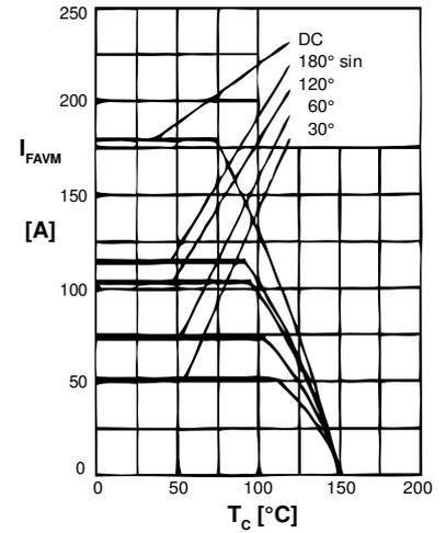
Fig. 3 Maximum forward current at case temperature
