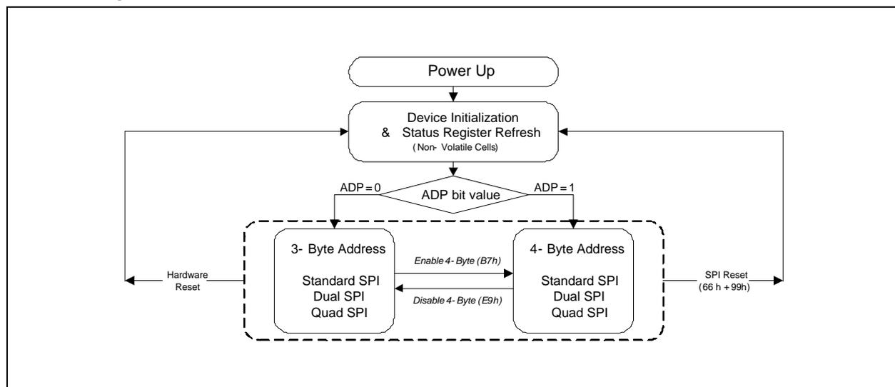
Figure 3. W25Q256JW Serial Flash Memory Operation Diagram
