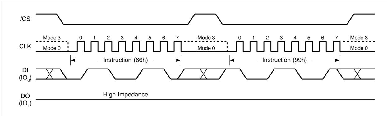
Figure 60. Enable Reset and Reset Instruction Sequence
