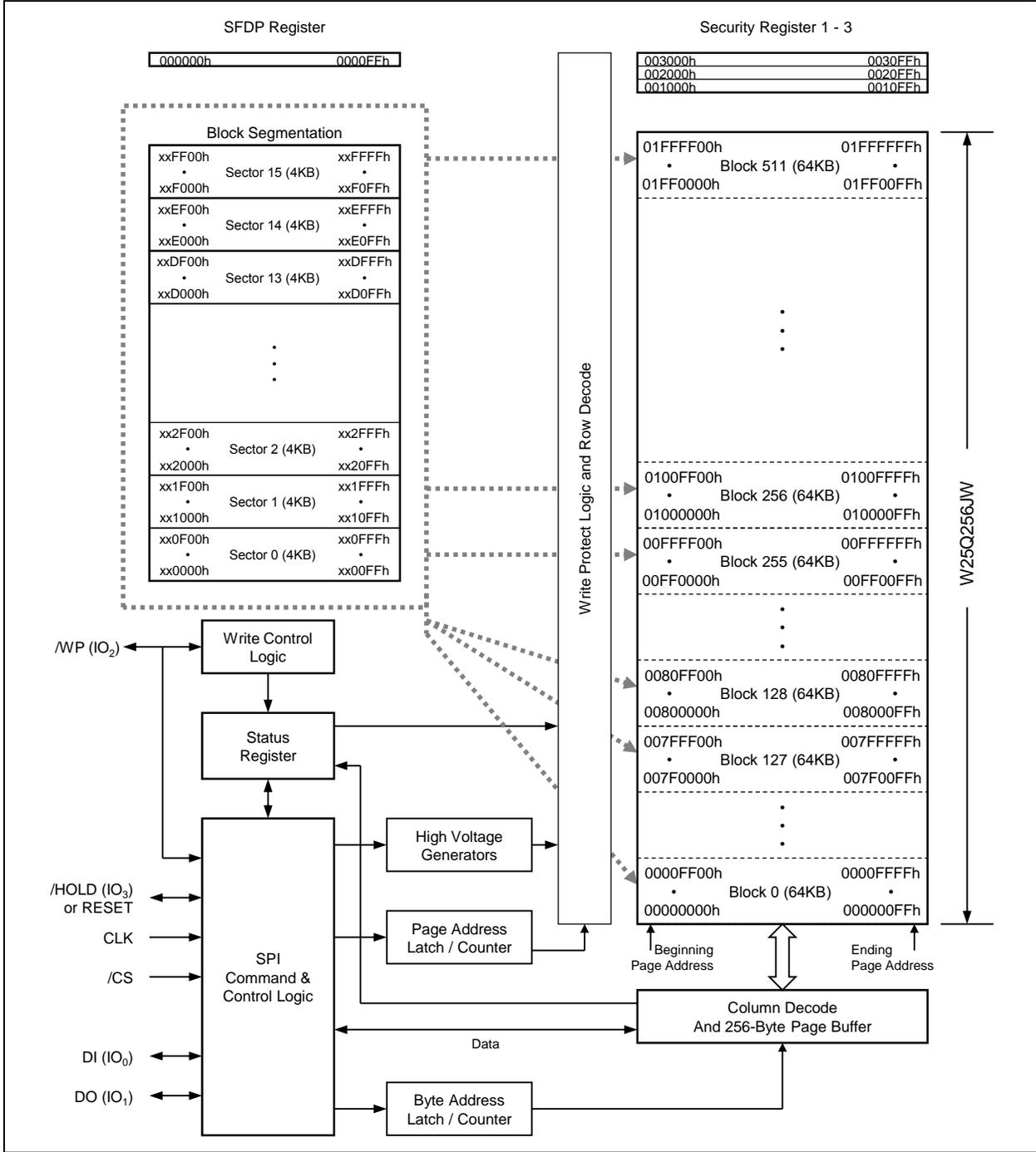
Figure 2. W25Q256JW Serial Flash Memory Block Diagram
