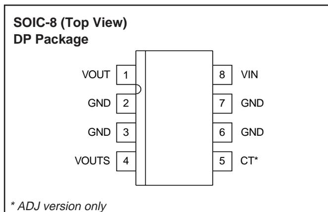
The UCC381 can be shutdown to 25μA (max) by pulling the CT pin low.
