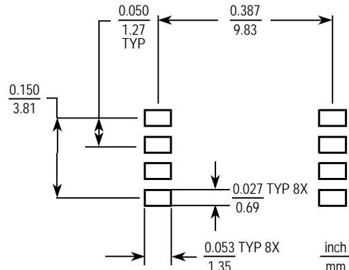
Figure 4. SSOP Footprint (Case 1317 and 1317A)
