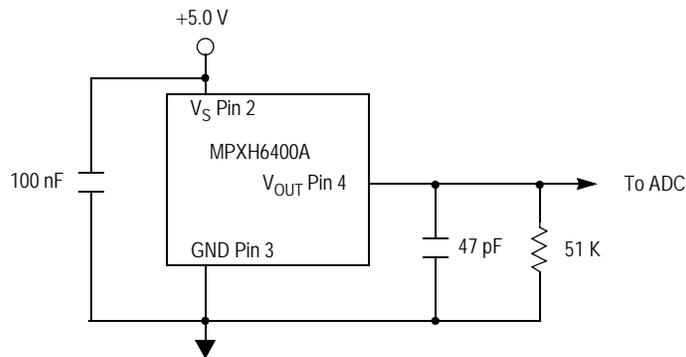
**Figure 2. Typical Application Circuit (Output Source Current Operation)**
