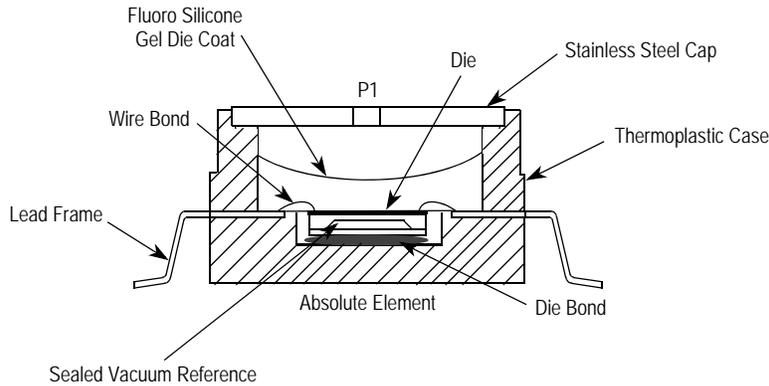
**Figure 1. Cross Sectional Diagram SSOP (not to scale)**
