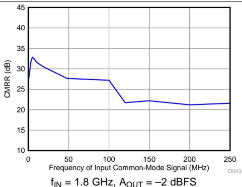
Figure 67. Common-Mode Rejection Ratio vs Tone Frequency
