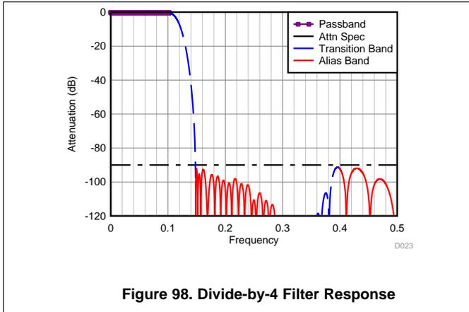
Figure 98. Divide-by-4 Filter Response
