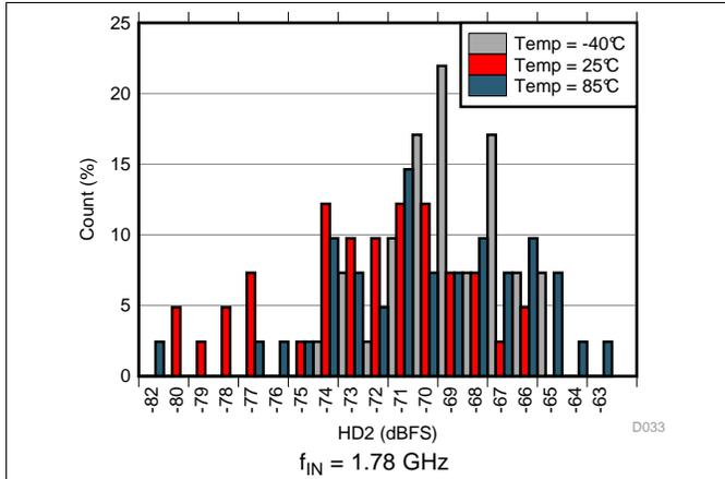
Figure 57. HD2 Histogram at AVDD19 = 2.0 V
