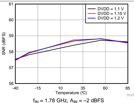
Figure 47. Signal-to-Noise Ratio vs DVDD Supply and Temperature
