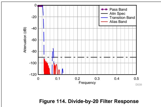
Figure 114. Divide-by-20 Filter Response
