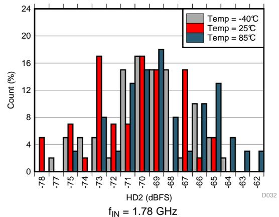
Figure 56. HD2 Histogram at AVDD19 = 1.9 V
