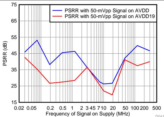
Figure 65. Power-Supply Rejection Ratio vs Tone Frequency
