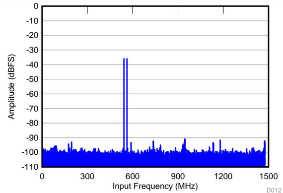
$f_{IN1} = 3.49$  GHz,  $f_{IN2} = 3.51$  GHz, IMD = 92 dBFS,
