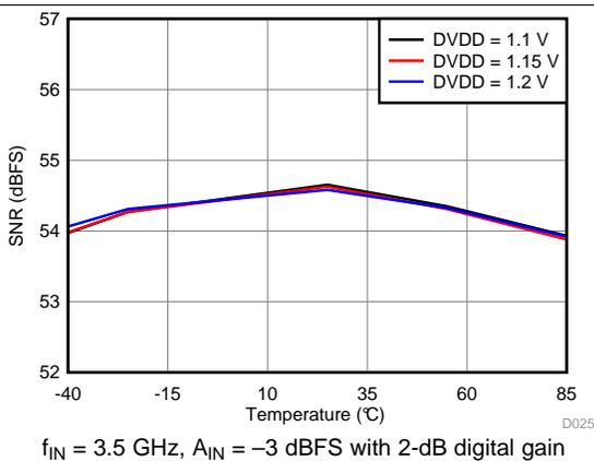
Figure 49. Signal-to-Noise Ratio vs DVDD Supply and Temperature
