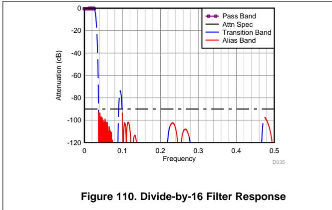
Figure 110. Divide-by-16 Filter Response
