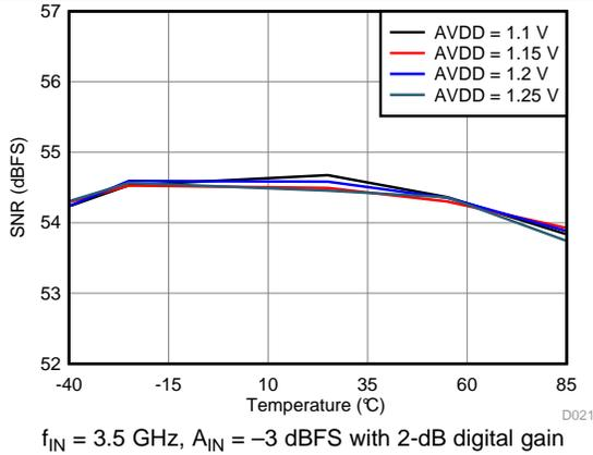
Figure 45. Signal-to-Noise Ratio vs AVDD Supply and Temperature
