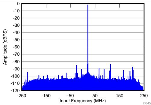
$f_{IN} = 1.78 \text{ GHz}$ ,  $A_{IN} = -2 \text{ dBFS}$ ,  $f_S = 2949.12 \text{ MSPS}$ ,
