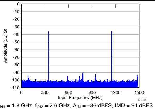
Figure 24. FFT for Two-Tone Input Signal (-36 dBFS)
