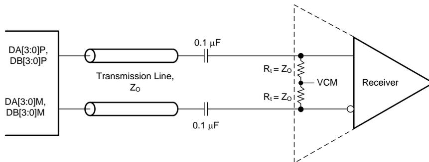
Figure 122. External Serial JESD204B Interface Connection
