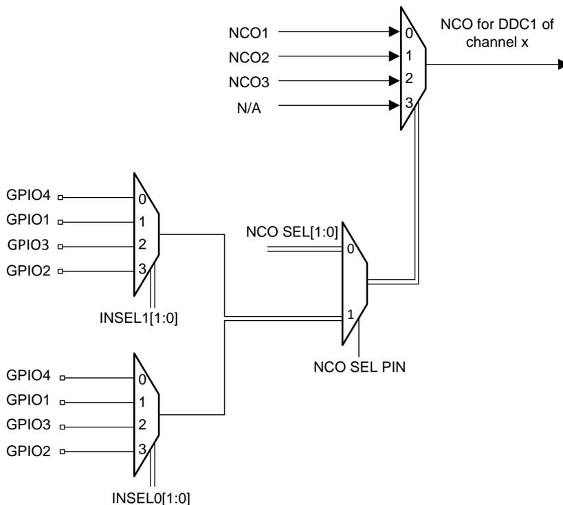
Figure 121. NCO Switching from GPIO and SPI
