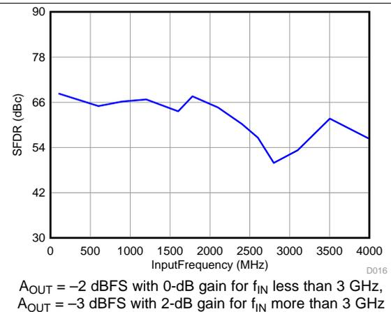
Figure 37. Spurious-Free Dynamic Range vs Input Frequency
