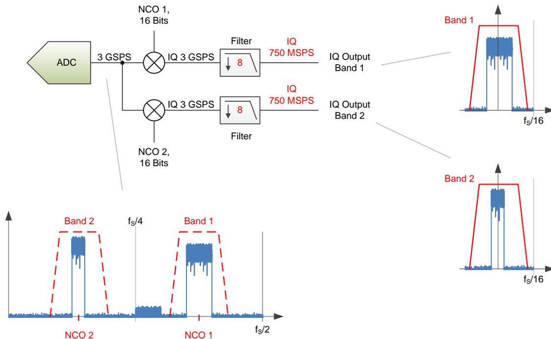
Figure 96. Dual-Band Example
