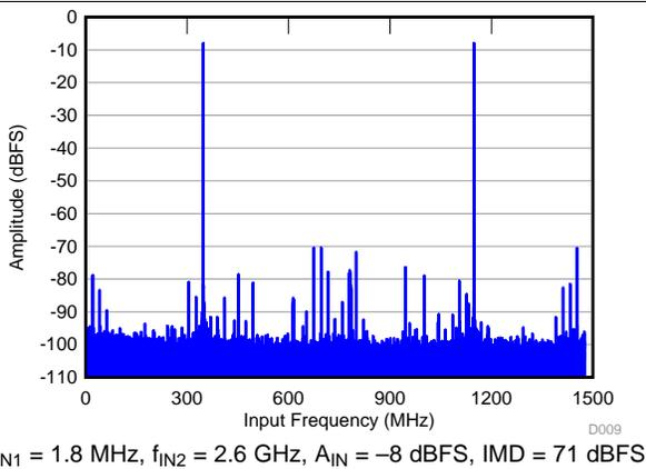
Figure 23. FFT for Two-Tone Input Signal (-8 dBFS)
