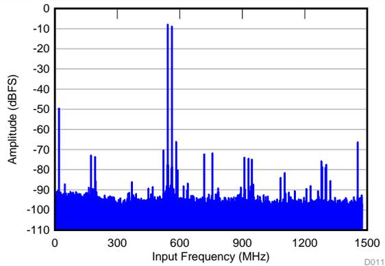
$f_{IN1} = 3.49$  MHz,  $f_{IN2} = 3.51$  GHz, IMD = 66 dBFS,
