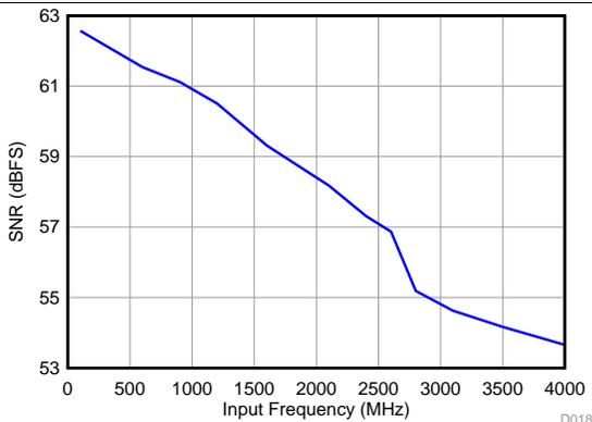
A<sub>OUT</sub> = -2 dBFS with 0-dB gain for f<sub>IN</sub> less than 3 GHz,
