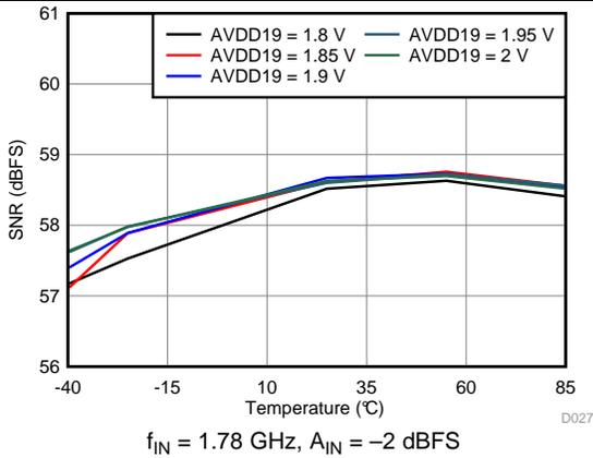
Figure 51. Signal-to-Noise Ratio vs AVDD19 Supply and Temperature
