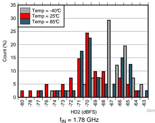
Figure 55. HD2 Histogram at AVDD19 = 1.8 V
