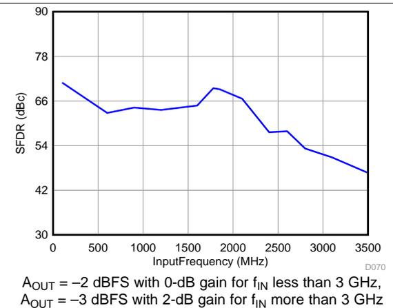
Figure 38. Spurious-Free Dynamic Range vs Input Frequency ( $f_s = 2457.6 \text{ MSPS}$ )
