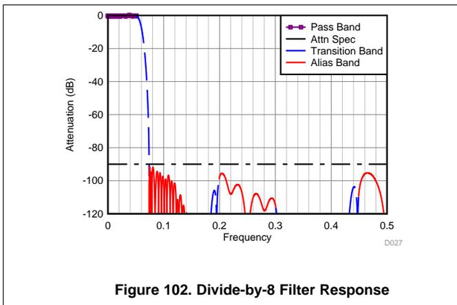
Figure 102. Divide-by-8 Filter Response
