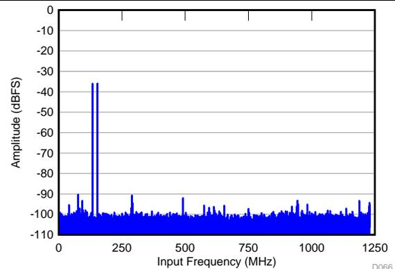
$f_{IN1} = 2.59$  GHz,  $f_{IN2} = 2.6$  GHz,  $A_{IN} = -36$  dBFS,
