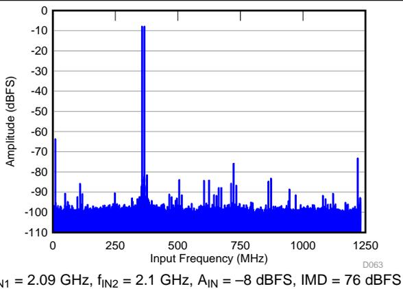
Figure 25. FFT for Two-Tone Input Signal (-8 dBFS,  $f_s = 2457.6 \text{ MSPS}$ )
