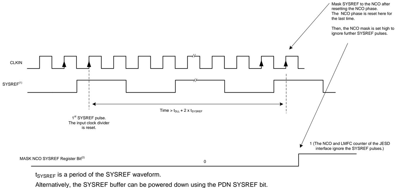
**Figure 92. SYSREF Used as a Periodic Waveform**
