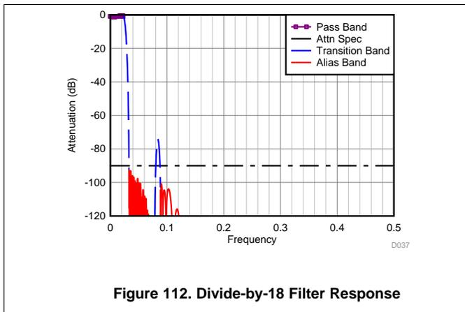
Figure 112. Divide-by-18 Filter Response
