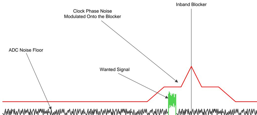
**Figure 256. Small Wanted Signal in Presence of Interferer**
