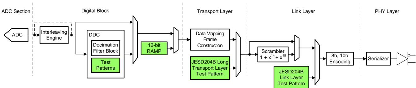
Figure 131. Test Pattern Generator Implementation
