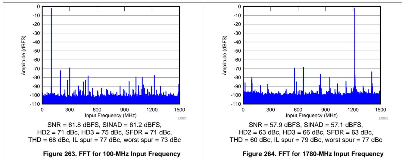
Figure 263. FFT for 100-MHz Input Frequency
