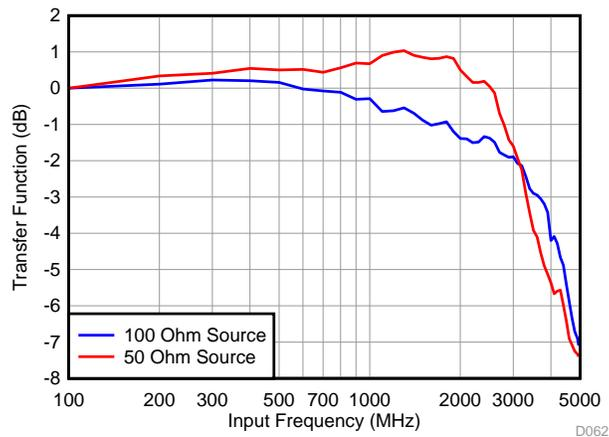
Figure 84. Input Bandwidth with a 100- $\Omega$  Source Resistance
