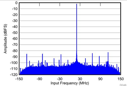
$f_{IN} = 1.78 \text{ GHz}$ ,  $A_{IN} = -2 \text{ dBFS}$ ,  $f_S = 2949.12 \text{ MSPS}$ ,
