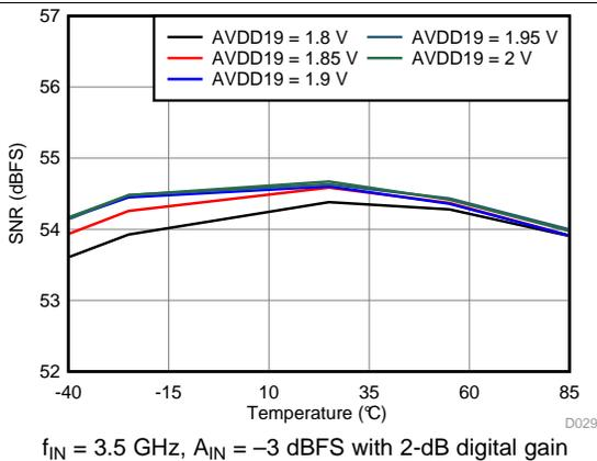
Figure 53. Signal-to-Noise Ratio vs AVDD19 Supply and Temperature
