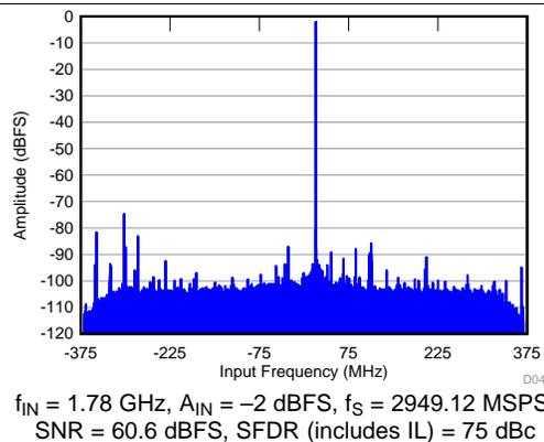
Figure 68. FFT in 4X Decimation (Complex Output)
