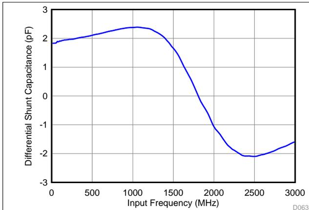
Figure 82. Differential Input Capacitance vs Input Frequency
