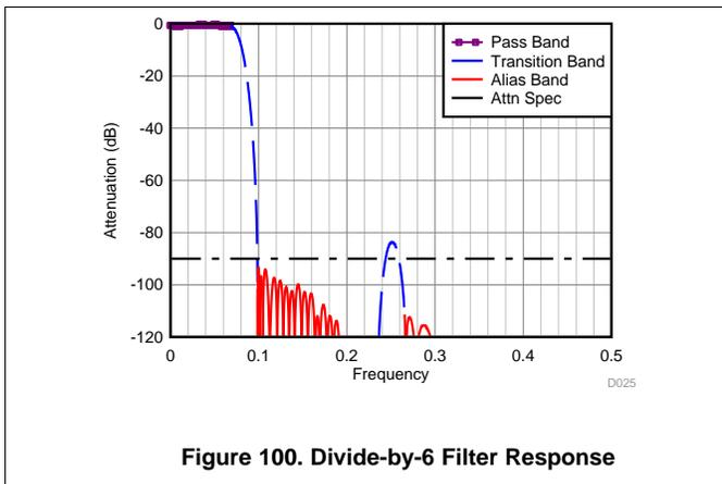
Figure 100. Divide-by-6 Filter Response
