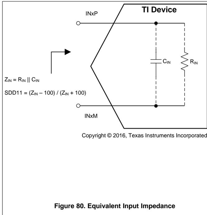
**Figure 80. Equivalent Input Impedance**
