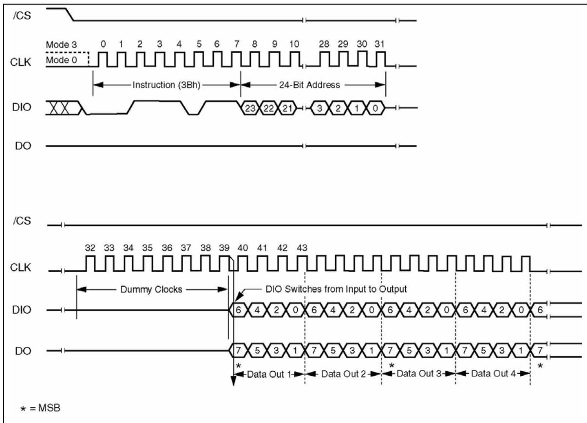
Figure 10. Fast Read Dual Output Instruction Sequence Diagram
