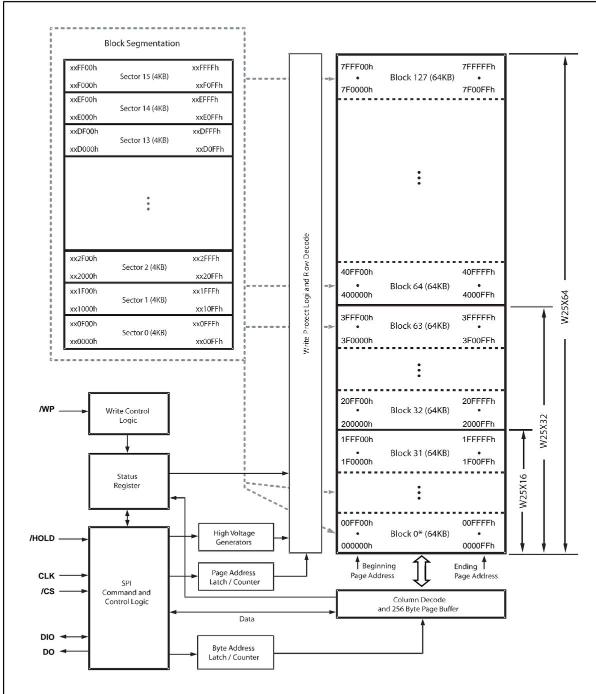
Figure 2. W25X16/16A, W25X32 and W25X64 Block Diagram
