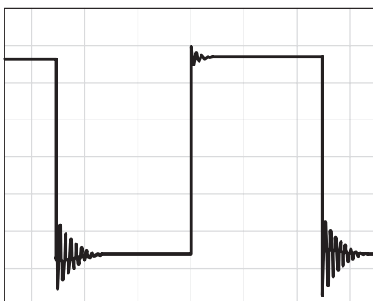
(b) C_L = 130 \text{ pF} , R_L = \text{NO LOAD}
