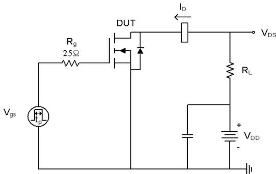
Fig17-1. Switching time test circuit for resistive load
