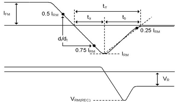
Fig16-2. Diode reverse recovery test waveform
