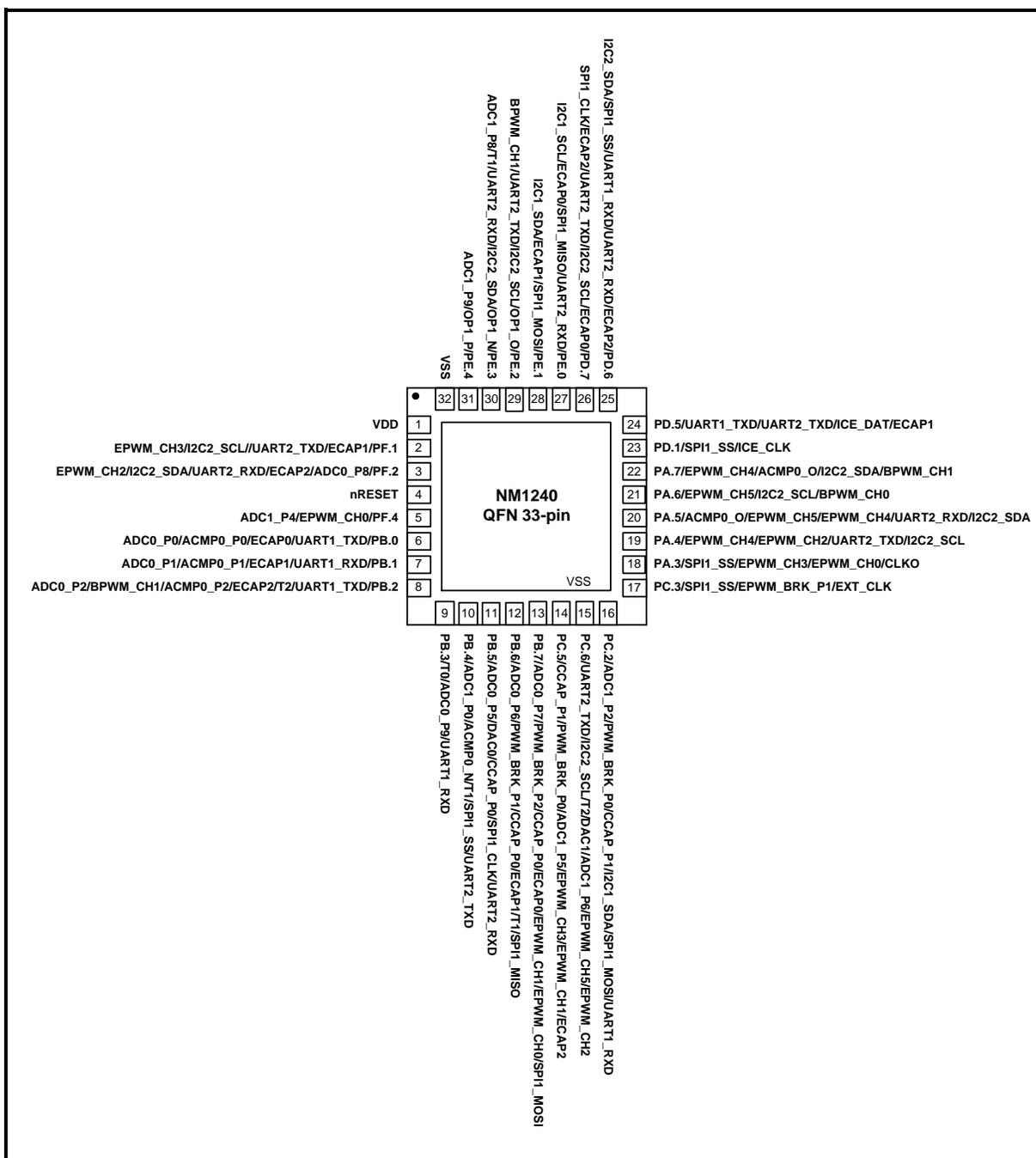
Figure 4.2-3 NuMicro® NM1240 Base Series QFN 33-pin Diagram
