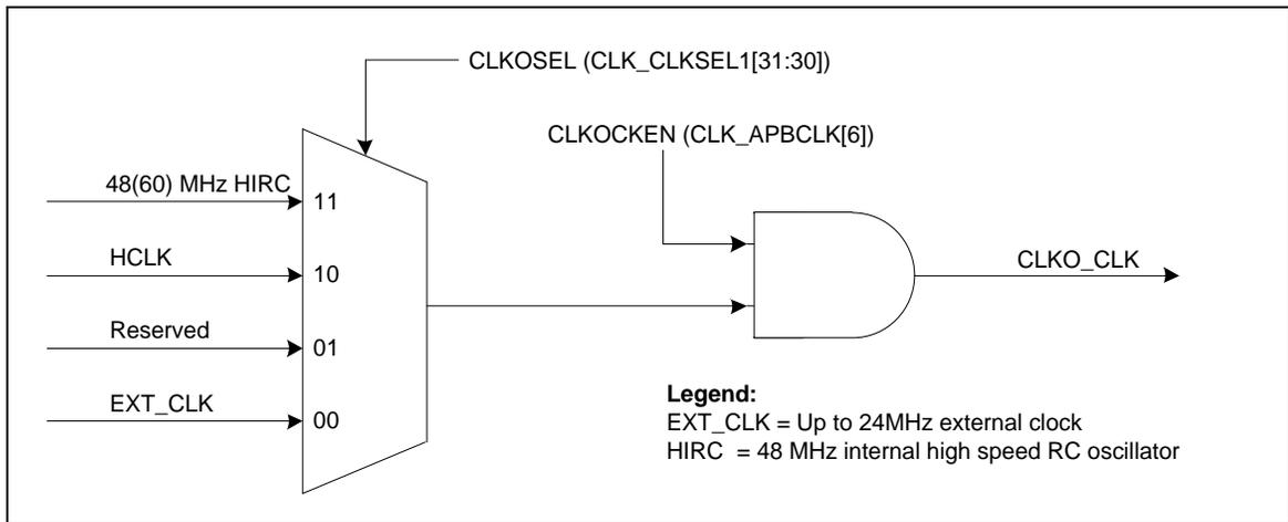
Figure 6.3-6 Clock Source of Frequency Divider
