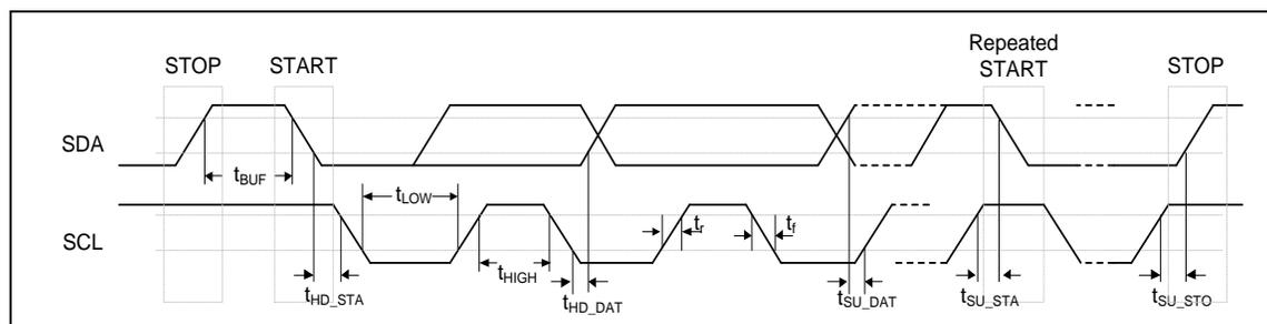
Figure 6.15-1 I<sup>2</sup>C Bus Timing
