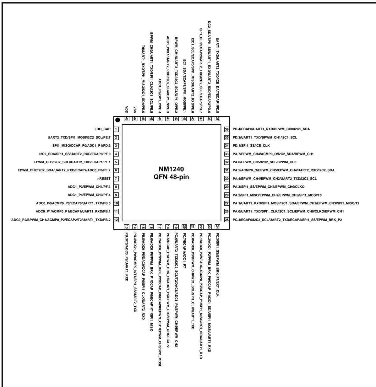
Figure 4.2-2 NuMicro® NM1240 Base Series QFN 48-pin Diagram
