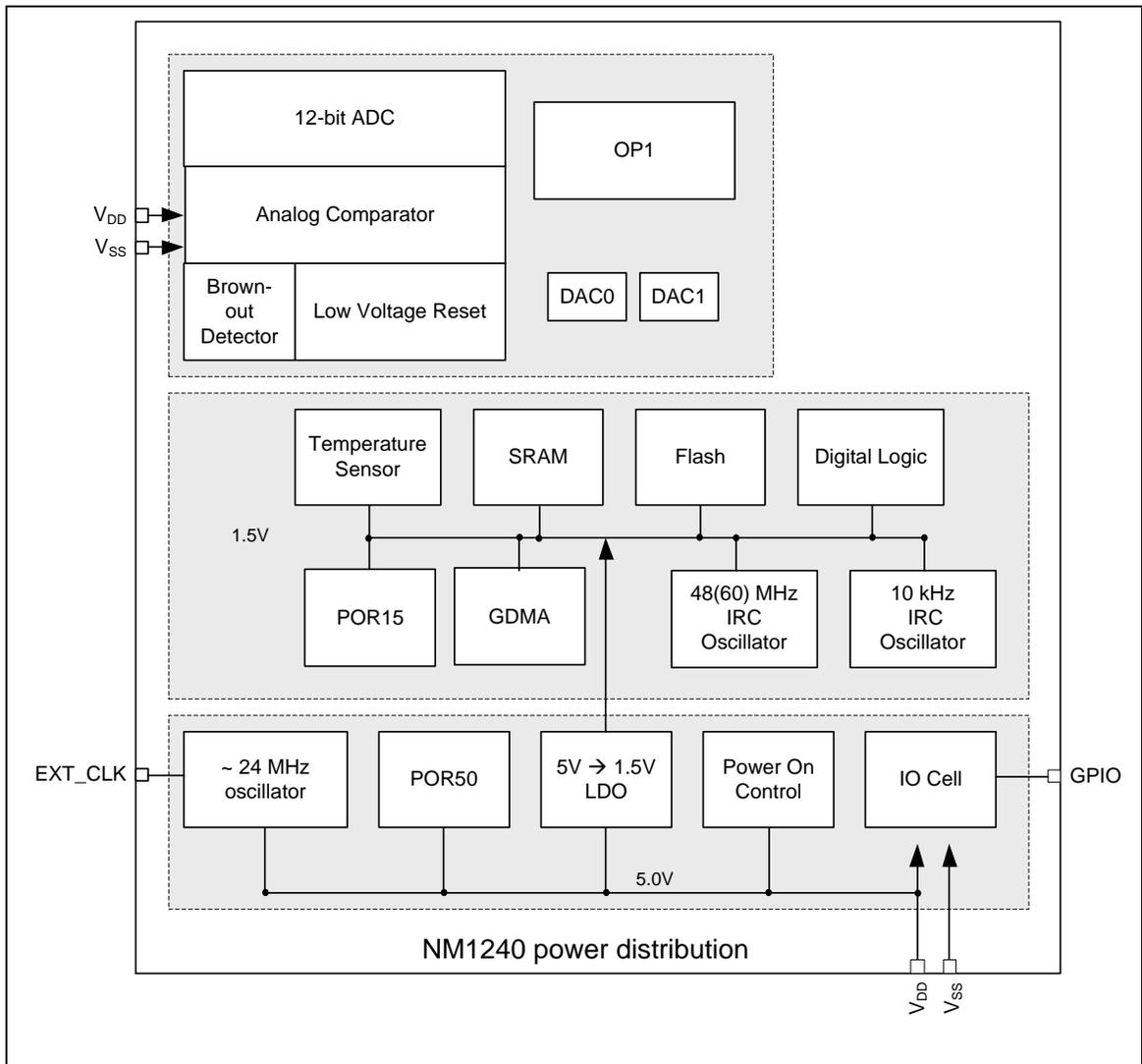
Figure 6.2-7 NuMicro® NM1240 Series Power Architecture Diagram
