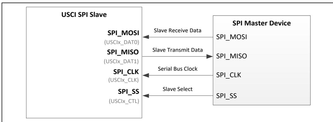
Figure 6.14-2 SPI Slave Mode Application Block Diagram (x=1)
