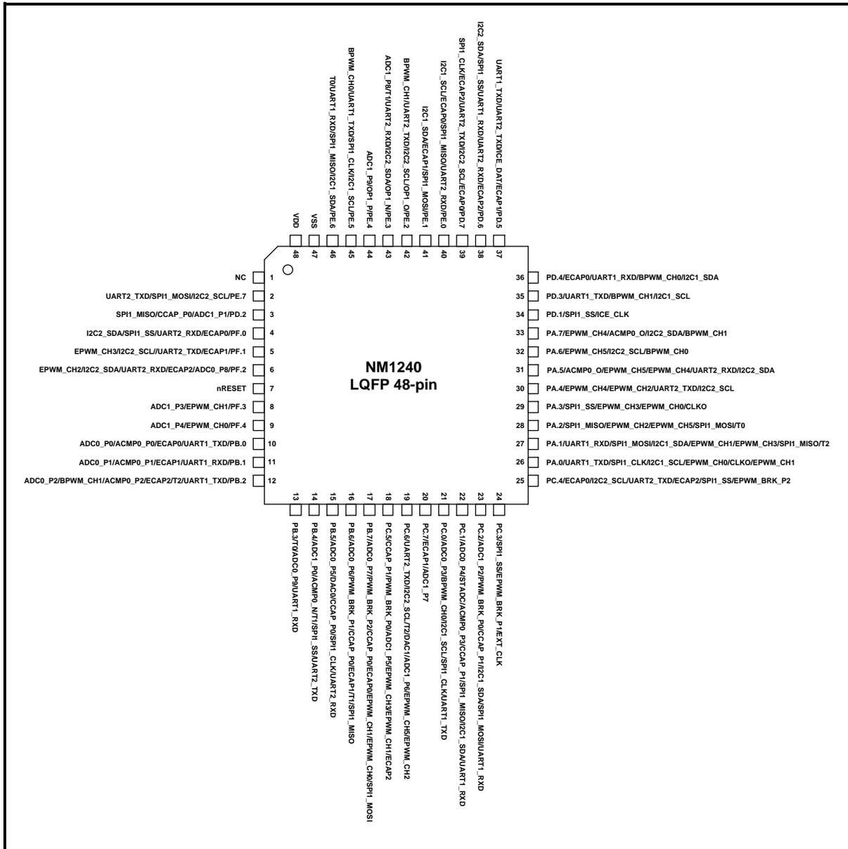
Figure 4.2-1 NuMicro® NM1240 Base Series LQFP 48-pin Diagram
