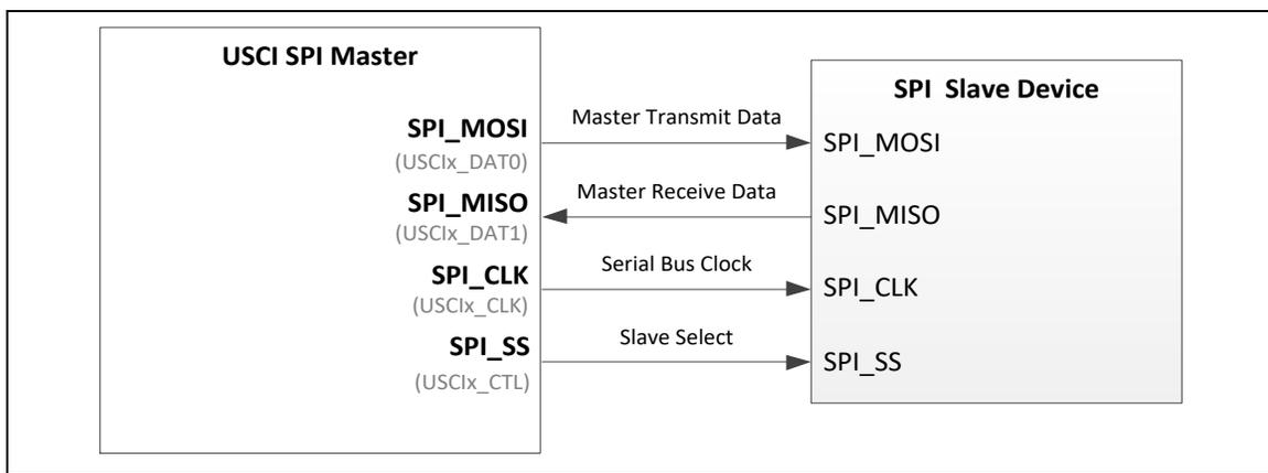
Figure 6.14-1 SPI Master Mode Application Block Diagram (x=1)
