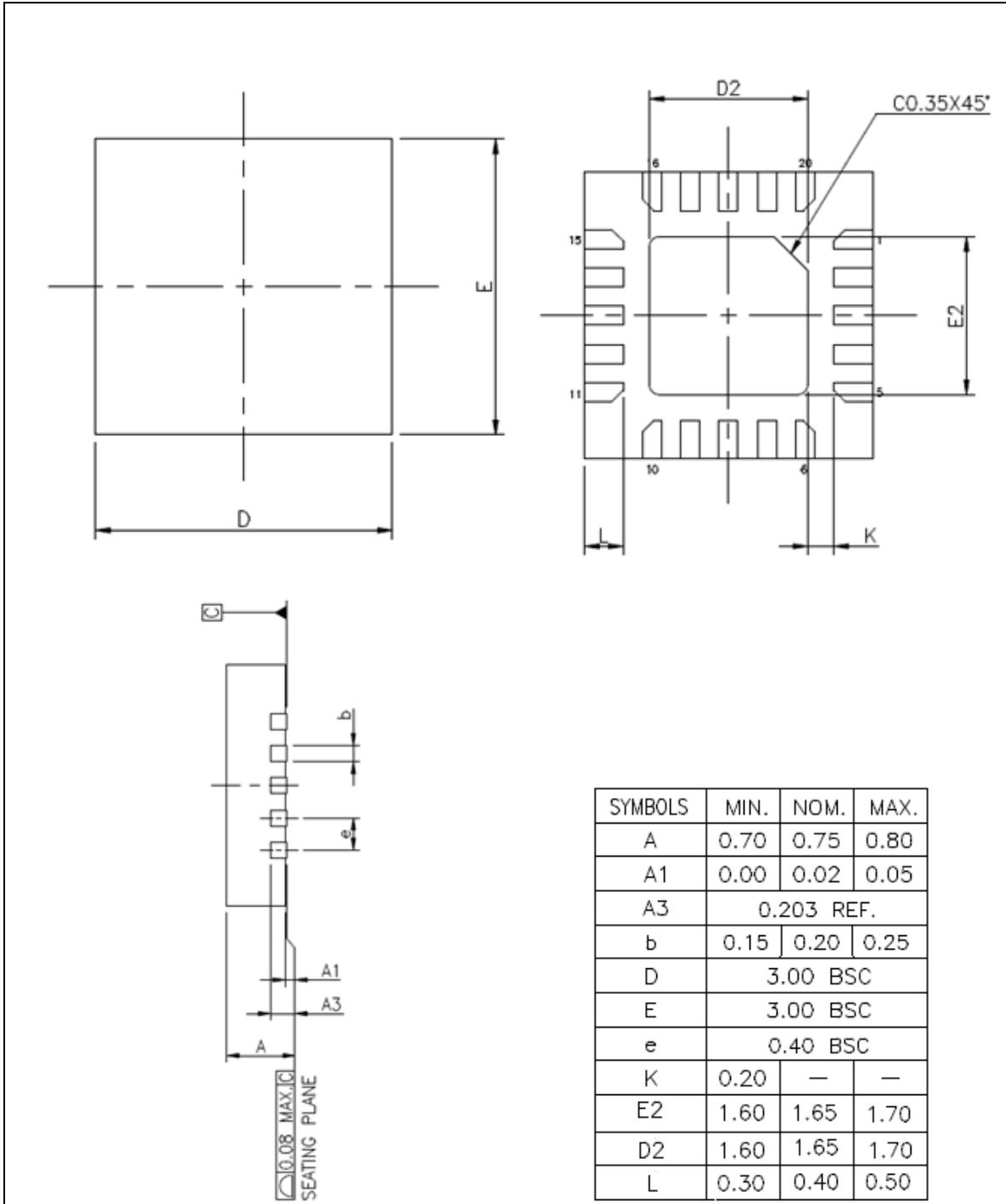
Figure 9.2-1 QFN-20 Package Dimension for MS51XB9AE
