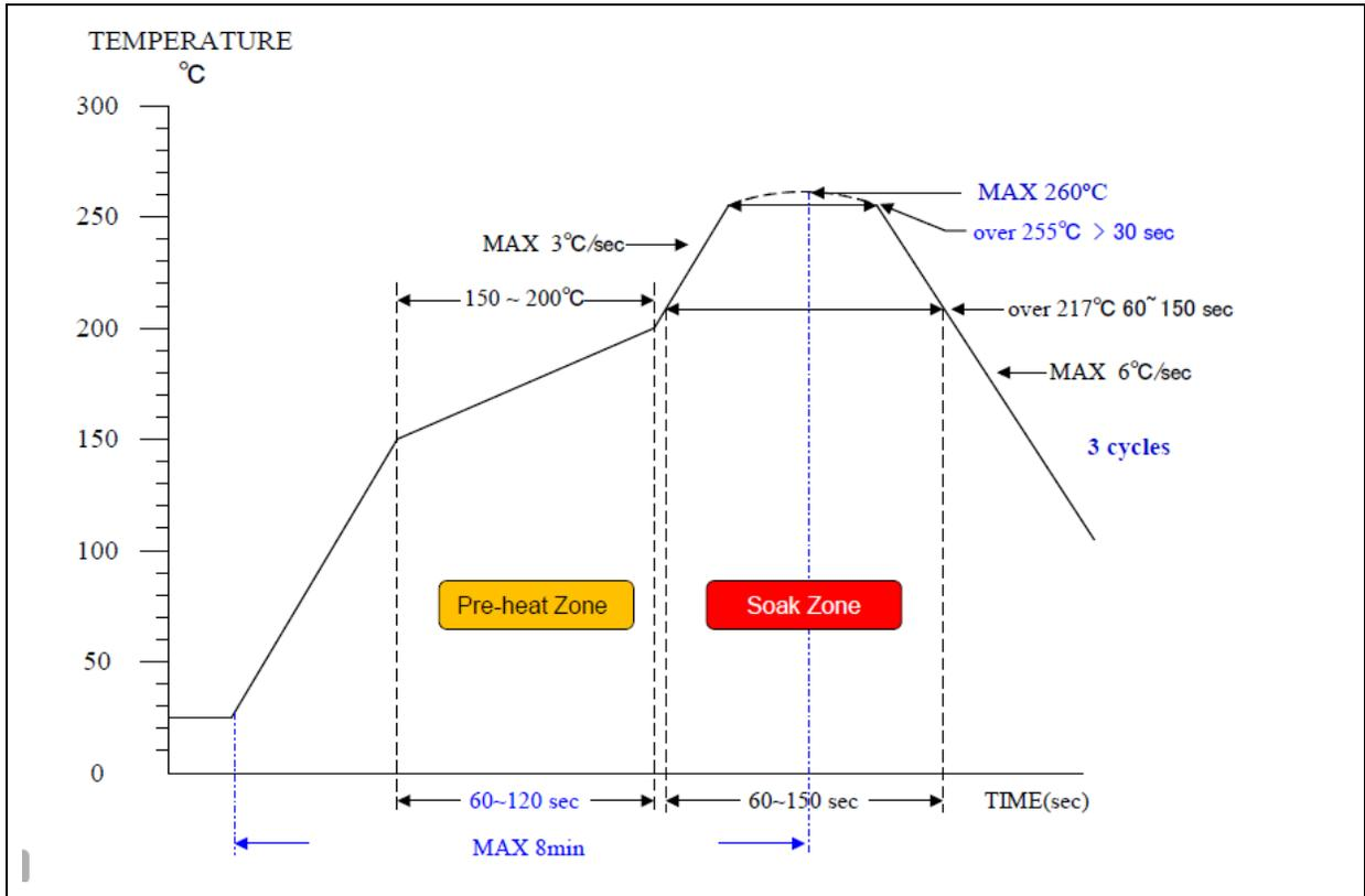
Figure 8.7-1 Soldering profile from J-STD-020C
