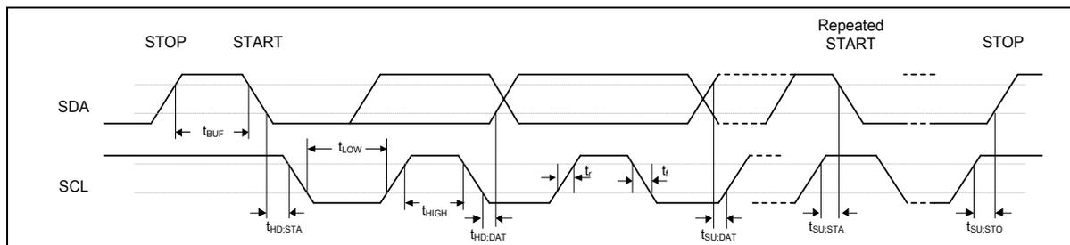
Figure 8.5-2 I<sup>2</sup>C Timing Diagram
