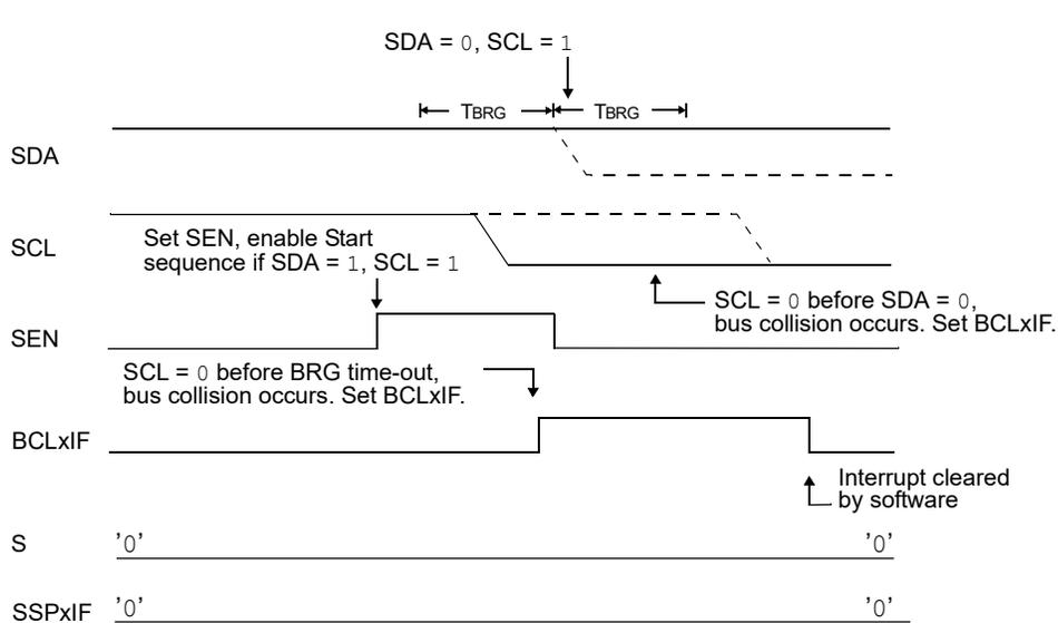
If the SDA pin is sampled low during this count, the BRG is reset and the SDA line is asserted early (see [Figure 29-36](#)). If, however, a '1' is sampled on the SDA pin, the SDA pin is asserted low at the end of the BRG count. The
