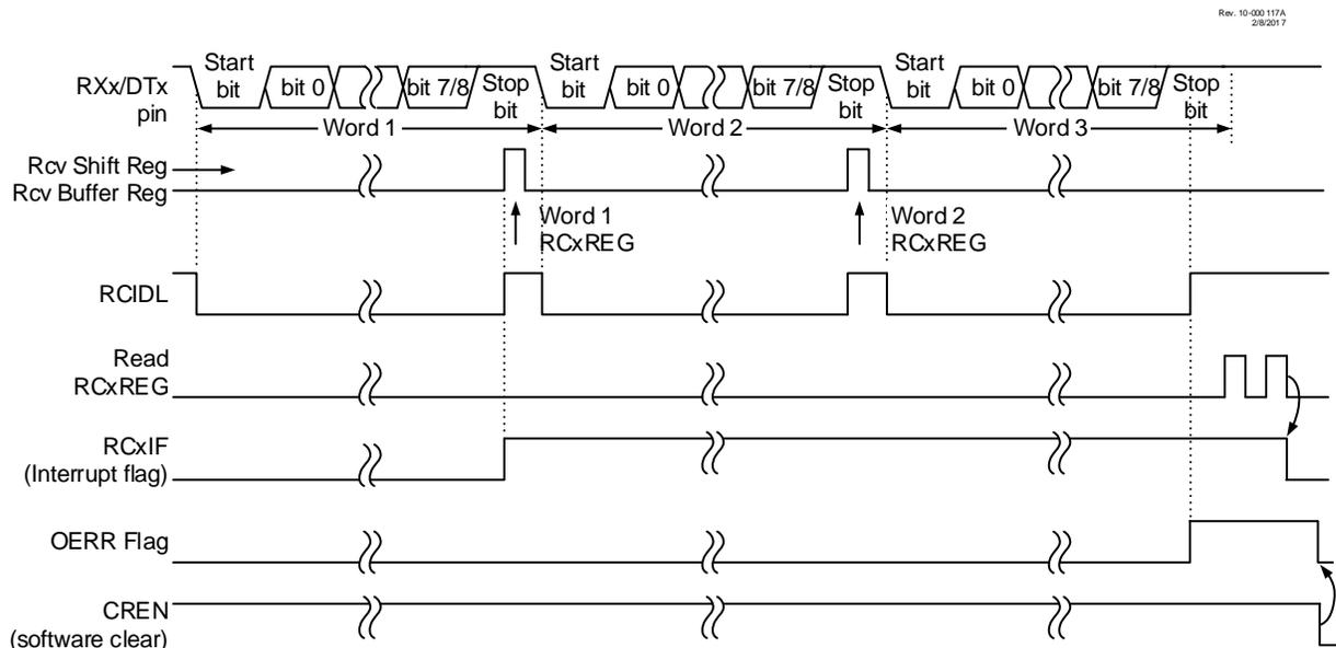
**Note:** This timing diagram shows three bytes appearing on the RXx input. The OERR flag is set because the RCxREG register is not read before the third word is received.
