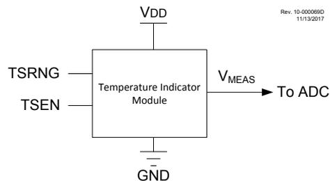
The output of the circuit is measured using the internal Analog-to-Digital Converter. A channel is reserved for the temperature circuit output. Refer to the “**ADCC - Analog-to-Digital Converter with Computation Module**” chapter for more details.
