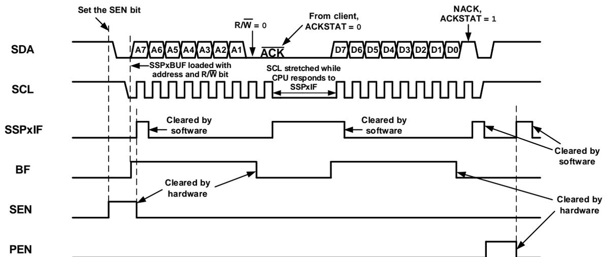
**Figure 29-30. I<sup>2</sup>C Host Mode Waveform (Transmission, 10-Bit Address)**
