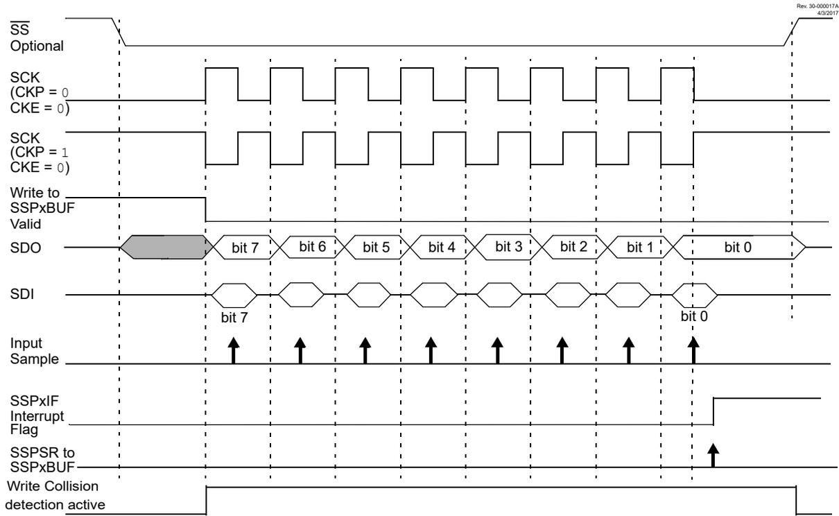
**Figure 29-8. SPI Mode Waveform (Client Mode with CKE = 1)**
