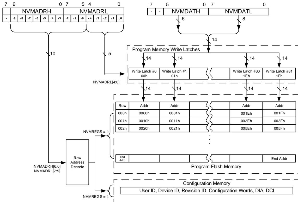
Figure 15-5. Program Flash Memory Write Sequence
