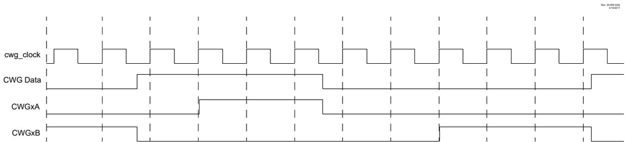
Dead band is always initiated on the edge of the input source signal. A count of zero indicates that no dead band is present.
