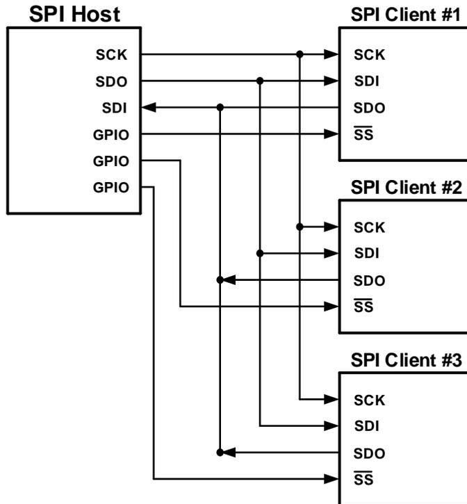
Transmissions involve two shift registers, eight bits in size: One in the host and one in the client. Data is always shifted out one bit at a time, with the Most Significant bit (MSb) shifted out first. At the same time, a new Least Significant bit (LSb) is shifted into the same register.
