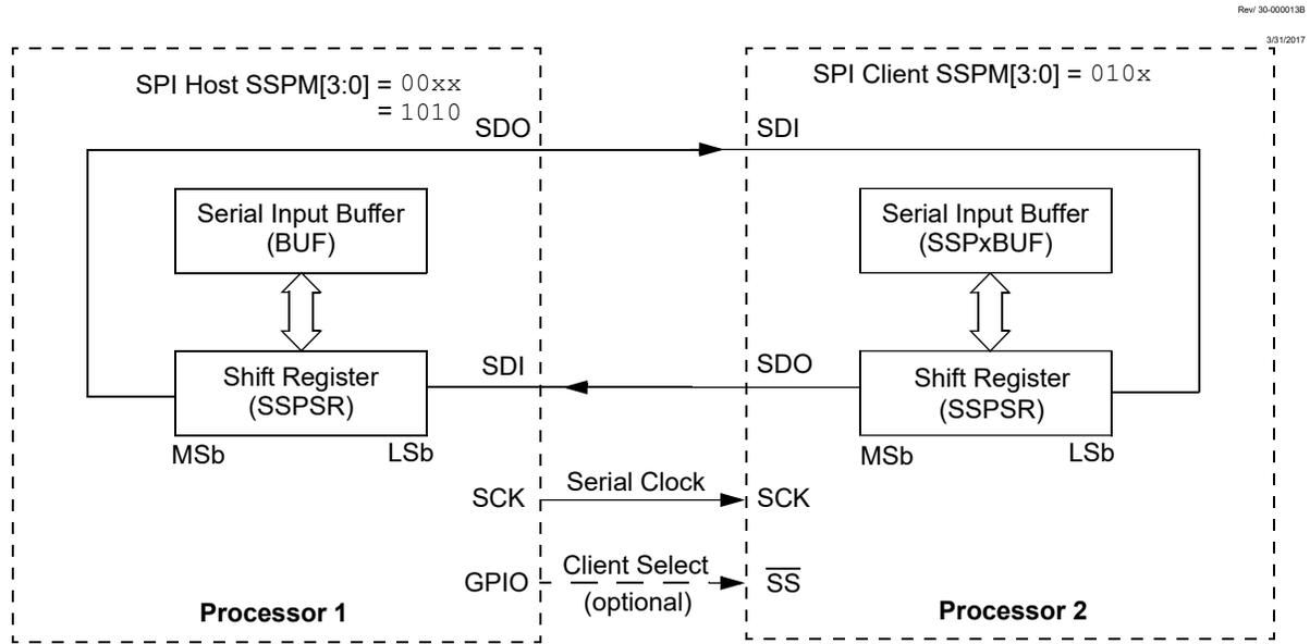
Data is shifted out of both shift registers on the programmed clock edge and latched on the opposite edge of the clock.
