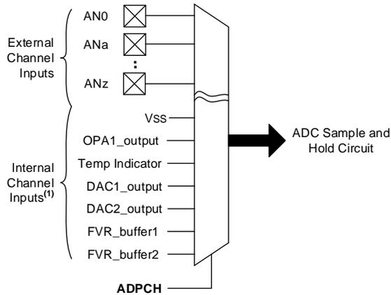
**Note 1:** The internal input channel selections vary. The inputs shown are all possible input selections. Refer to the “**ADC Positive Input Channel Selection**” table for device-specific selection options.
