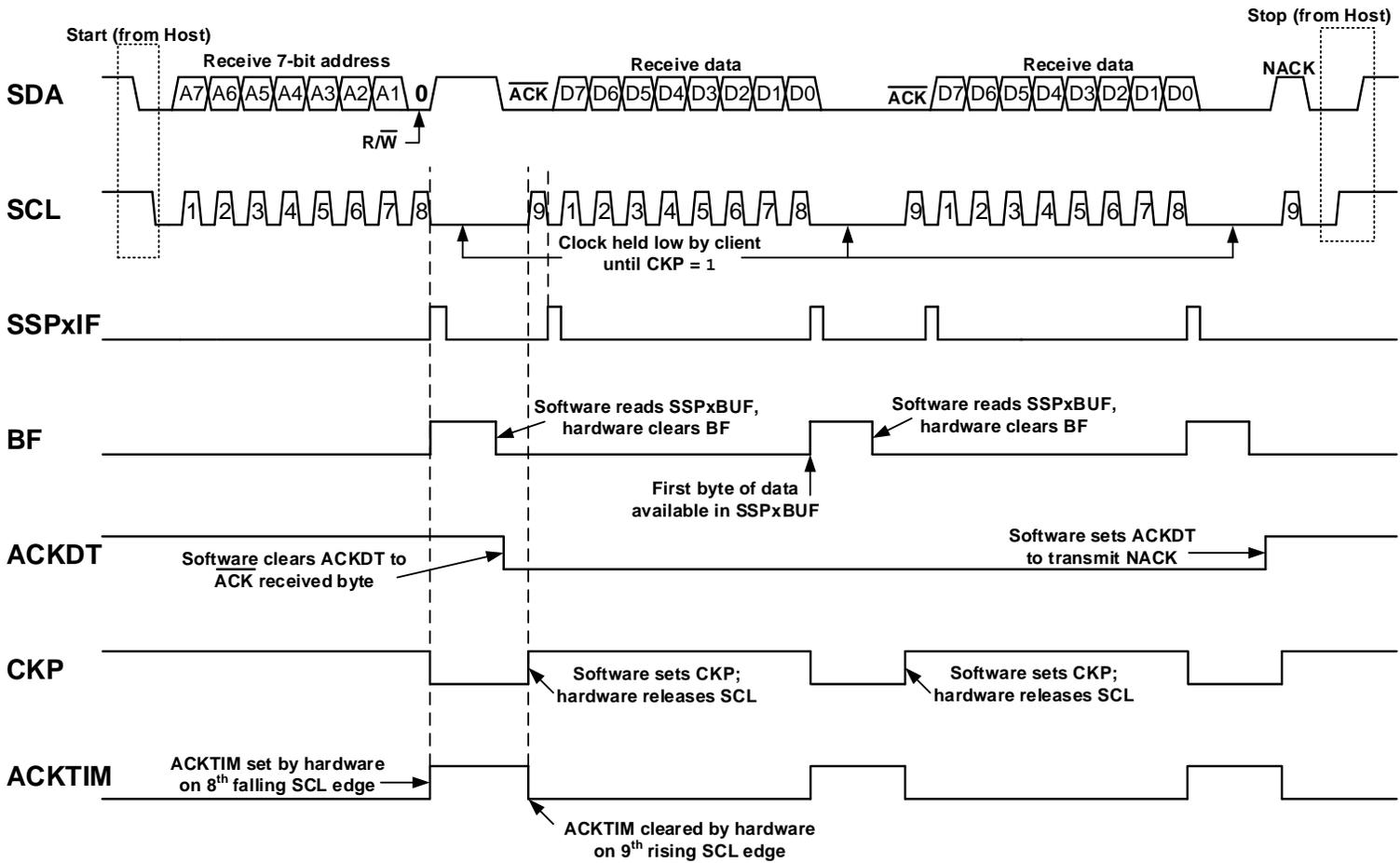
Figure 29-18. I<sup>2</sup>C Client, 7-Bit Address, Reception (SEN = 1, AHEN = 1, DHEN = 1)
