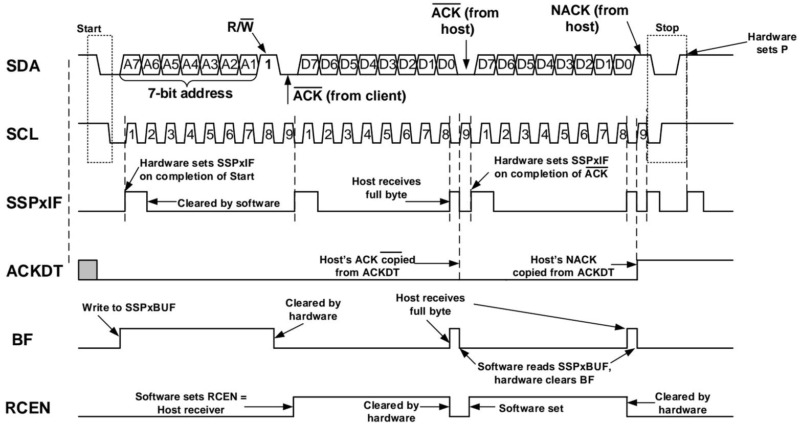
Figure 29-32. I<sup>2</sup>C Host Mode Waveform (Reception, 10-Bit Address)
