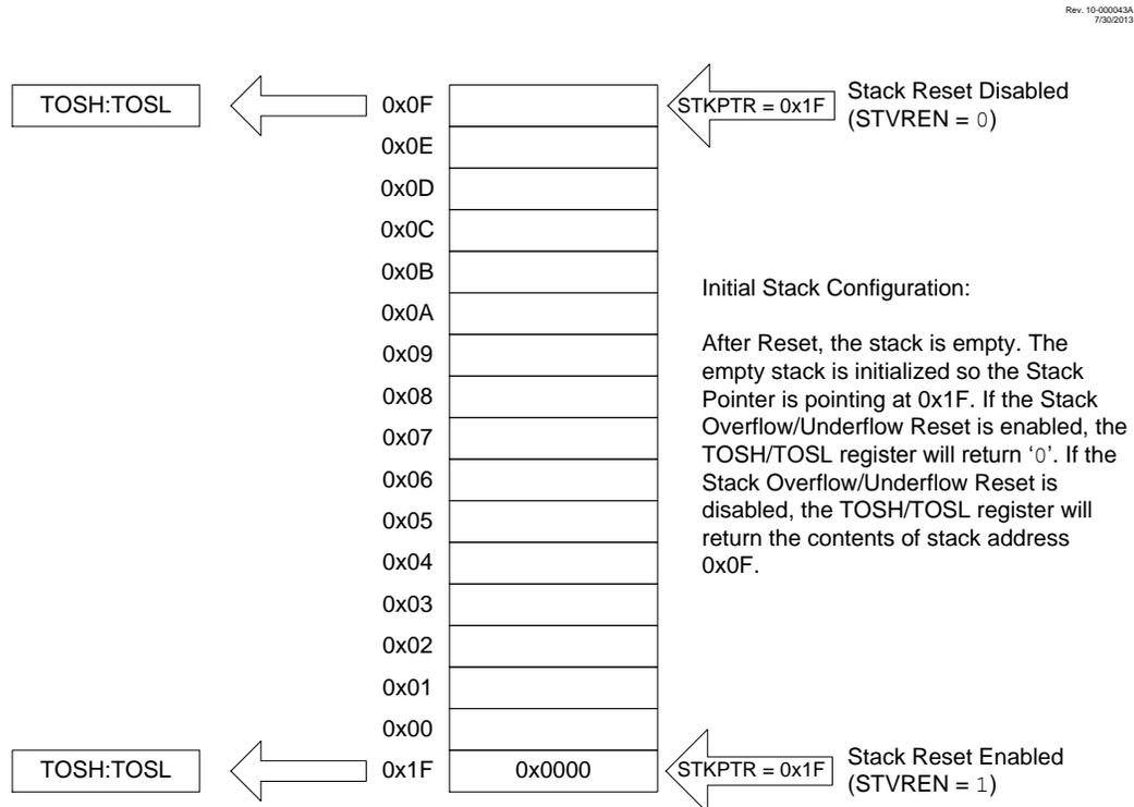
Figure 9-15. Accessing the Stack Example 2
