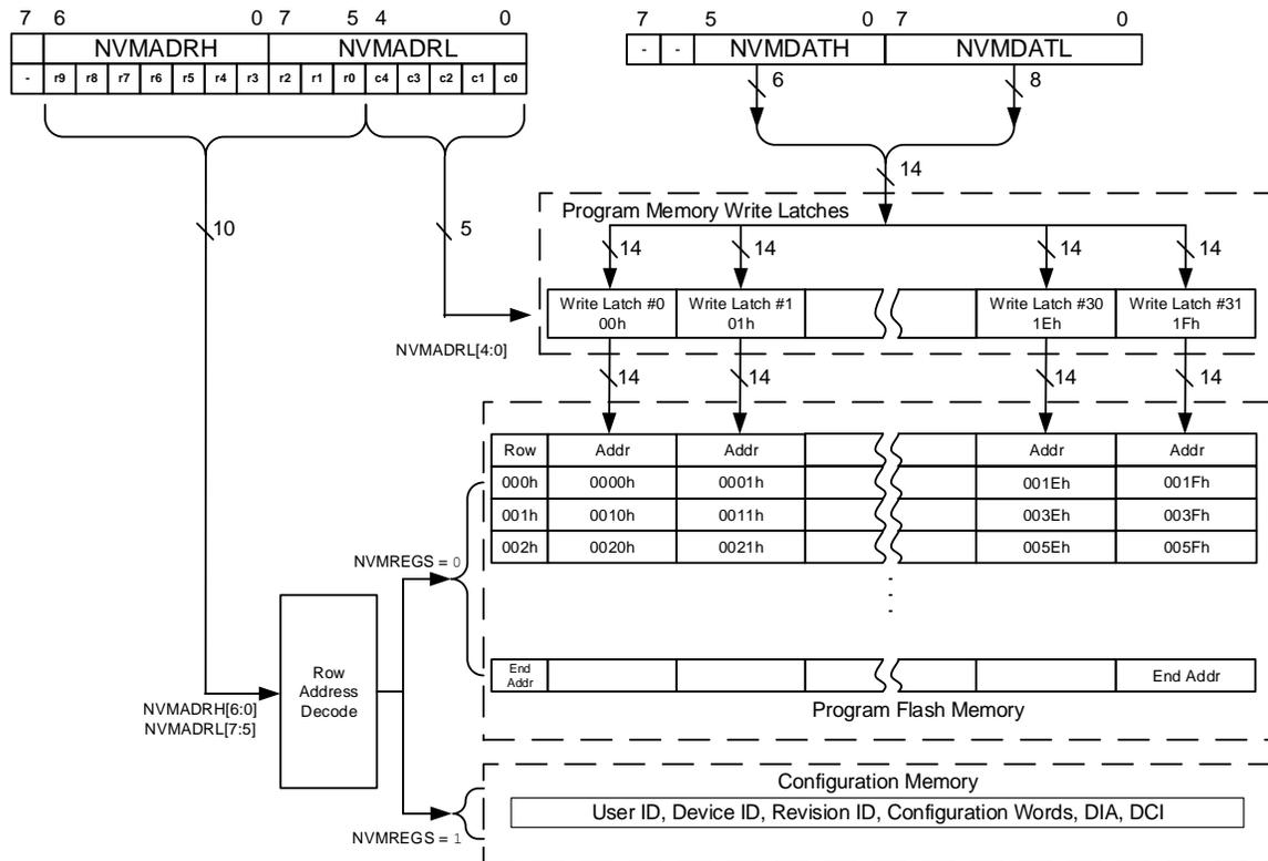
Figure 15-5. Program Flash Memory Write Sequence
