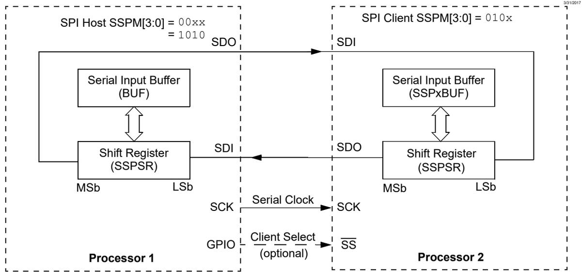
Data is shifted out of both shift registers on the programmed clock edge and latched on the opposite edge of the clock.
