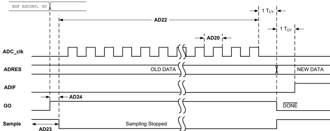
Figure 41-11. ADC Conversion Timing (ADC Clock from ADCRC)
