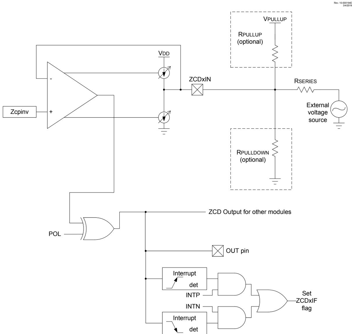
The ZCD module is useful when monitoring an A/C waveform for, but not limited to, the following purposes:
