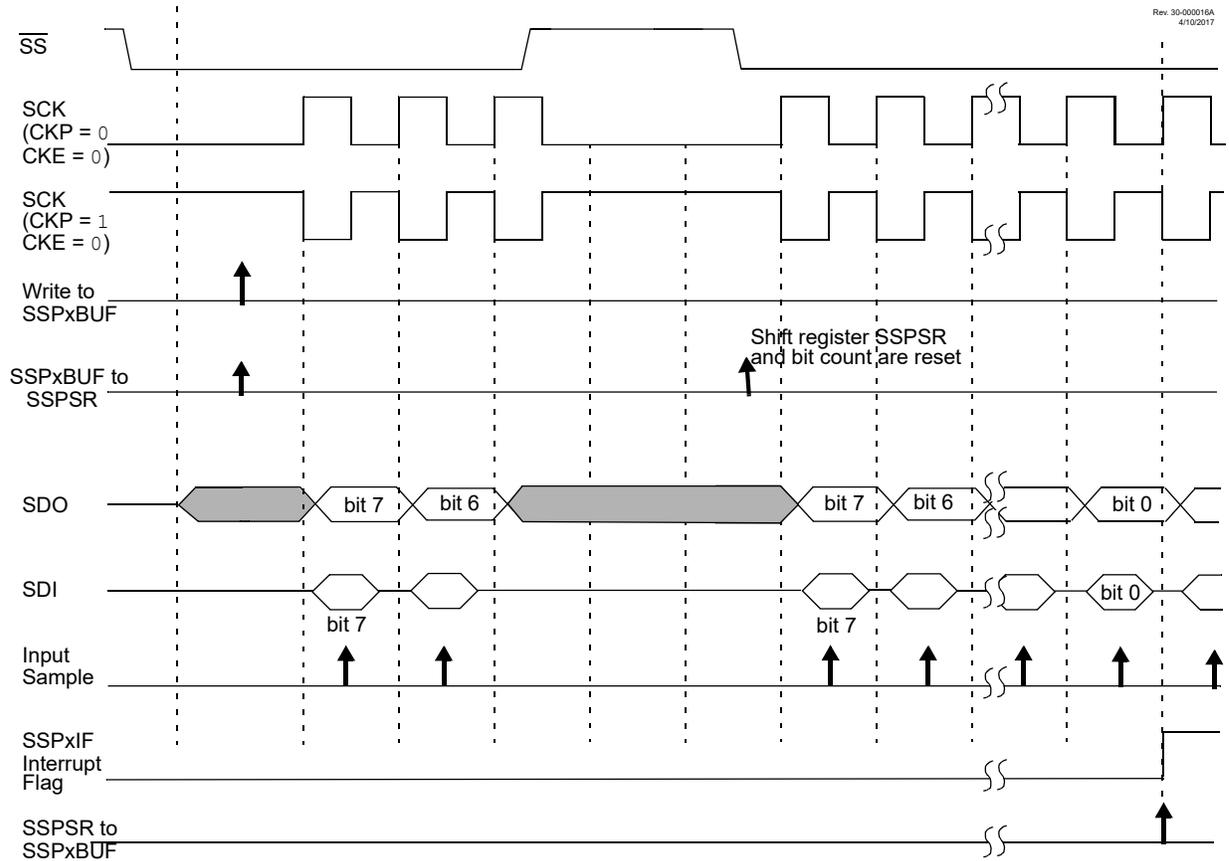
Figure 29-7. SPI Mode Waveform (Client Mode with CKE = 0)
