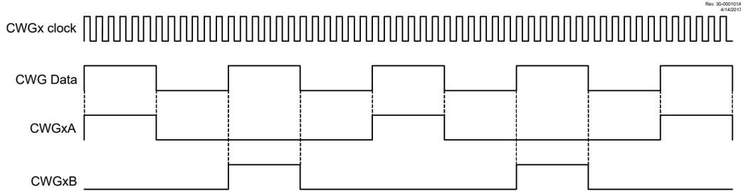
**23.2.4.2 Asynchronous Steering Mode**
