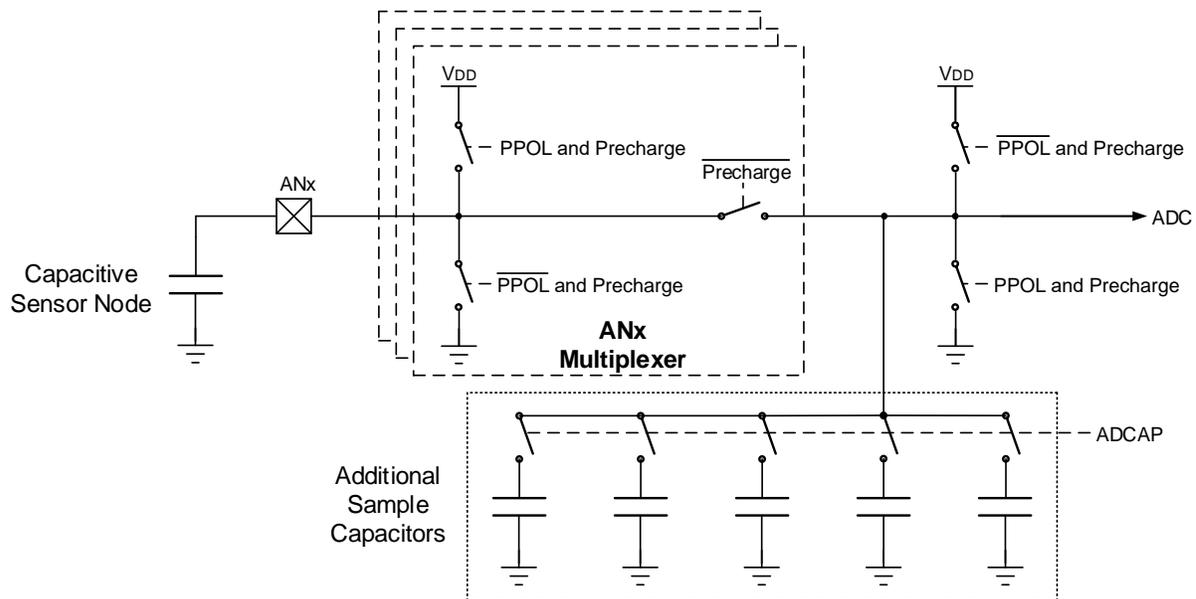
This is an example to configure ADC for CVD operation:
