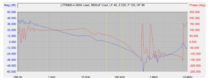
Figure 3. Measured Bode Plot of the LTP8800-4A
