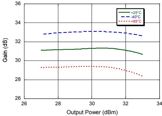
**Gain vs. Pout over Frequency Band**
