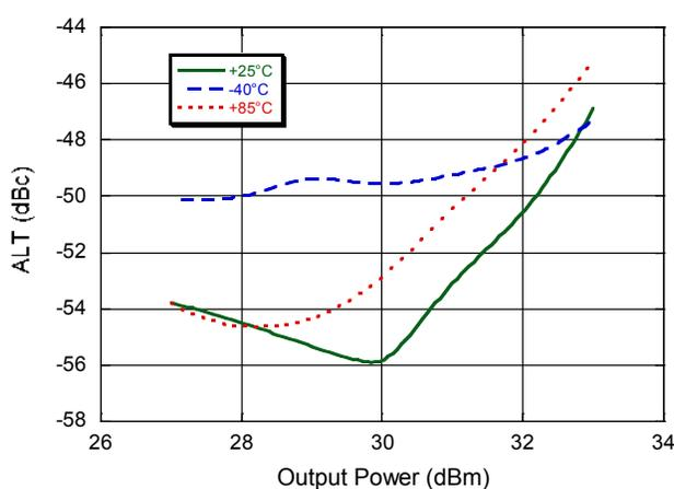
**Alternate Channel Power vs. Pout over Frequency Band**
