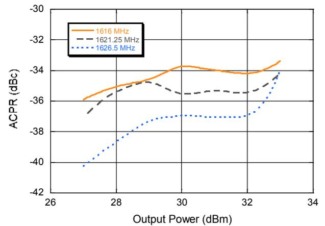
**Alternate Channel Power vs. Pout over Temperature**
