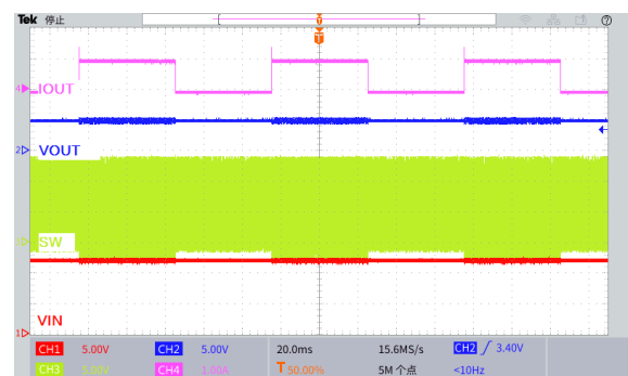
Figure 27. Load Transient Response ( V_{IN}=12V , V_{OUT}=5.0V , I_{OUT}=0 to 1A)
