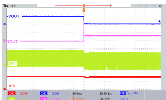
Figure 22. Output Short Circuit Waveform ( V_{IN}=8V , V_{OUT}=5.0V )
