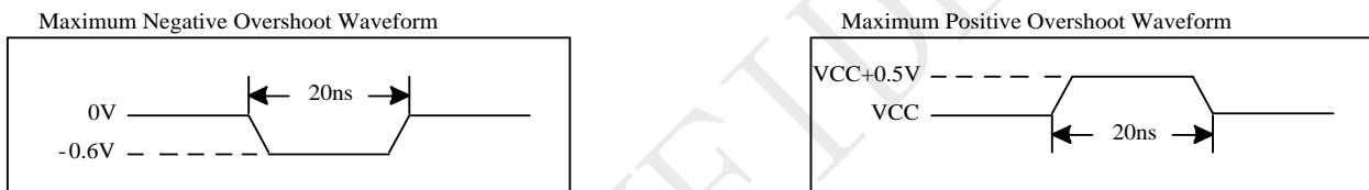
Figure 5-1 Maximum Overshoot Waveform
