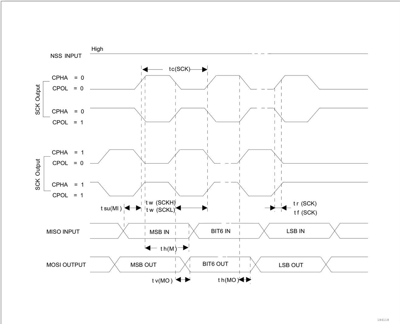
Figure 17. SPI timing diagram-master mode<sup>(1)</sup>
