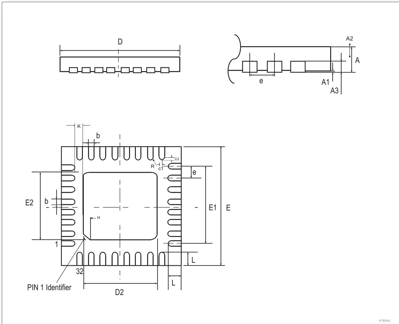
Figure 23. QFN32 - 32-pin quad flat no-leads package outline
