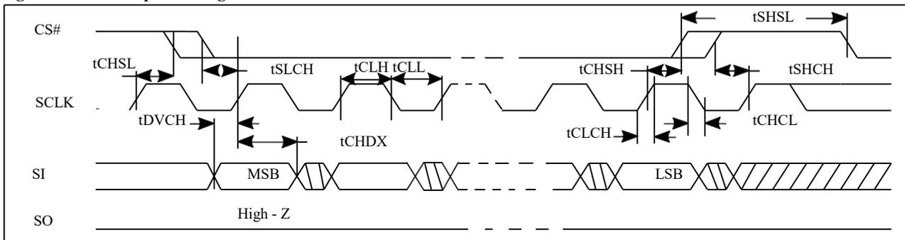
Figure 4-5 Output Timing
