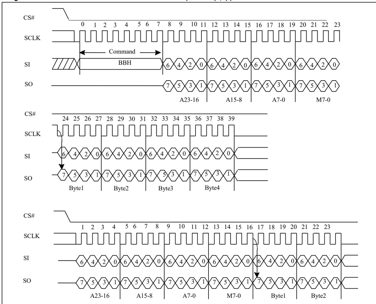
Note: 2 X IO Read Performance Enhance Mode, if M5-4 = 1, 0. If not using performance enhance recommend to set M5-4 ≠ 1, 0.
