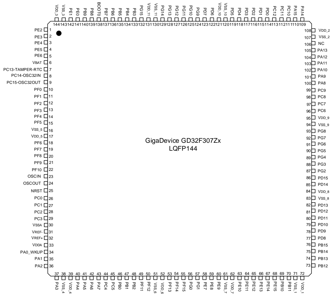
Figure 2-2 GD32F307Zx LQFP144 pinouts
