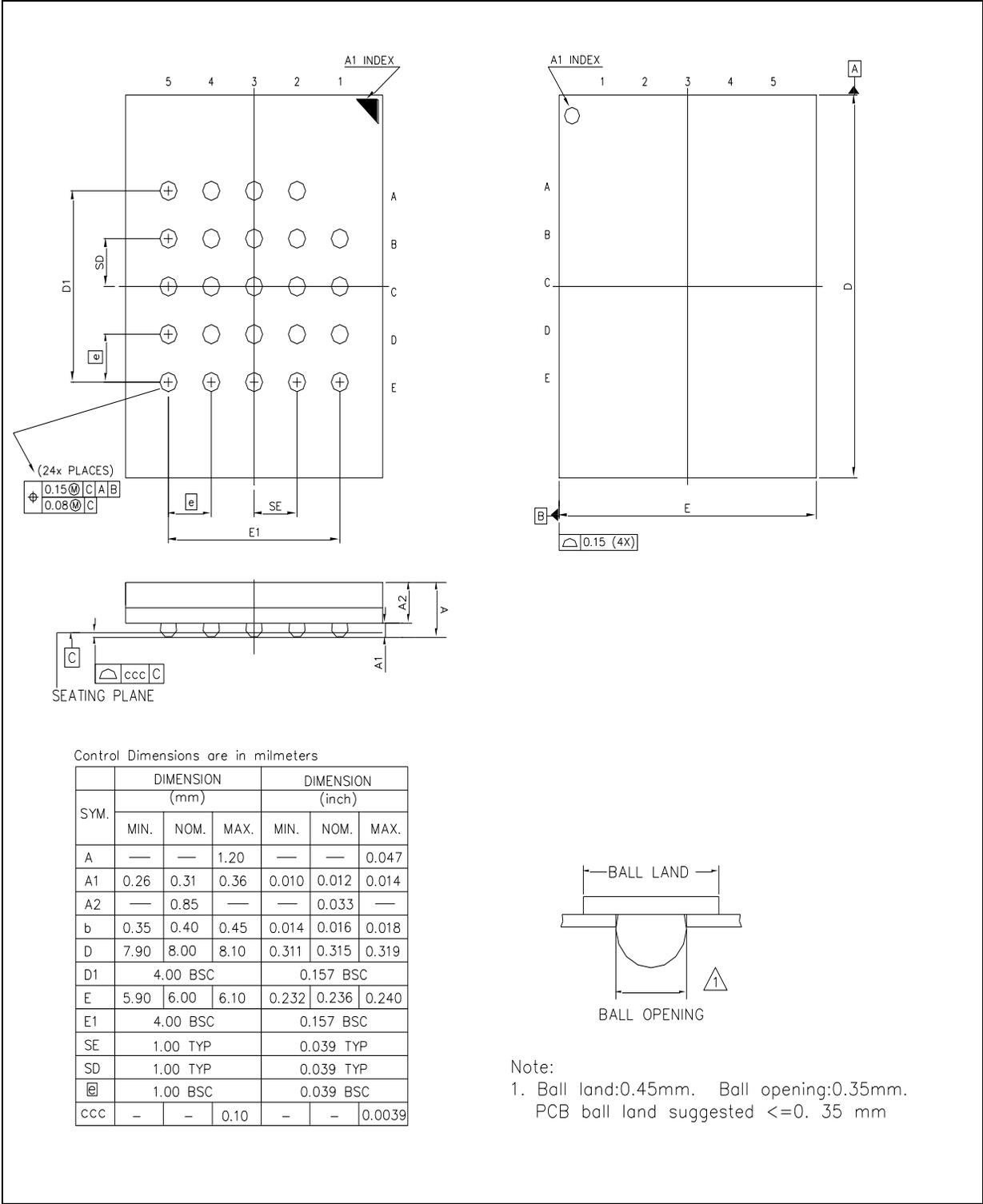
Control Dimensions are in millimeters
