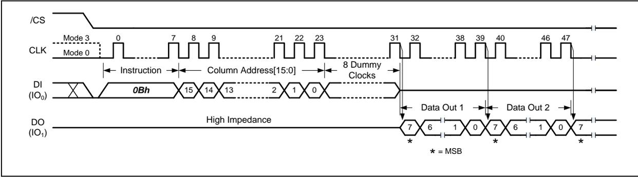
Figure 17. Fast Read Instruction (Buffer Read Mode, BUF=1)
