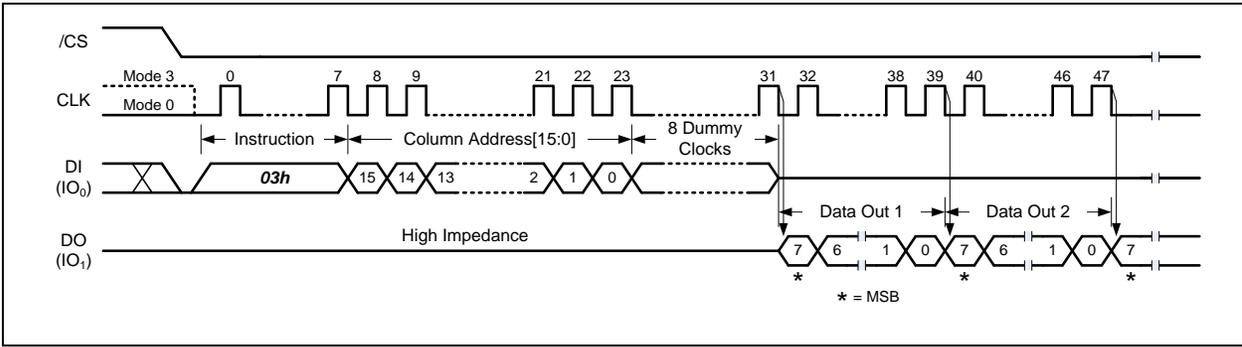
Figure 16. Read Data Instruction (Buffer Read Mode, BUF=1)
