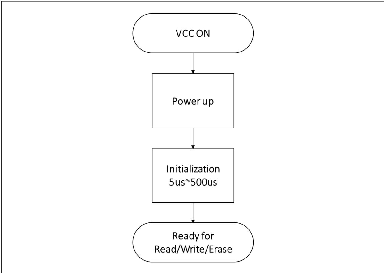
Figure 3a. W25N01KV Flash Memory Operation Diagram
