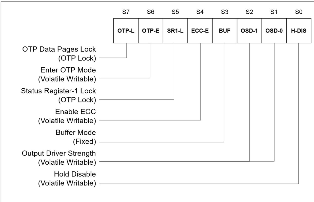
Figure 4b. Configuration Register / Status Register-2 (Address Bxh)
