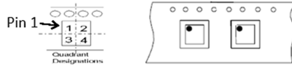
Figure 12.5 Quadrant Designation for Pin1 Orientation in Tape
