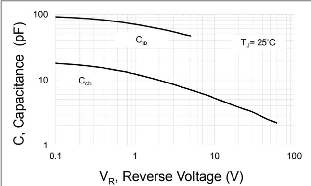
**Fig.5 Typical Capacitance**
