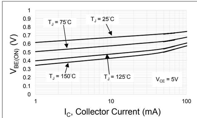
**Fig.4 Typical Base - Emitter Voltage vs Collector Current**
