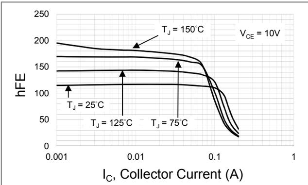
**Fig.3 Typical DC Current Gain vs Collector Current**
