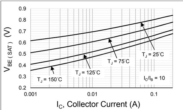
**Fig.1 Typical Base-Emitter Saturation Voltage**
