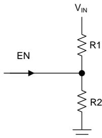
Figure 47. Undervoltage Lockout
