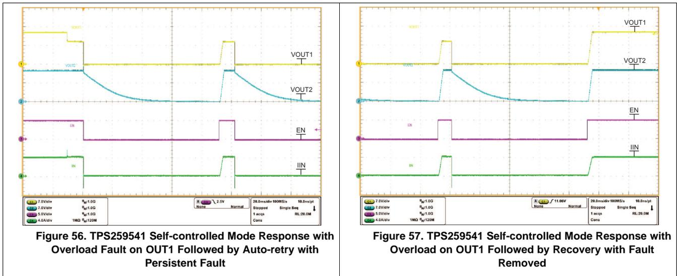
Figure 56. TPS259541 Self-controlled Mode Response with Overload Fault on OUT1 Followed by Auto-retry with Persistent Fault
