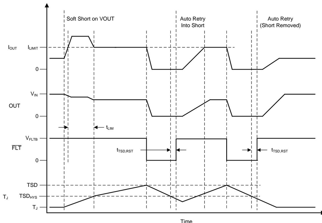
Figure 50. TPS2595x1, TPS2595x3, TPS2595x5 Overcurrent Response (Auto-Retry)
