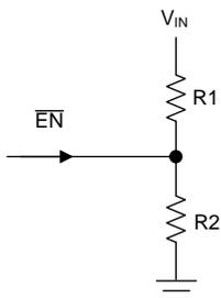
Figure 48. Overvoltage Lockout
