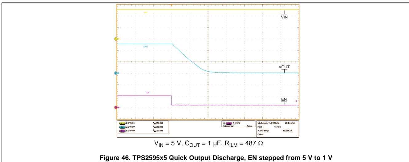
V<sub>IN</sub> = 5 V, C<sub>OUT</sub> = 1 μF, R<sub>ILM</sub> = 487 Ω
