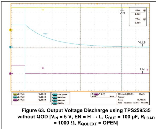
Figure 63. Output Voltage Discharge using TPS259535 without QOD [V<sub>IN</sub> = 5 V, EN = H → L, C<sub>OUT</sub> = 100 μF, R<sub>LOAD</sub> = 1000 Ω, R<sub>QODEXT</sub> = OPEN]
