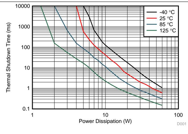
Figure 26. Thermal Shutdown Time vs Power Dissipation
