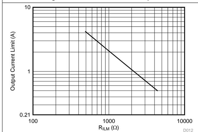
Figure 13. Output Current Limit ( $I_{LIMIT}$ ) vs  $R_{ILM}$
