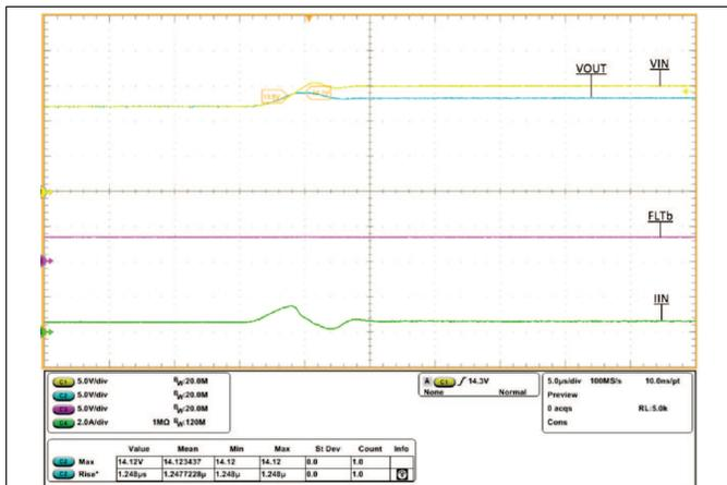
V<sub>IN</sub> Stepped from 12 V to 15 V, C<sub>OUT</sub> = 1 μF, R<sub>ILM</sub> = 487 Ω, FLT = 3.3 V through 10 kΩ, R<sub>OUT</sub> = 20 Ω
