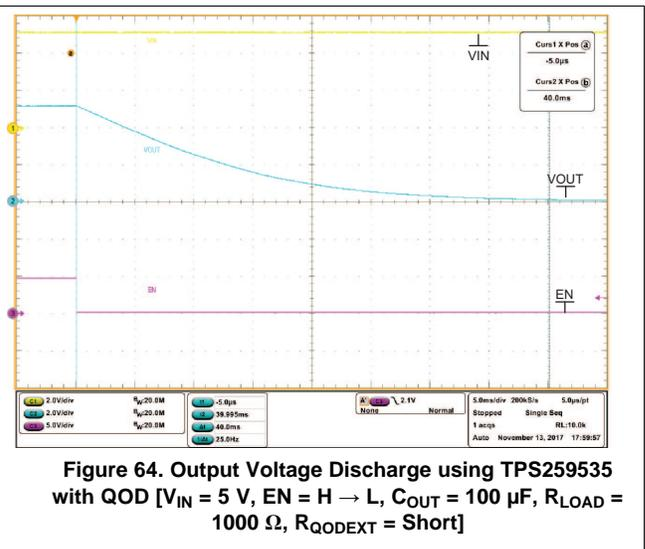
Figure 64. Output Voltage Discharge using TPS259535 with QOD [V<sub>IN</sub> = 5 V, EN = H → L, C<sub>OUT</sub> = 100 μF, R<sub>LOAD</sub> = 1000 Ω, R<sub>QODEXT</sub> = Short]
