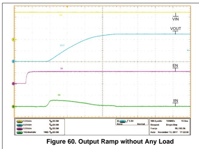
Figure 60. Output Ramp without Any Load
