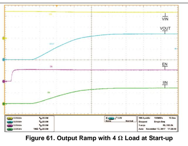
Figure 61. Output Ramp with 4 Ω Load at Start-up
