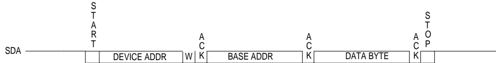
Figure 16-128. Byte Write to Device with Internal Addresses
