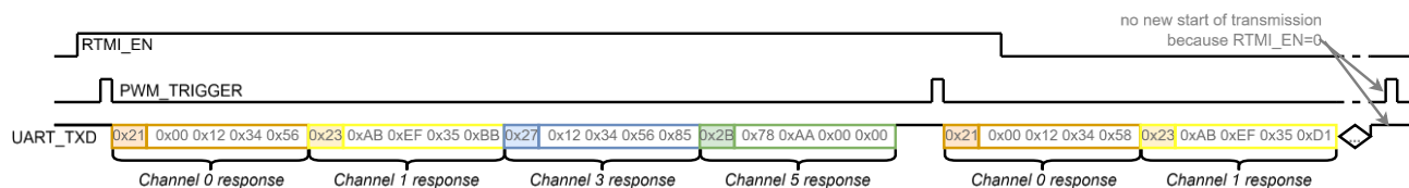
Figure 22. Example of a UART Stream Channel Response Datagram
