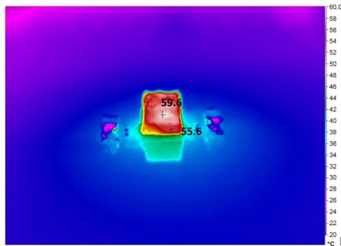
Figure 29. Thermal Image at 12V IN , 1V, 15A Output, No Airflow and Heat Sink, T_A = 25^{\circ}\text{C} .
