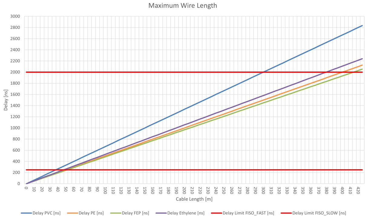
Figure 54. Maximum wire length according to wire insulator and operating frequency
