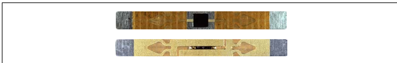
Figure 1: Pin Configuration Module Contactless Card – MFCC1 (top / bottom view)
