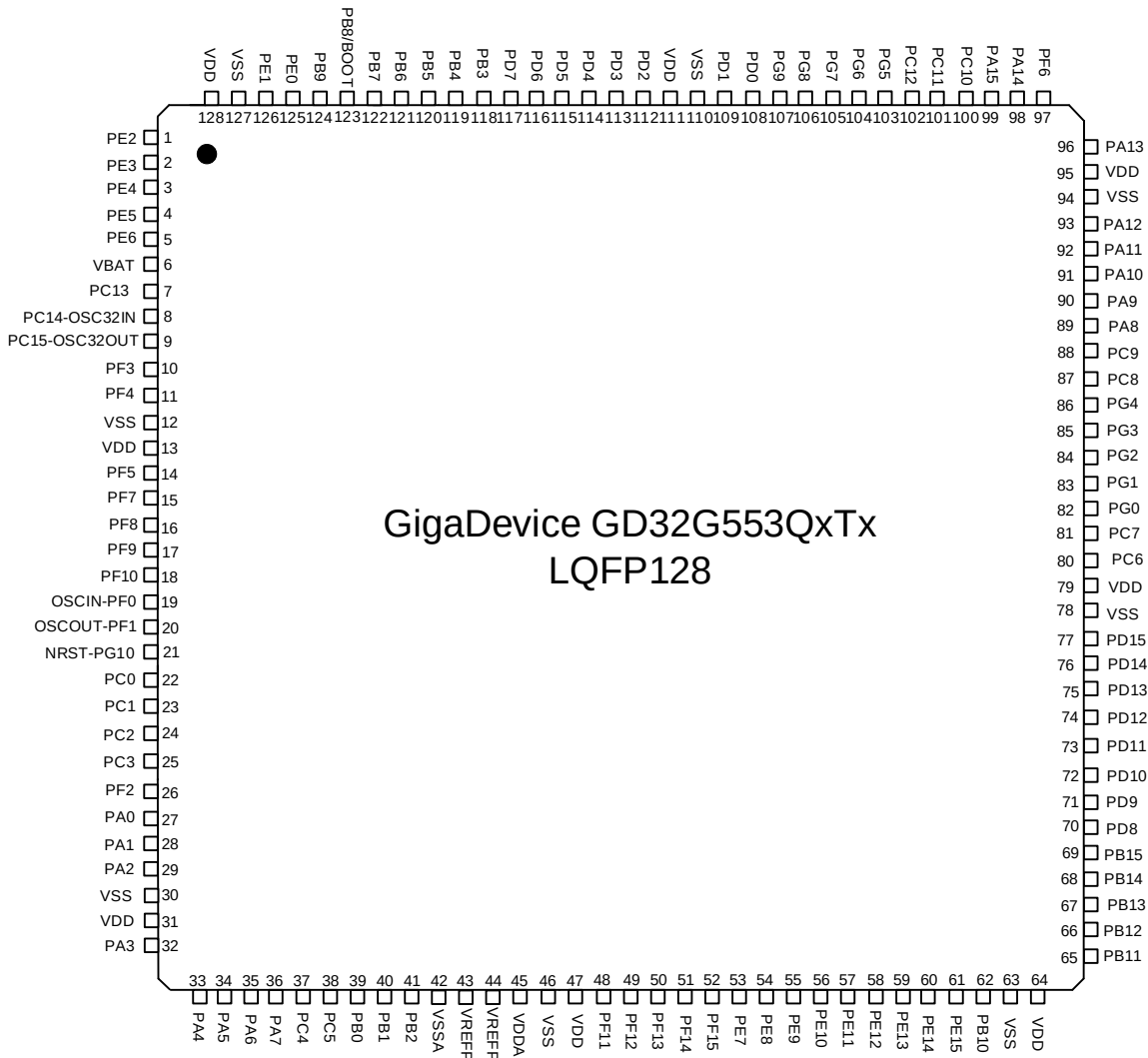
Figure 2-2. GD32G553QxTx LQFP128 pinouts (1)
