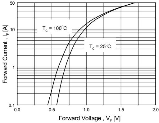
**Figure 1. Typical Forward Voltage Drop vs. Forward Current**
