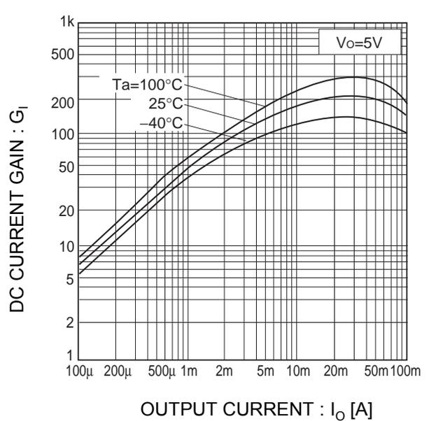
●Electrical characteristic curves( $T_a = 25^\circ\text{C}$ )
