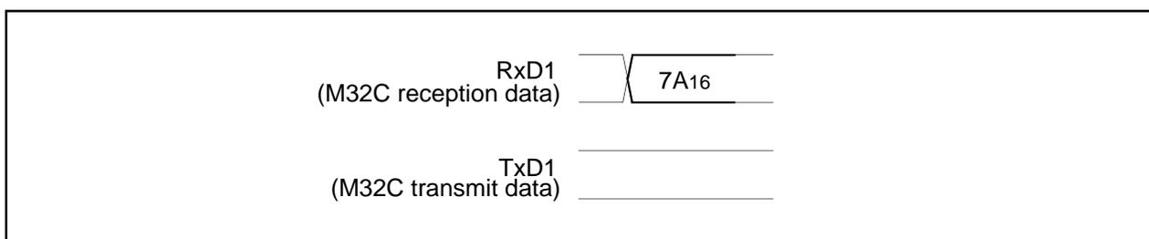
Figure 1.35.32. Timing for enabling the lock bit
