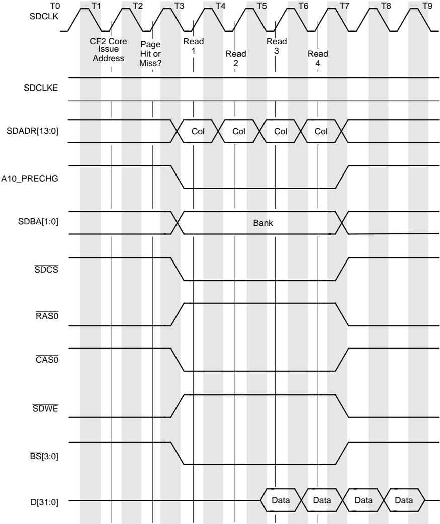
**Figure 9-10. SDRAM Burst Read, 32-Bit Port, Page Hit, Access = 5-1-1-1**
