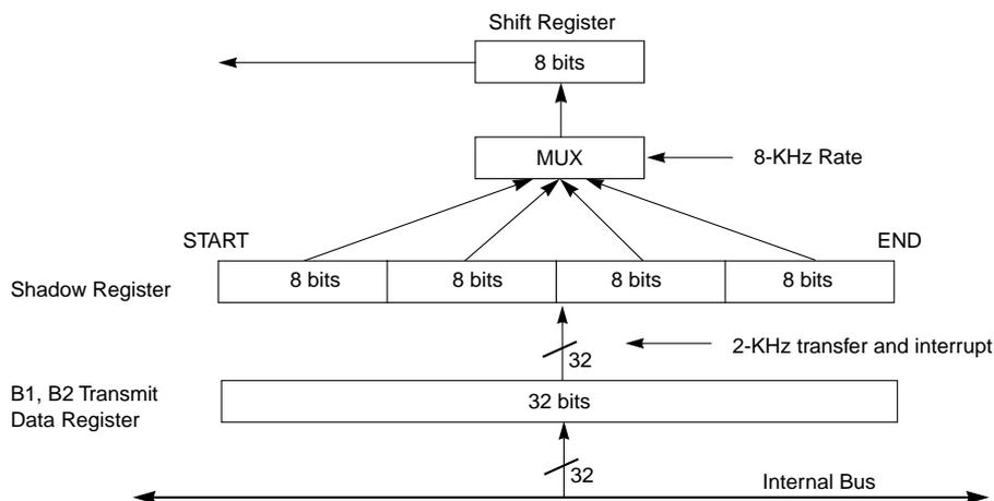
**Figure 13-5. GCI/IDL B Data Transmit Register Multiplexing**
