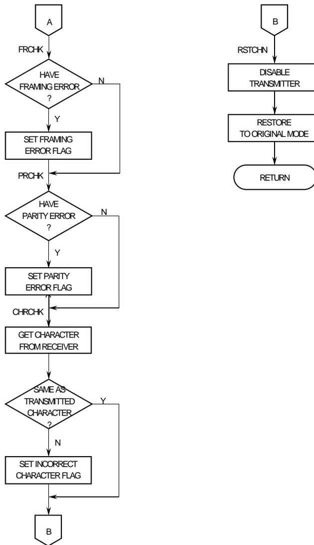
Figure 16-31. UART Mode Programming Flowchart (Sheet 3 of 5)
