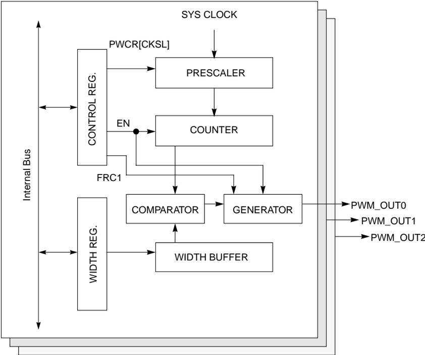
Figure 18-1. PWM Block Diagram (3 Identical Modules)
