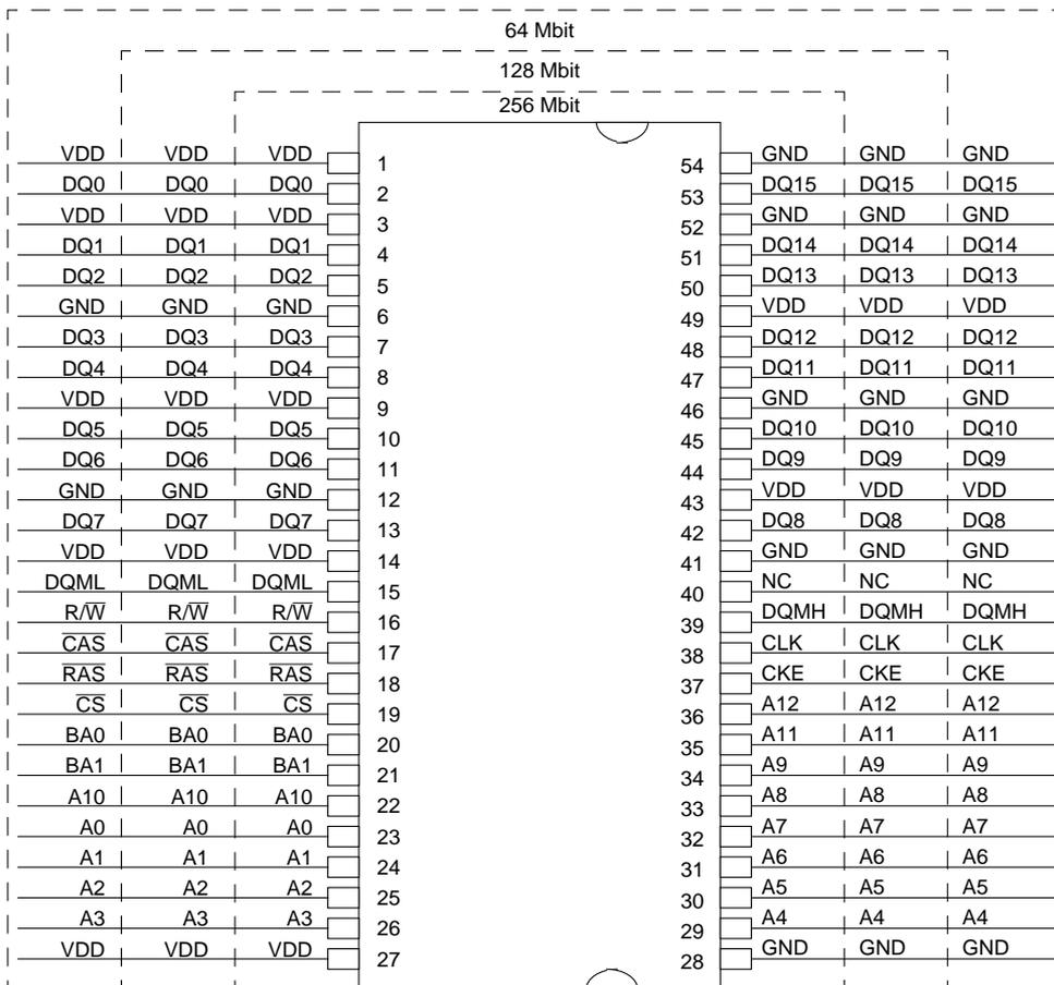
**Figure 9-2. 54-Pin TSOP SDRAM Pin Definition**
