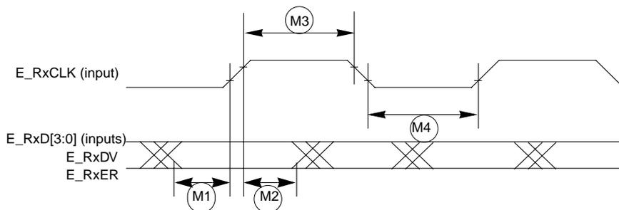
**Figure 23-11. MII Receive Signal Timing Diagram**
