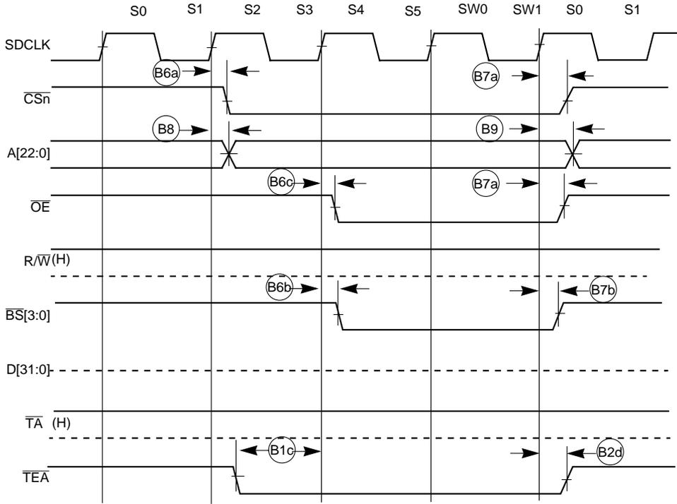
Figure 23-5. SRAM Bus Cycle Terminated by  $\overline{TEA}$
