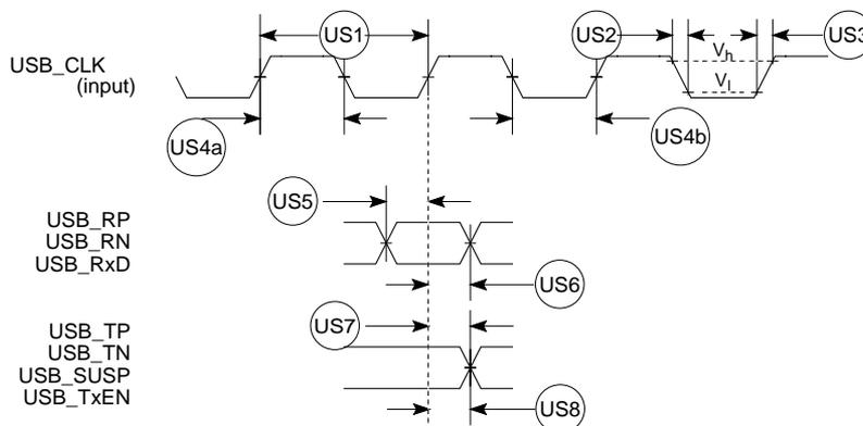
**Figure 23-22. USB Interface Timing**
