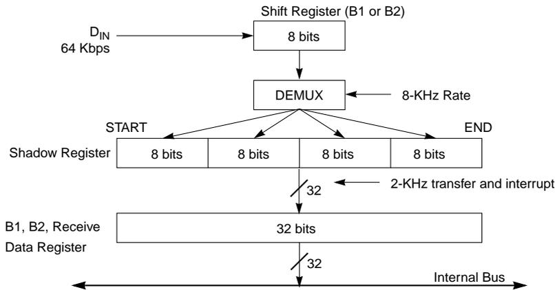
Figure 13-3. GCI/IDL B-Channel Receive Data Register Demultiplexing
