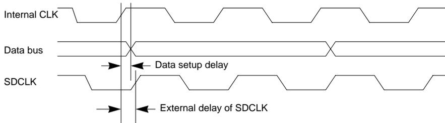
**Figure 9-5. Example Setup Time Violation on SDRAM Data Input during Write**
