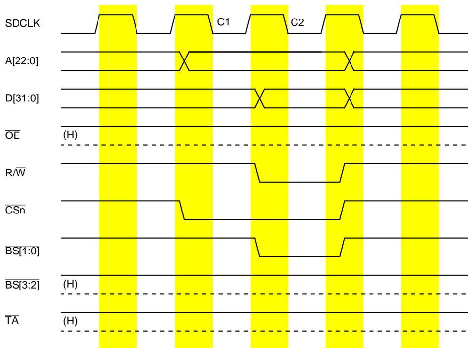
**Figure 20-4. Word Write; EBI = 00; 16-/32-Bit Port; Internal Termination**
