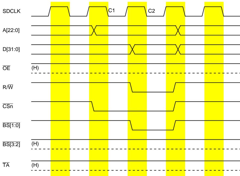
**Figure 20-11. Word Write; EBI=11; 16/32-Bit Port; Internal Termination**
