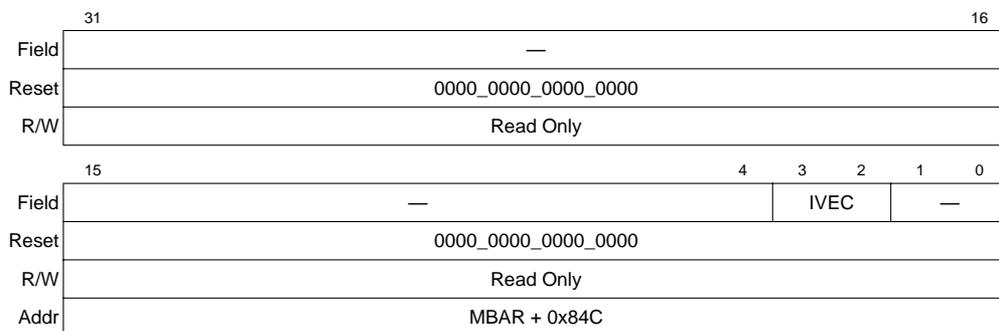
Figure 11-7. Interrupt Vector Status Register (IVSR)
