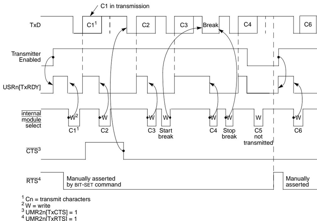
**Figure 16-25. Transmitter Timing**
