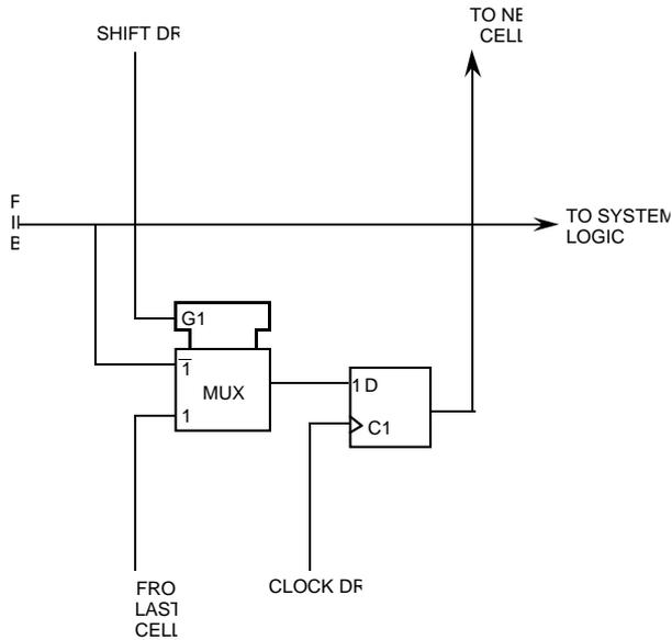
**Figure 21-4. Input Cell (I.Cell). Observe only (BC-4)**
