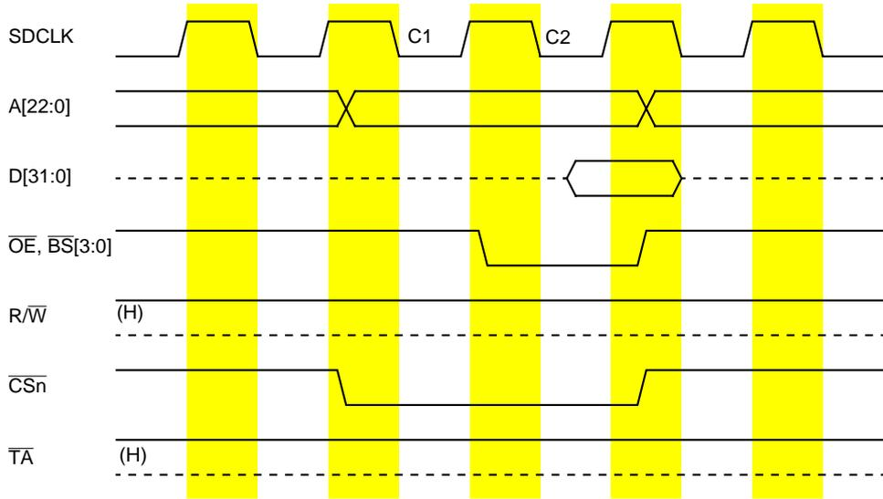
Figure 20-3. Longword Read; EBI = 00; 32-Bit Port; Internal Termination
