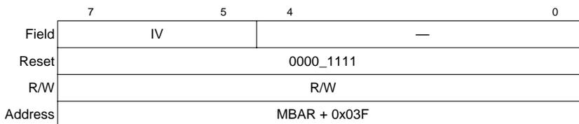
**Figure 7-9. Programmable Interrupt Vector Register (PIVR)**
