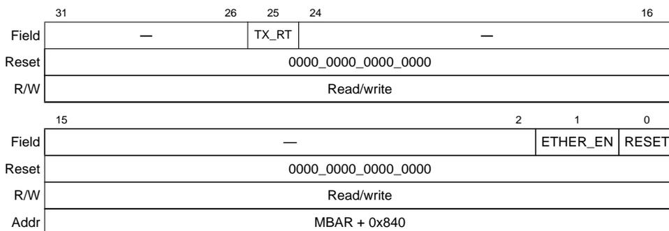
Figure 11-5. Ethernet Control Register (ECR)
