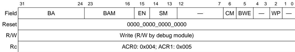
**Figure 4-5. Access Control Register Format (ACR<sub>n</sub>)**
