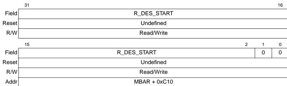
Figure 11-23. Pointer to Receive Descriptor Ring (ERDSR)
