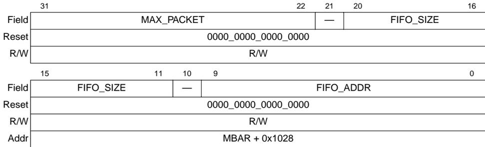
**Figure 12-13. USB Endpoint 0 IN Configuration Register (IEP0CFG)**
