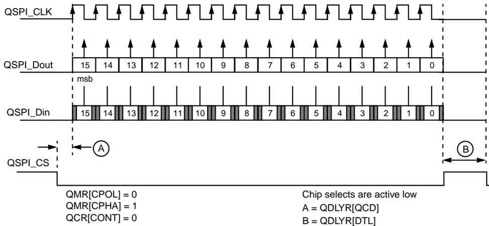
Figure 14-4. QSPI Clocking and Data Transfer Example
