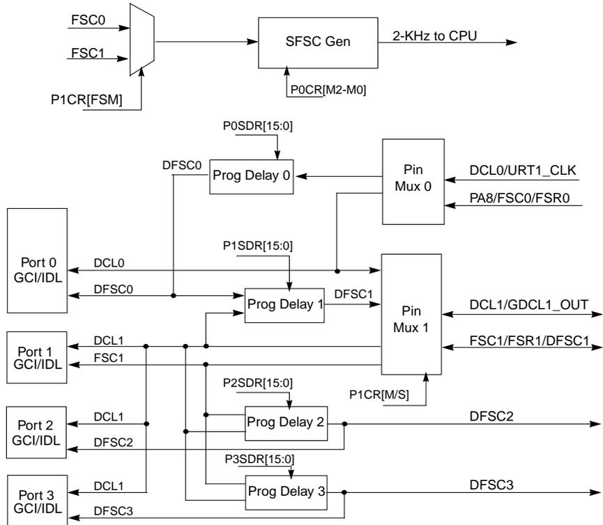
Figure 13-11. PLIC Internal Timing Signal Routing
