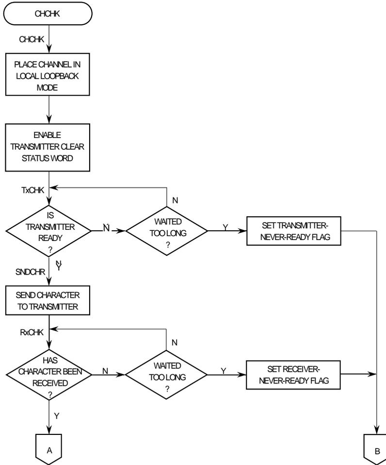
Figure 16-31. UART Mode Programming Flowchart (Sheet 2 of 5)
