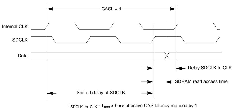
**Figure 9-8. Timing Refinement with Effective CAS Latency**
