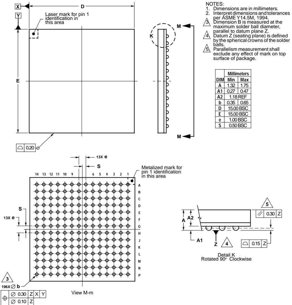
Figure 22-2. 196 MAPBGA Package Dimensions (Case No. 1128A-01)
