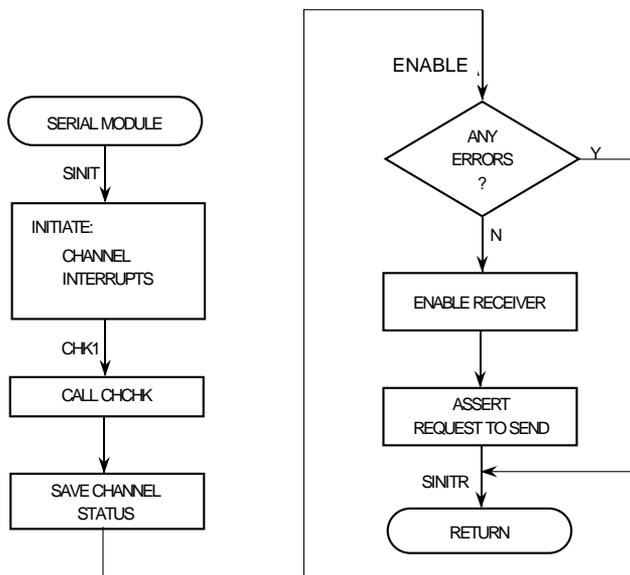
**Figure 16-31. UART Mode Programming Flowchart (Sheet 1 of 5)**
