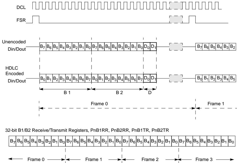
**Figure 13-6. B-Channel Unencoded and HDLC Encoded Data**
