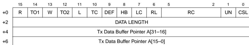
**Figure 11-27. Transmit Buffer Descriptor (TxBD)**
