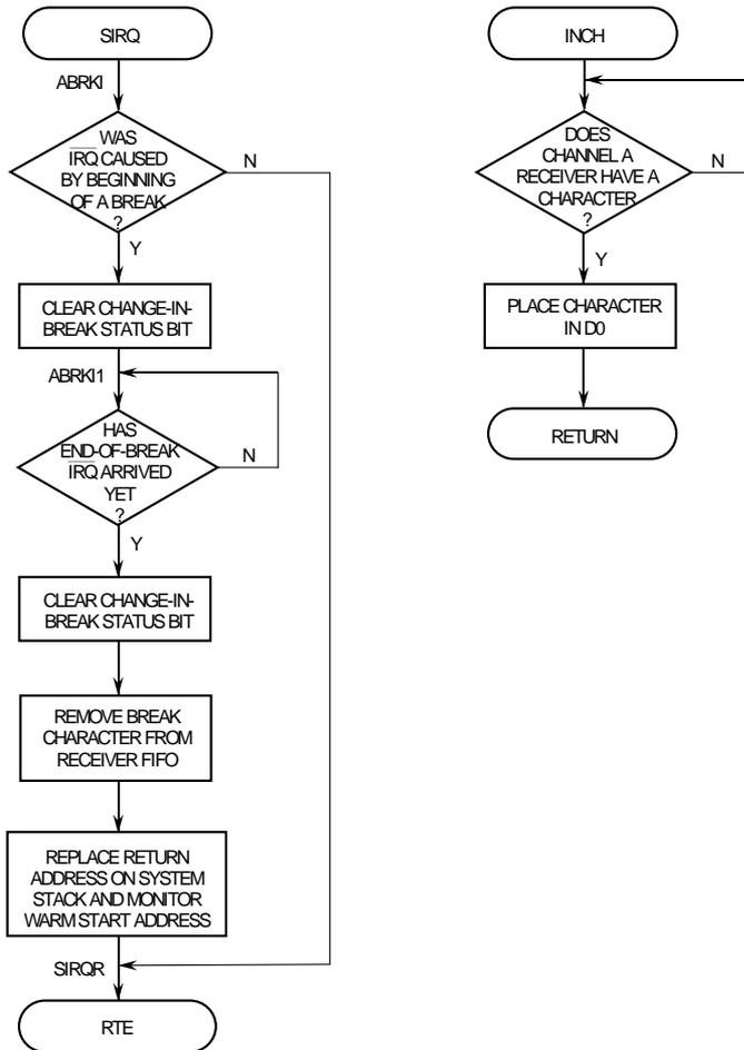
Figure 16-31. UART Mode Programming Flowchart (Sheet 4 of 5)
