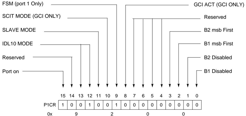
**Figure 13-35. Port 1 Configuration Register (P1CR)**
