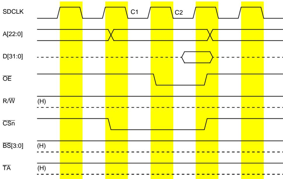
Figure 20-10. Longword Read; EBI=11; 32-Bit Port; Internal Termination
