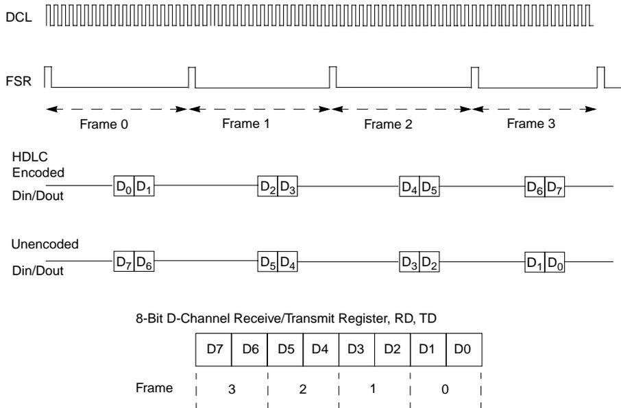
Figure 13-7. D-Channel HDLC Encoded and Unencoded Data.
