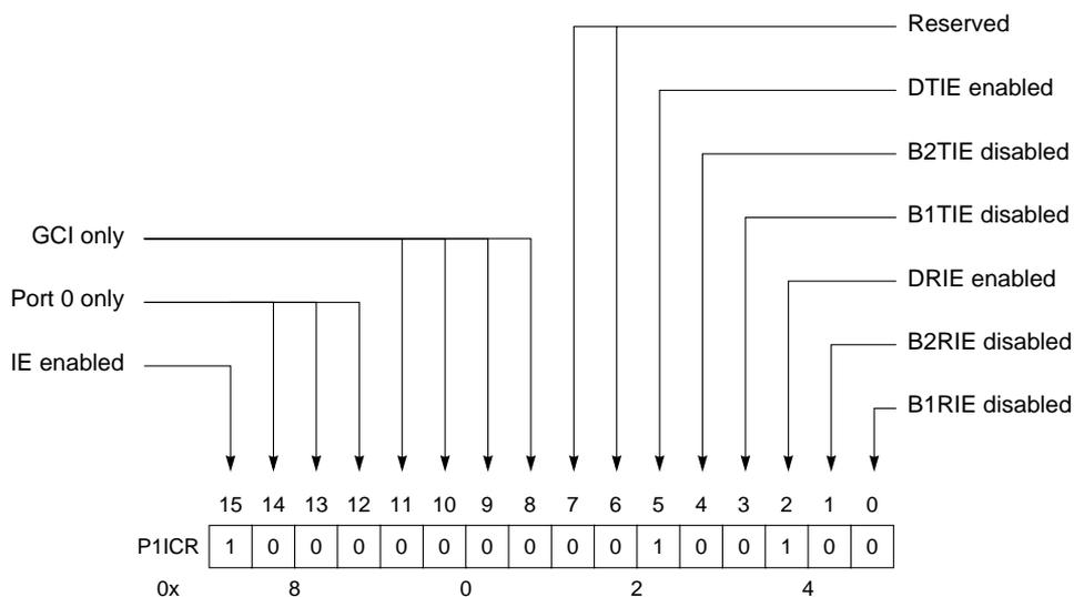
**Figure 13-36. Port 1 Interrupt Configuration Register (P1ICR)**
