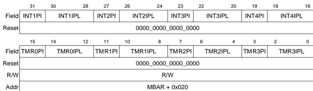
**Figure 7-2. Interrupt Control Register 1 (ICR1)**
