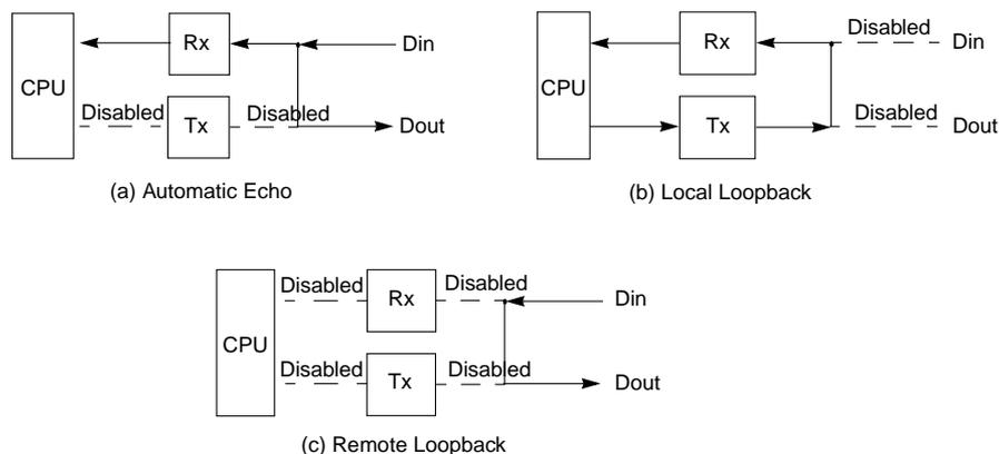
Figure 13-9. GCI/IDL Loopback Mode
