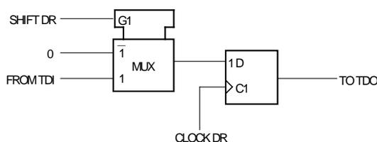
Figure 21-8. Bypass Register
