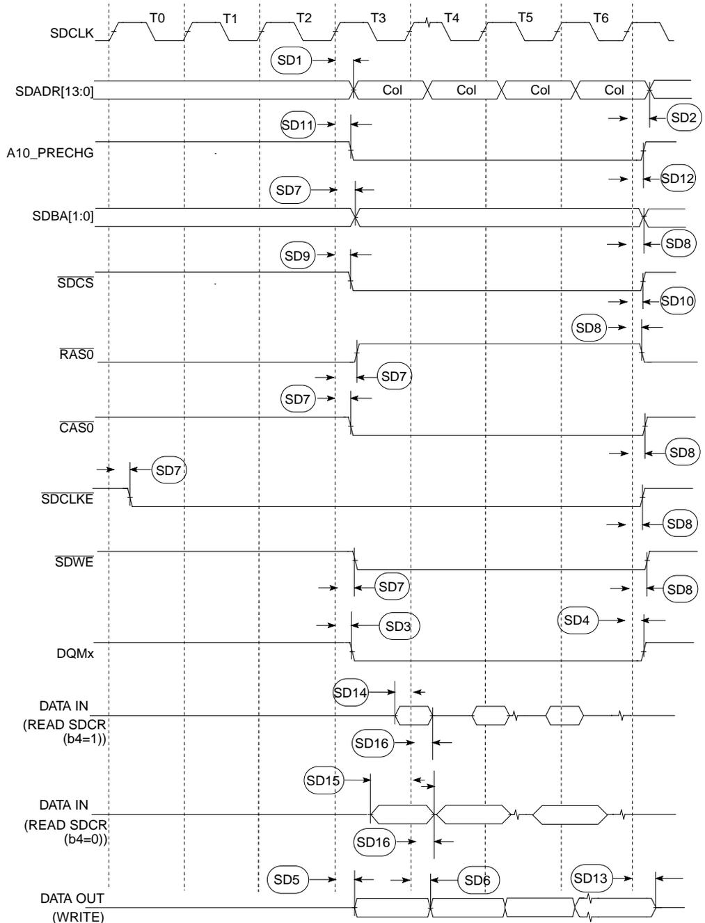
Figure 23-9. SDRAM Signal Timing
