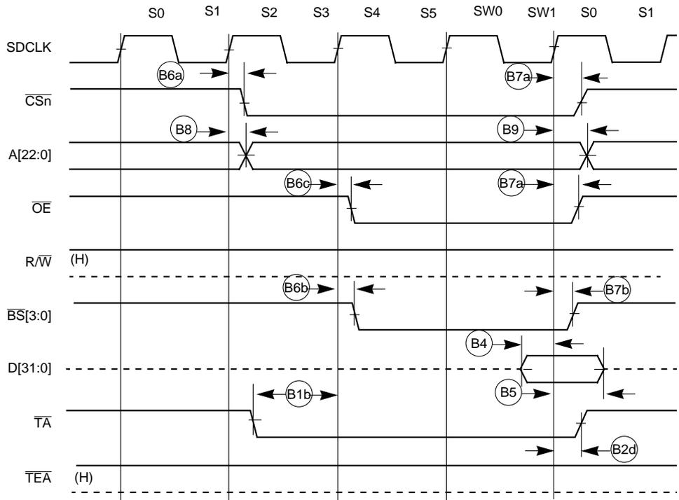
Figure 23-4. SRAM Bus Cycle Terminated by  $\overline{TA}$
