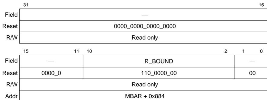
**Figure 11-12. FIFO Receive Bound Register (FRBR)**
