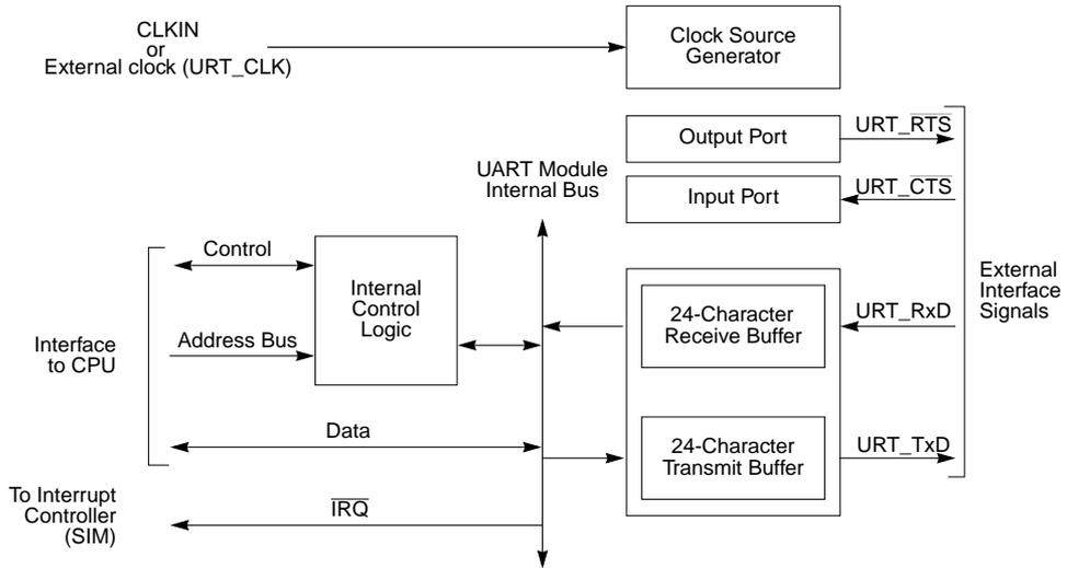
**Figure 16-21. UART Block Diagram Showing External and Internal Interface Signals**
