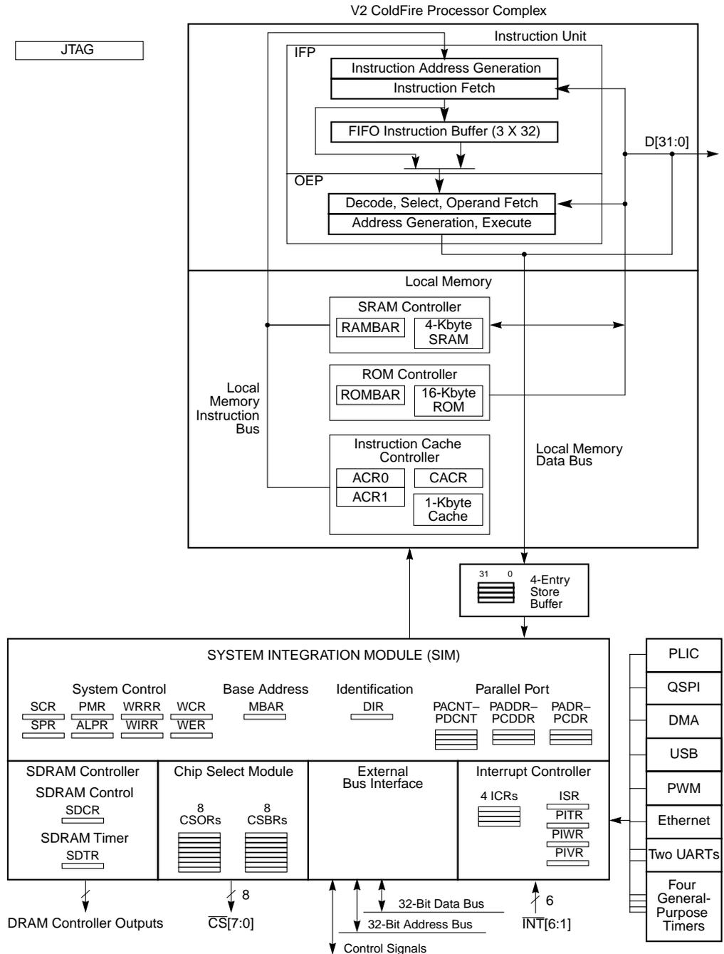
Figure 1-1. MCF5272 Block Diagram
