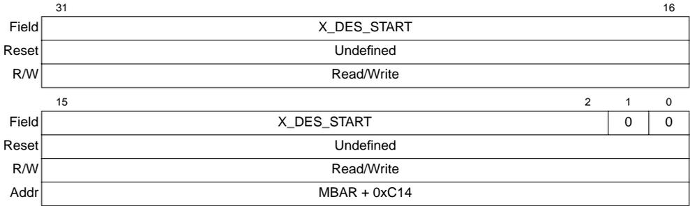
Figure 11-24. Pointer to Transmit Descriptor Ring (ETDSR)
