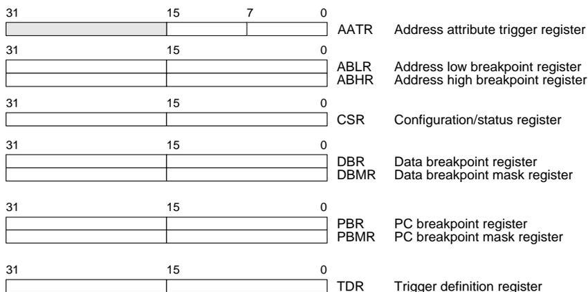
Note: Each debug register is accessed as a 32-bit register; shaded fields above are not used (don't care). All debug control registers are writable from the external development system or the CPU via the WDEBUI instruction. CSR is write-only from the programming model. It can be read or written through the BDM port using the RDMREG and WDMREG commands.
