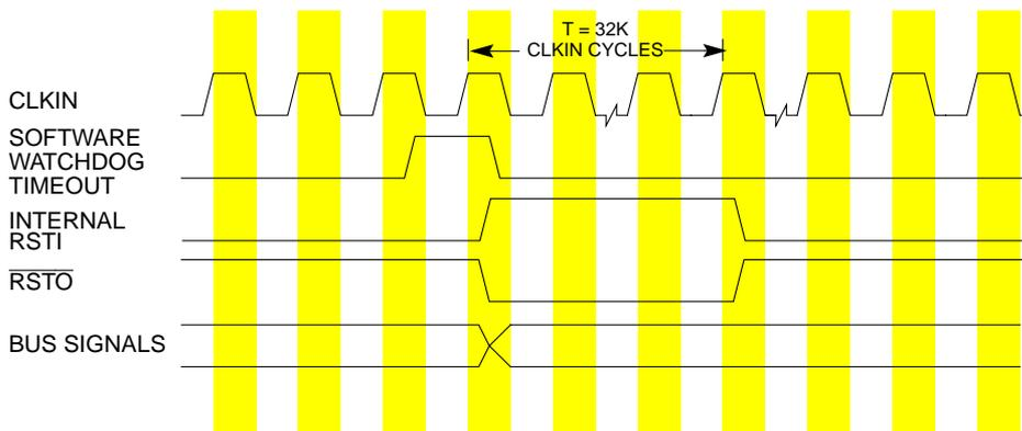
Figure 20-23. Software Watchdog Timer Reset Timing
