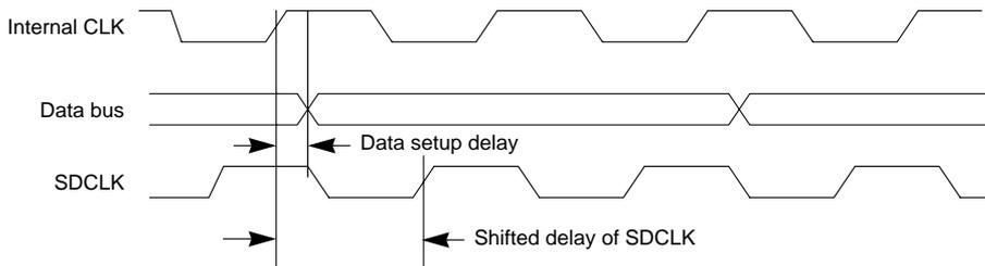
**Figure 9-6. Timing Refinement with Inverted SDCLK**
