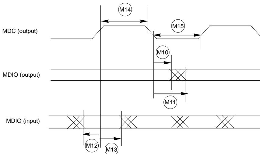
**Figure 23-14. MII Serial Management Channel Timing Diagram**
