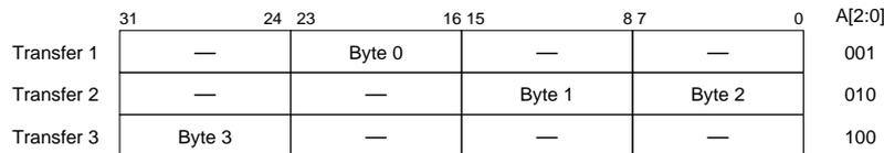
**Figure 20-18. Example of a Misaligned Longword Transfer**
