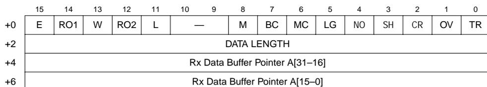
**Figure 11-26. Receive Buffer Descriptor (RxB D)**
