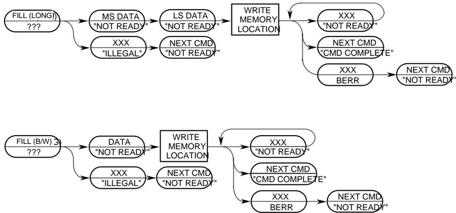
Figure 5-28. FILL Command Sequence
