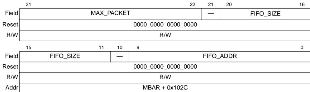
**Figure 12-14. USB Endpoint 0 OUT Configuration Register**
