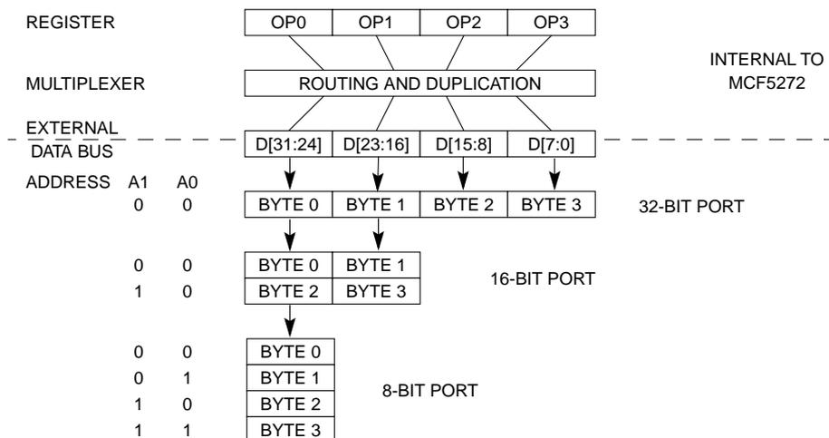
**Figure 20-2. MCF5272 Interface to Various Port Sizes**
