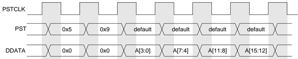
**Figure 5-3. Example JMP Instruction Output on PST/DDATA**
