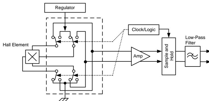
Figure 2. Chopper stabilization circuit (dynamic quadrature offset cancellation)
