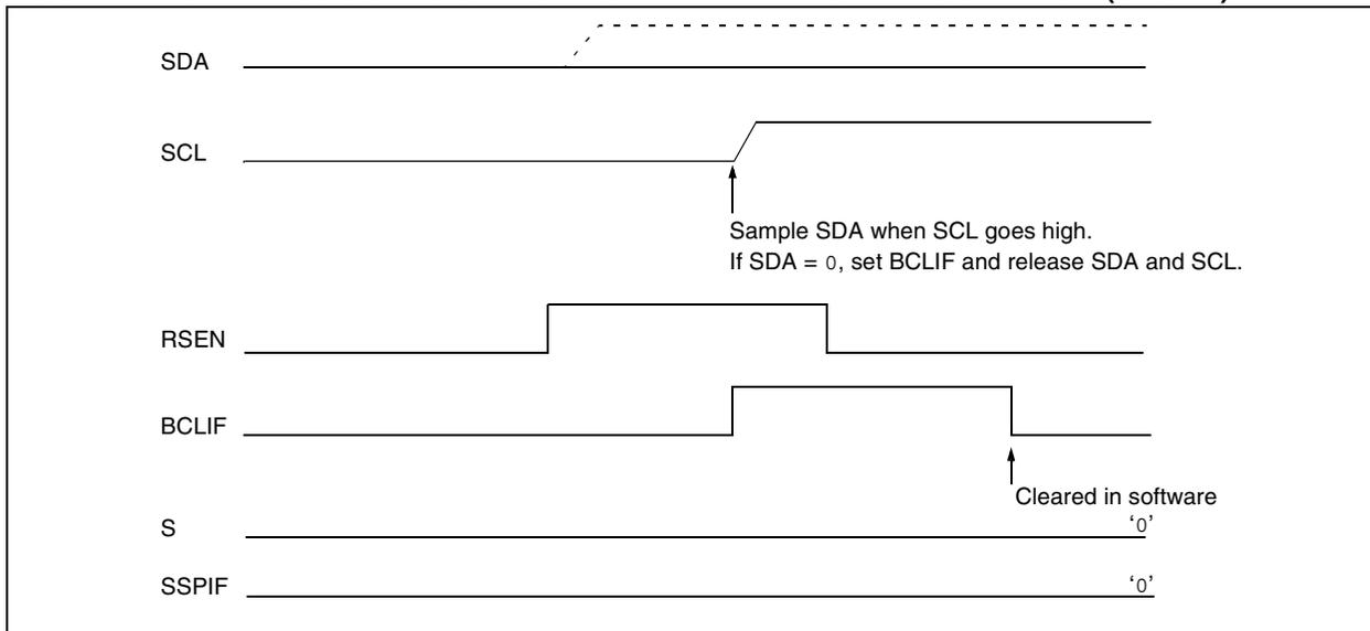
**FIGURE 17-30: BUS COLLISION DURING A REPEATED START CONDITION (CASE 2)**
