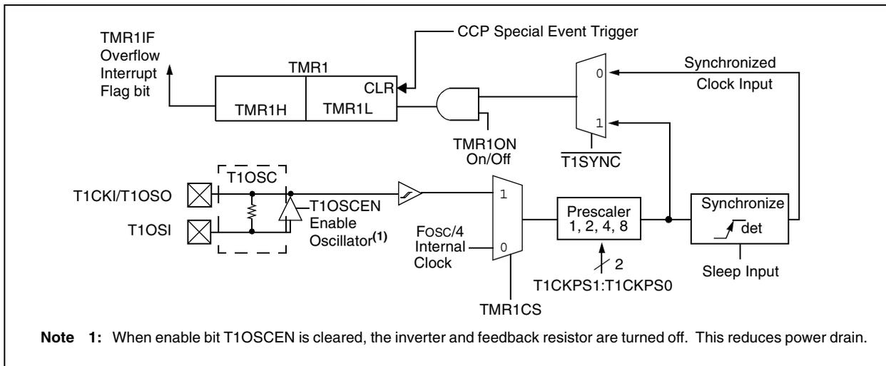
**FIGURE 12-2: TIMER1 BLOCK DIAGRAM: 16-BIT READ/WRITE MODE**
