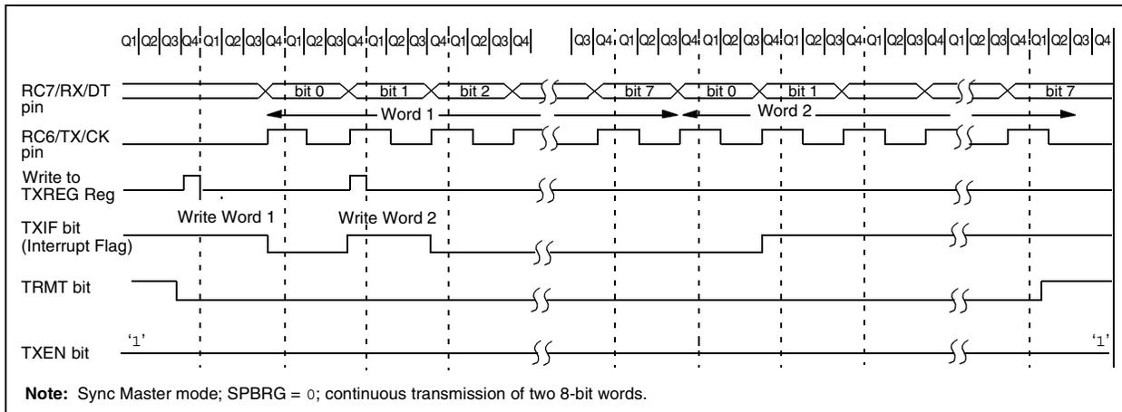
**FIGURE 18-7: SYNCHRONOUS TRANSMISSION (THROUGH TXEN)**
