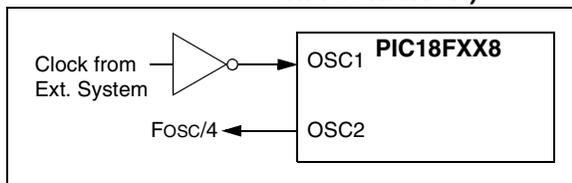
The ECIO Oscillator mode functions like the EC mode, except that the OSC2 pin becomes an additional general purpose I/O pin. Figure 2-4 shows the pin connections for the ECIO Oscillator mode.
