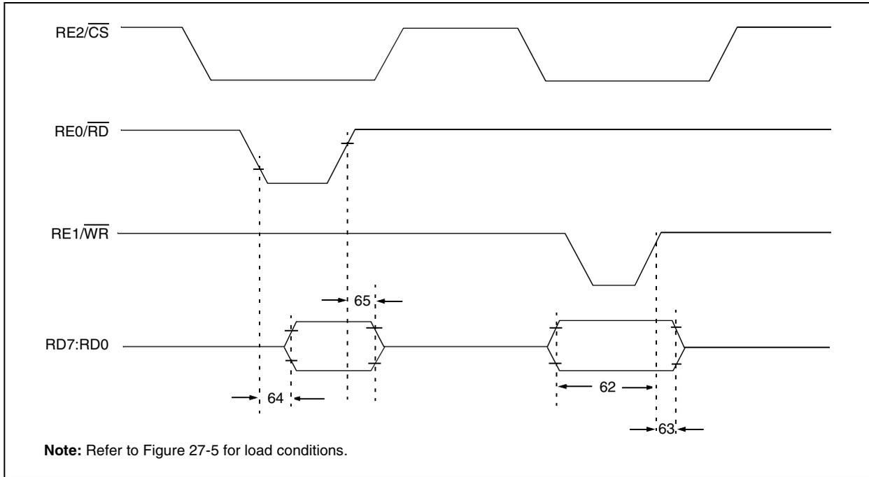
**TABLE 27-12: PARALLEL SLAVE PORT REQUIREMENTS (PIC18F248 AND PIC18F458)**
