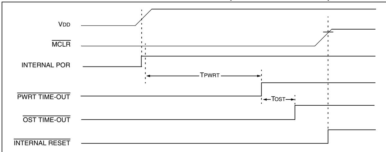
**FIGURE 3-6: SLOW RISE TIME ( $\overline{\text{MCLR}}$  TIED TO  $V_{DD}$ )**
