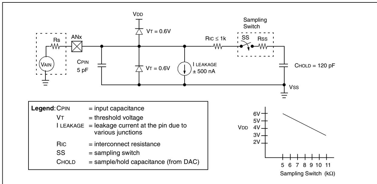
To calculate the minimum acquisition time, Equation 20-1 may be used. This equation assumes that 1/2 LSB error is used (1024 steps for the A/D). The 1/2 LSB error is the maximum error allowed for the A/D to meet its specified resolution.
