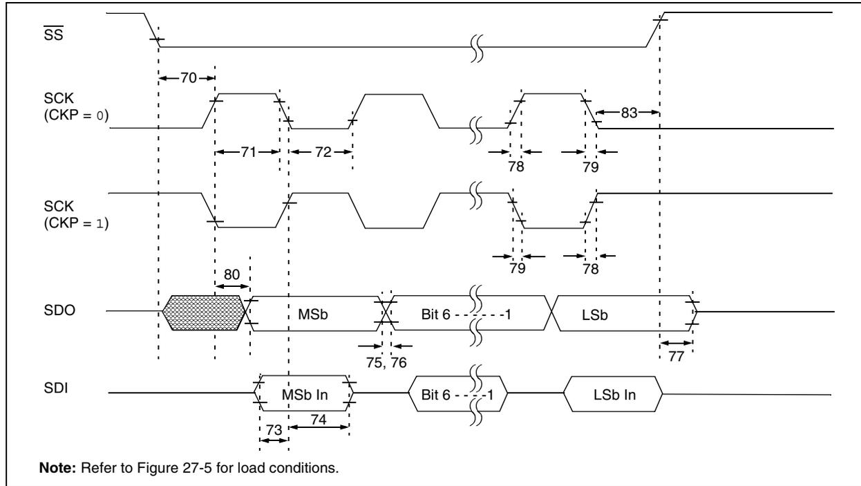
**TABLE 27-15: EXAMPLE SPI™ MODE REQUIREMENTS, SLAVE MODE TIMING (CKE = 0)**
