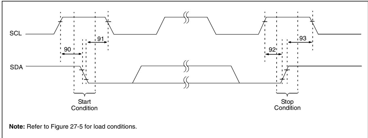
**TABLE 27-19: MASTER SSP I<sup>2</sup>C™ BUS START/STOP BITS REQUIREMENTS**
