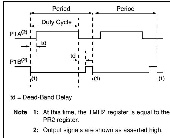
**FIGURE 16-4: EXAMPLES OF HALF-BRIDGE OUTPUT MODE APPLICATIONS**
