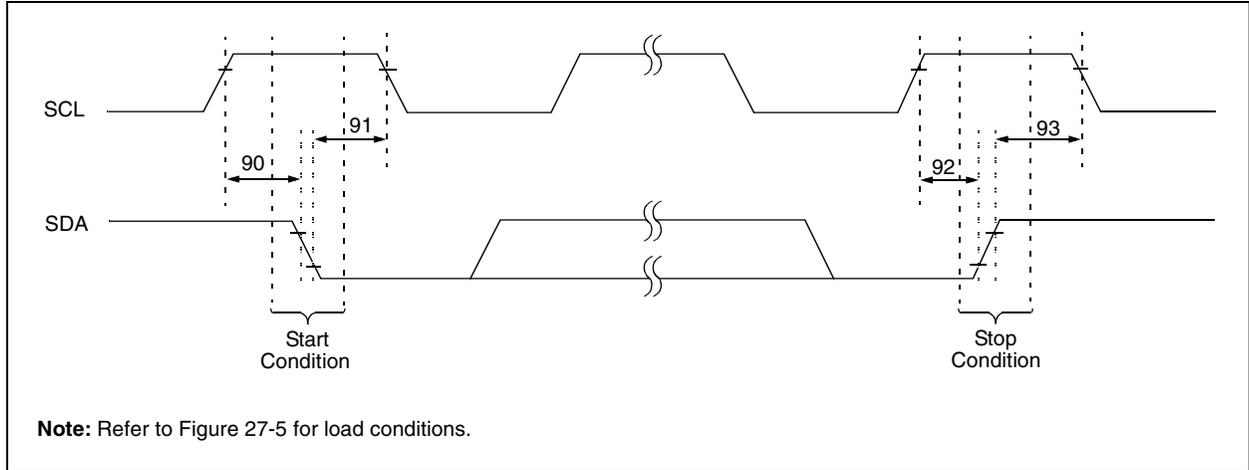
**TABLE 27-17: I<sup>2</sup>C™ BUS START/STOP BITS REQUIREMENTS (SLAVE MODE)**
