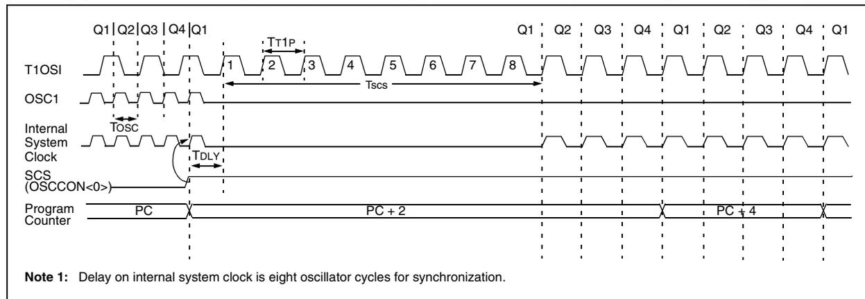
**FIGURE 2-8: TIMING DIAGRAM FOR TRANSITION BETWEEN TIMER1 AND OSC1 (HS, XT, LP)**
