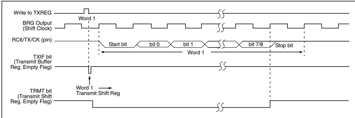
**FIGURE 18-3: ASYNCHRONOUS TRANSMISSION (BACK TO BACK)**
