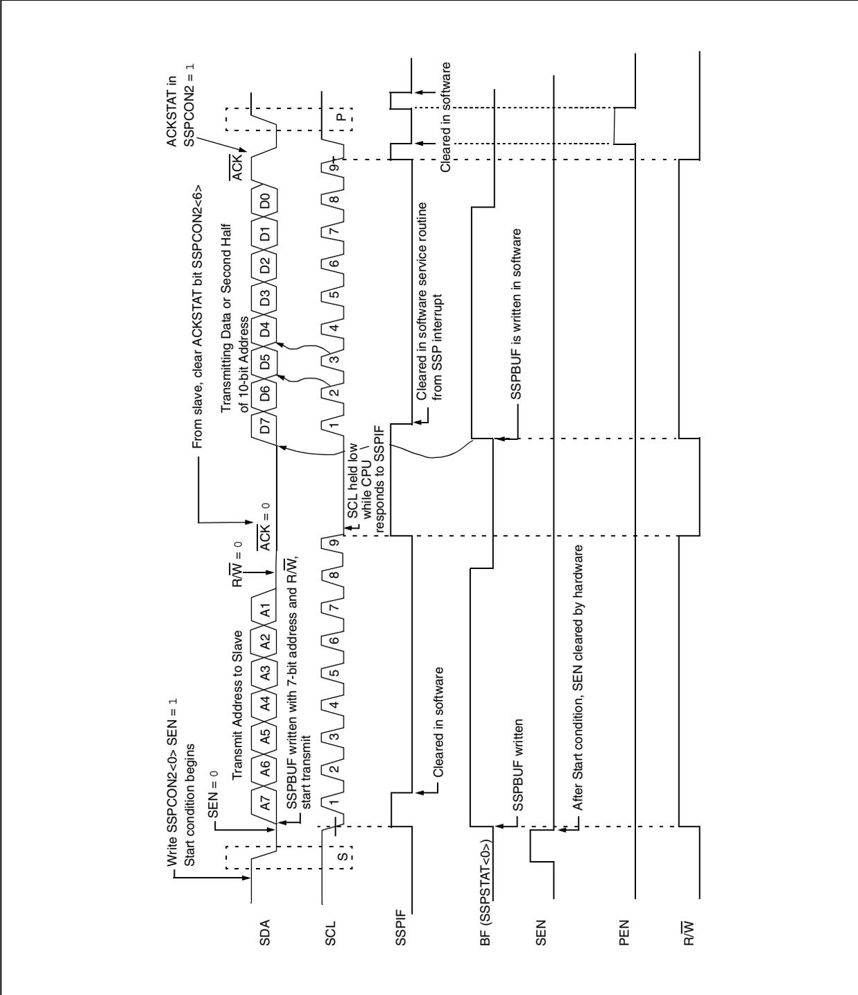
**FIGURE 17-22: I<sup>2</sup>C™ MASTER MODE WAVEFORM (RECEPTION, 7-BIT ADDRESS)**
