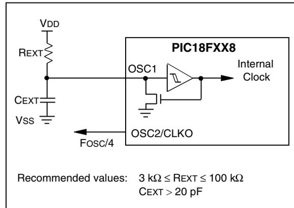
The RCIO Oscillator mode functions like the RC mode, except that the OSC2 pin becomes an additional general purpose I/O pin. The I/O pin becomes bit 6 of PORTA (RA6).
