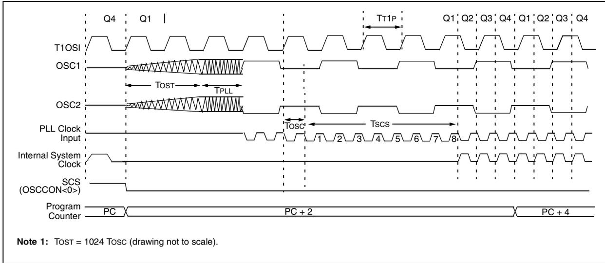
**FIGURE 2-10: TIMING FOR TRANSITION BETWEEN TIMER1 AND OSC1 (RC, EC)**
