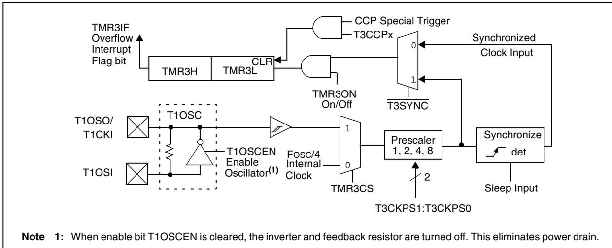
**FIGURE 14-2: TIMER3 BLOCK DIAGRAM CONFIGURED IN 16-BIT READ/WRITE MODE**
