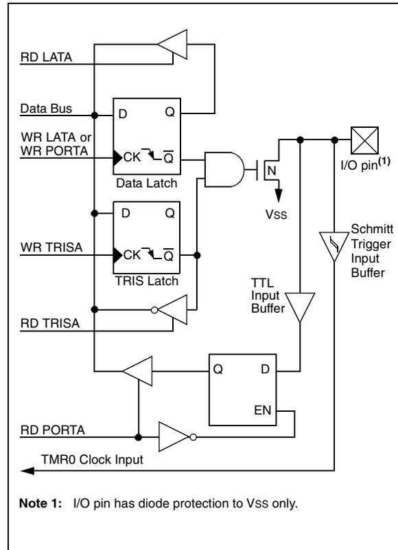
**FIGURE 9-3: OSC2/CLKO/RA6 PIN BLOCK DIAGRAM**
