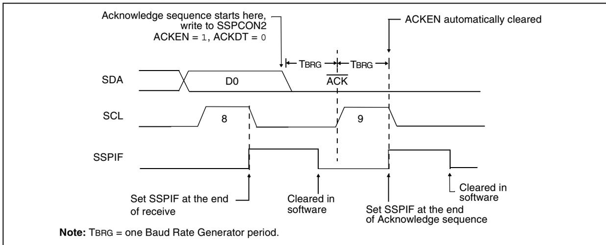
**FIGURE 17-24: STOP CONDITION RECEIVE OR TRANSMIT MODE**
