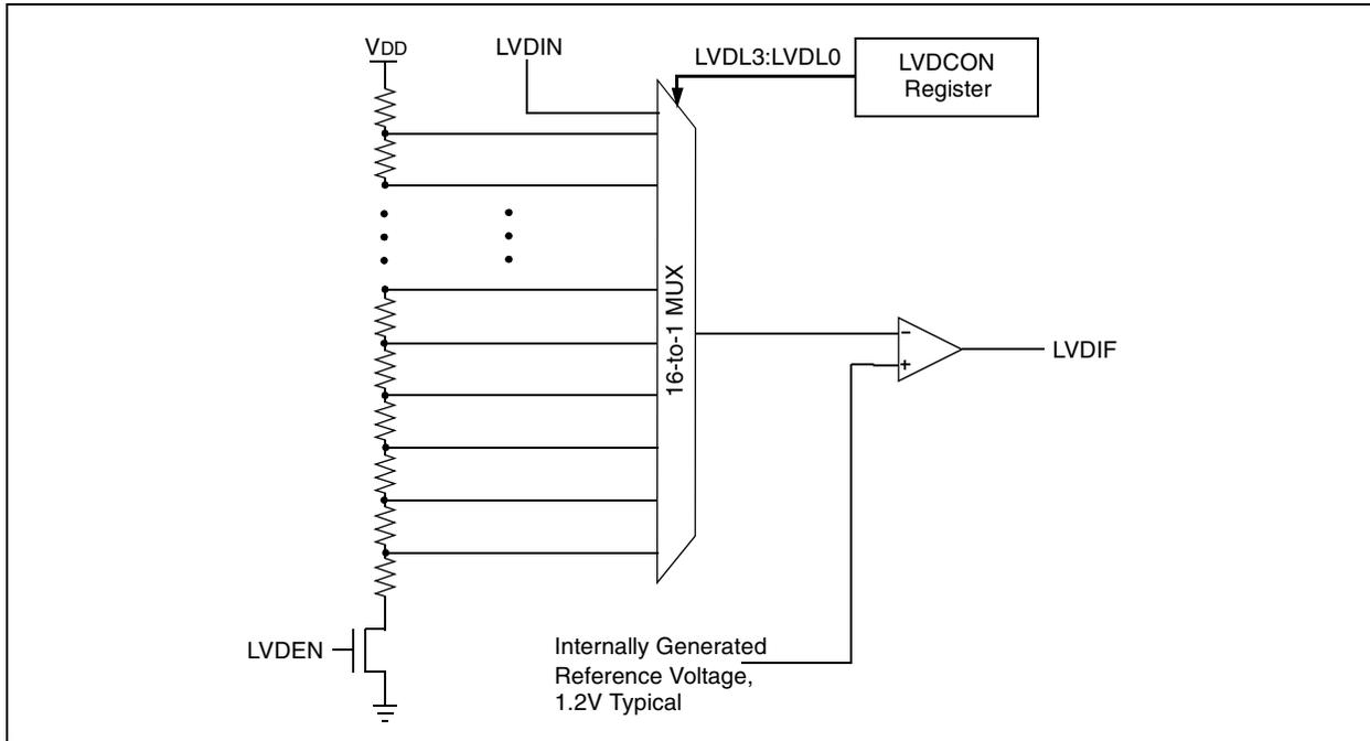
The LVD module has an additional feature that allows the user to supply the trip voltage to the module from an external source. This mode is enabled when bits LVDL3:LVDL0 are set to '1111'. In this state, the comparator input is multiplexed from the external input pin LVDIN to one input of the comparator (Figure 23-3).
