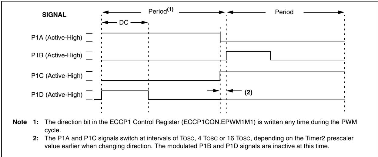
**FIGURE 16-8: PWM DIRECTION CHANGE AT NEAR 100% DUTY CYCLE**
