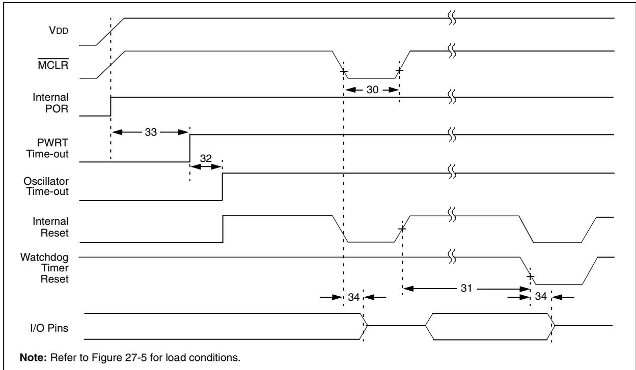
**FIGURE 27-9: BROWN-OUT RESET AND LOW-VOLTAGE DETECT TIMING**
