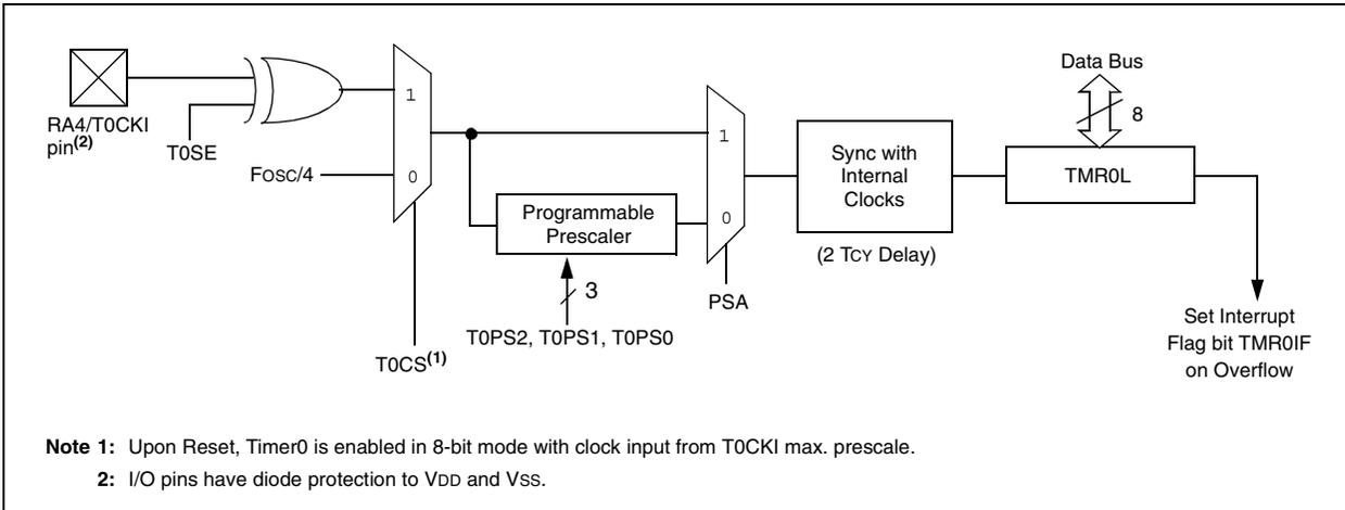
**FIGURE 11-2: TIMER0 BLOCK DIAGRAM IN 16-BIT MODE**
