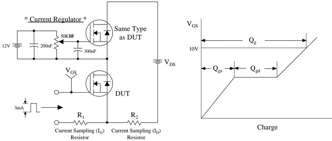
**Fig 13. Resistive Switching Test Circuit & Waveforms**
