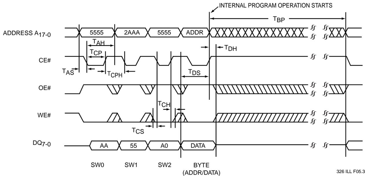
FIGURE 5: CE# CONTROLLED PROGRAM CYCLE TIMING DIAGRAM
