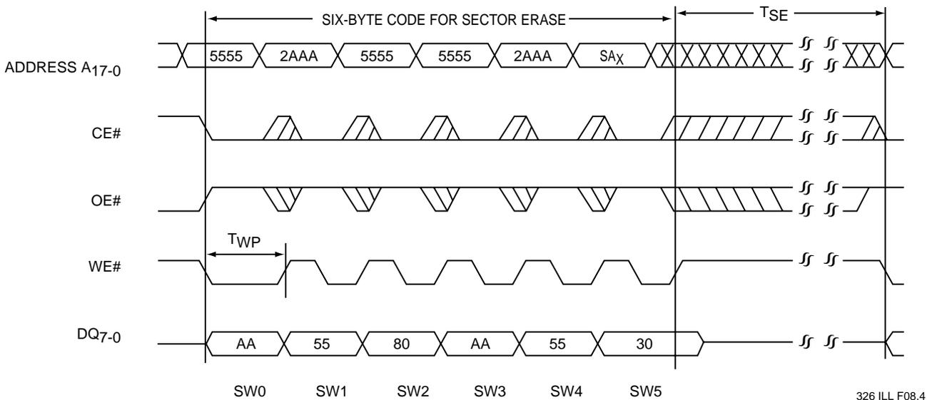
Note: The device also supports CE# controlled sector erase operation. The WE# and CE# signals are interchangeable as long as minimum timings are met. (See Table 10)
