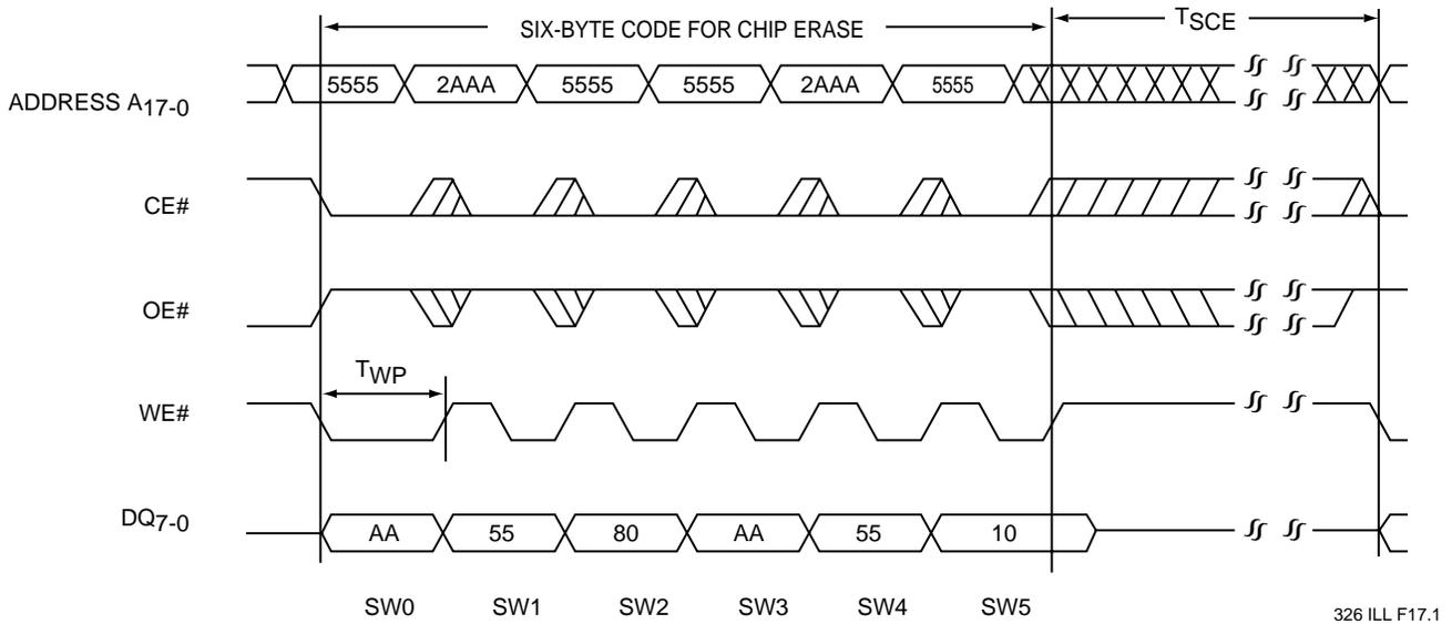
Note: The device also supports CE# controlled chip erase operation. The WE# and CE# signals are interchangeable as long as minimum timings are met. (See Table 10)
