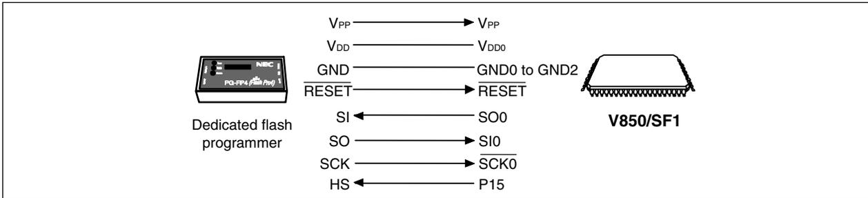
The dedicated flash programmer outputs the transfer clock, and the V850/SF1 operates as a slave.
