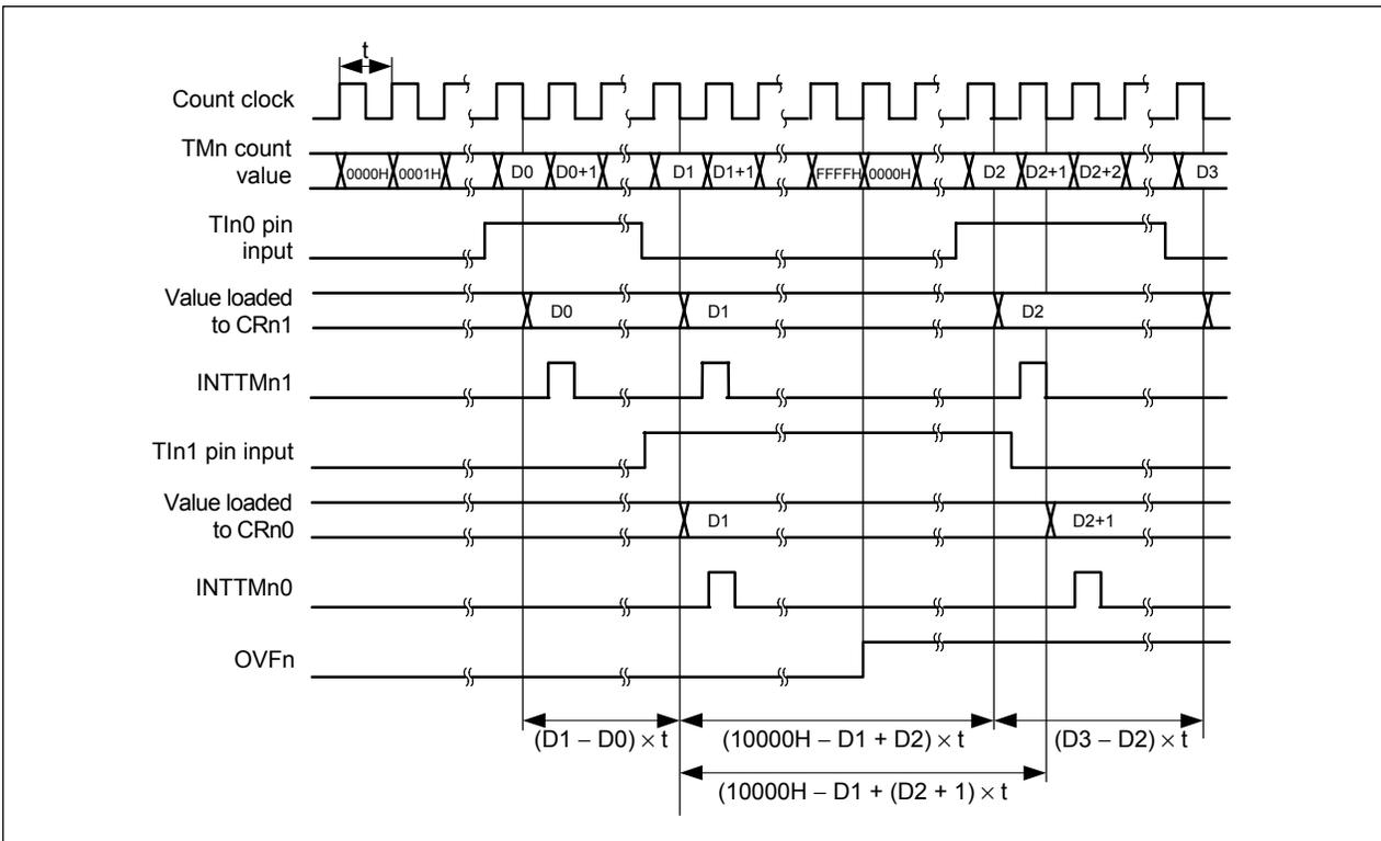
**(3) Pulse width measurement with free-running counter and two capture registers**
