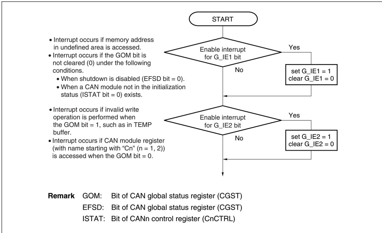
Figure 18-30. Setting of CAN Global Status Register (CGST)
