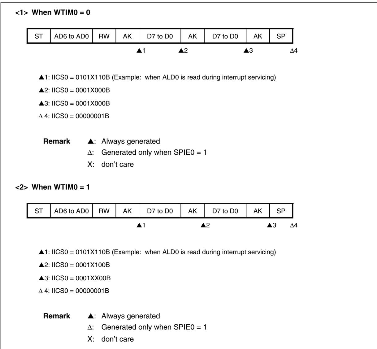
(b) When arbitration loss occurs during transmission of extension code
