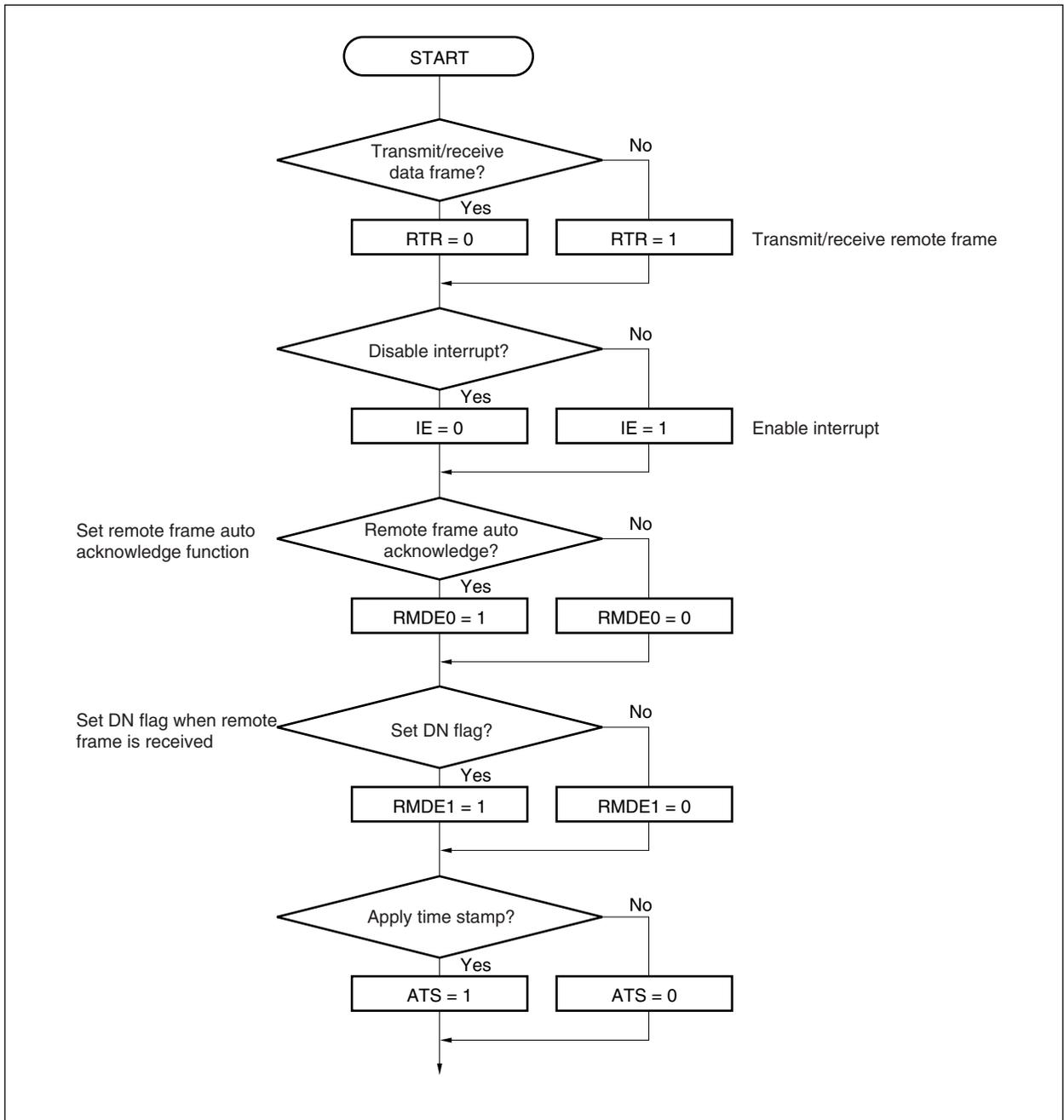
Figure 18-40. Setting of CAN Message Status Registers 00 to 31 (M\_STAT00 to M\_STAT31)
