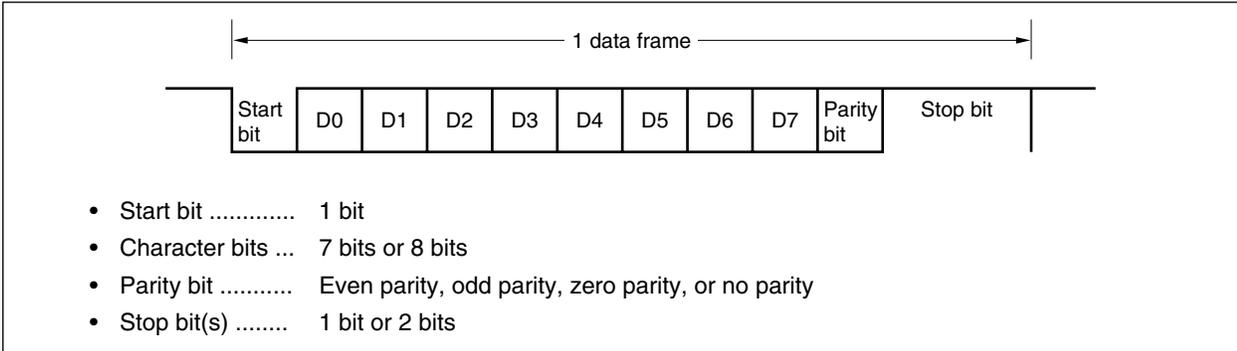
When 7 bits is selected as the number of character bits, only the lower 7 bits (from bit 0 to bit 6) are valid, so during a transmission the most significant bit (bit 7) is ignored and during reception the most significant bit (bit 7) must be set to 0.
