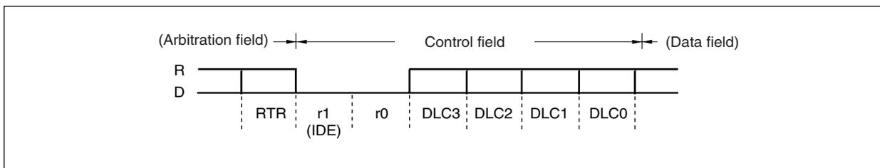
In standard format mode, the arbitration field’s IDE bit is the same bit as the r1 bit.
