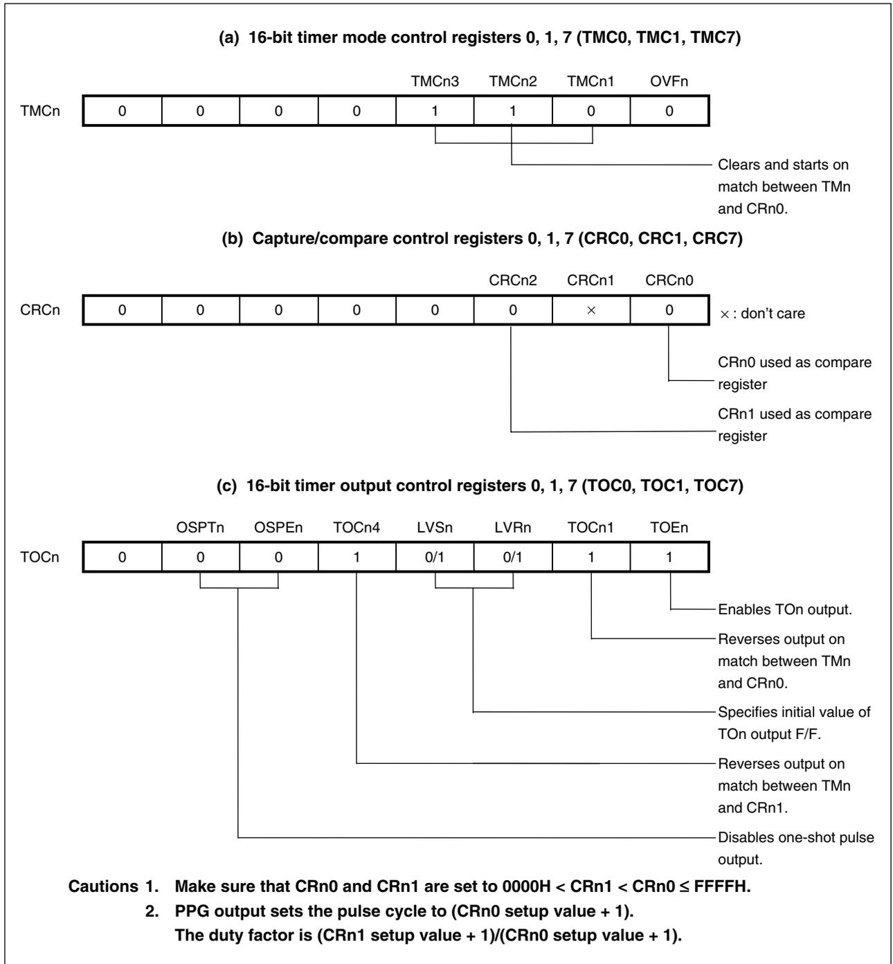
Figure 8-6. Configuration of PPG Output
