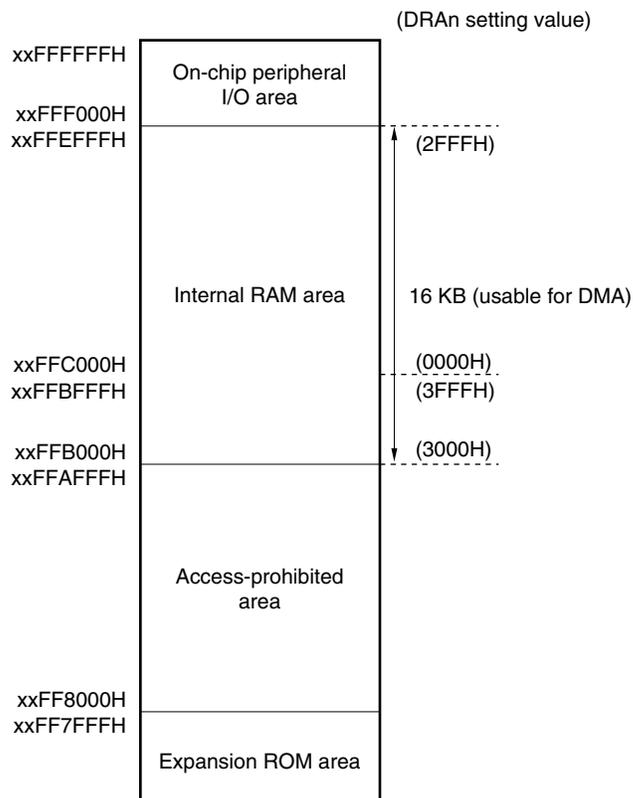
**Caution** Do not set odd addresses for 16-bit transfer (DCHCn register DS<sub>n</sub> = 1).
