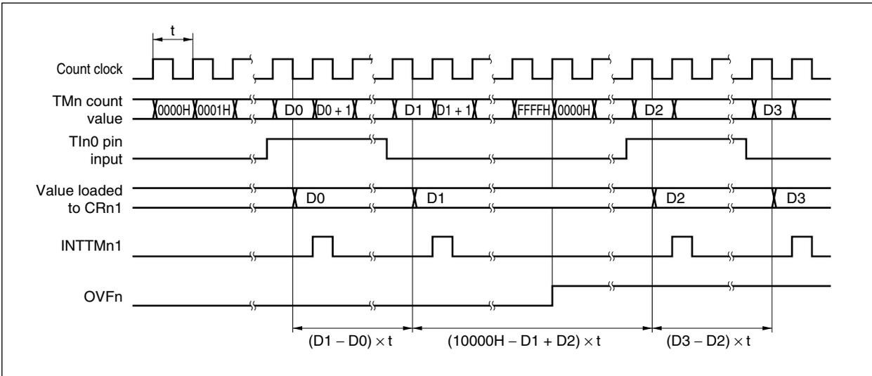
**(2) Measurement of two pulse widths with free-running counter**
