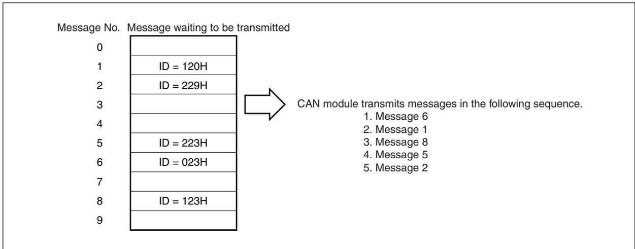
**Figure 18-9. Message Processing Example (When PBB Bit = 1)**
