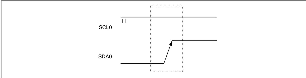
A stop condition is generated when bit 0 (SPT0) of IIC control register 0 (IICC0) is set to 1. When the stop condition is detected, bit 0 (SPD0) of IIC status register 0 (IICS0) is set to 1 and INTIIC0 is generated when bit 4 (SPIE0) of IICC0 is set to 1.
