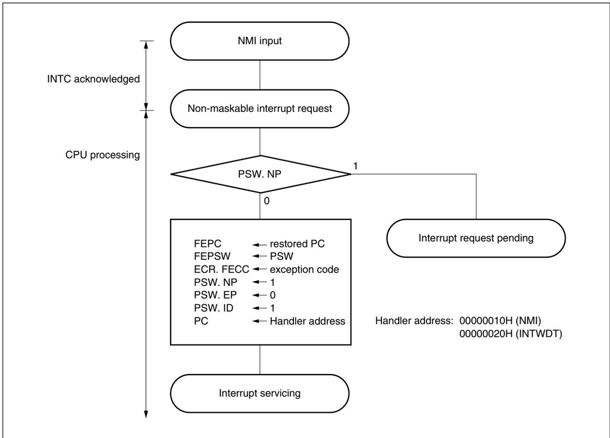
Figure 7-2. Acknowledging Non-Maskable Interrupt Requests
