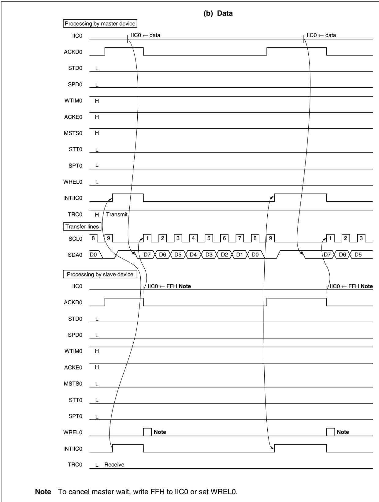
**Figure 11-22. Example of Master to Slave Communication
