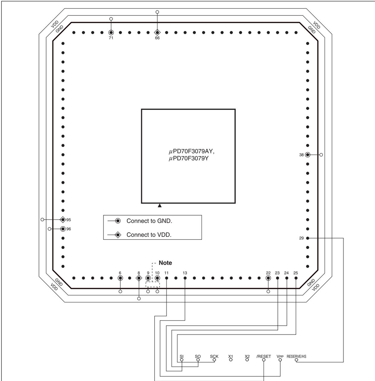
**Note** The  $\mu$ PD70F3079AY and 70F3079Y cannot be supplied with the clock from the CLK pin of the flash programmer (PG-FP3/PG-FP4). Supply the clock by creating an oscillator on the flash writing adapter (broken-line portion). An example of the oscillator is shown below.
