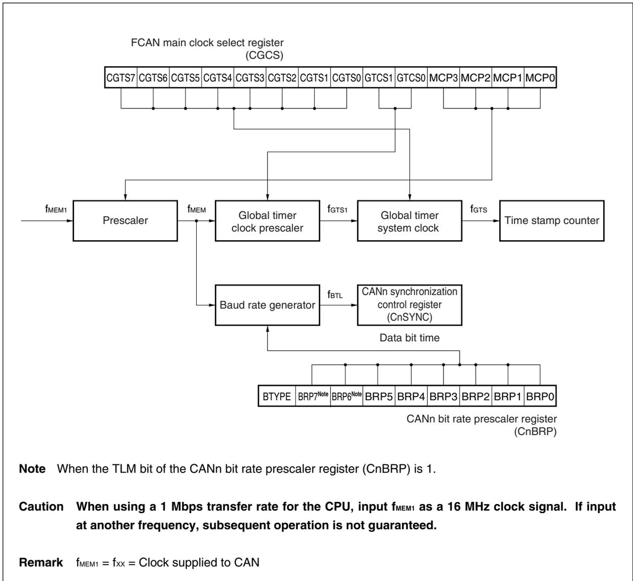
**Note** When the TLM bit of the CANn bit rate prescaler register (CnBRP) is 1.
