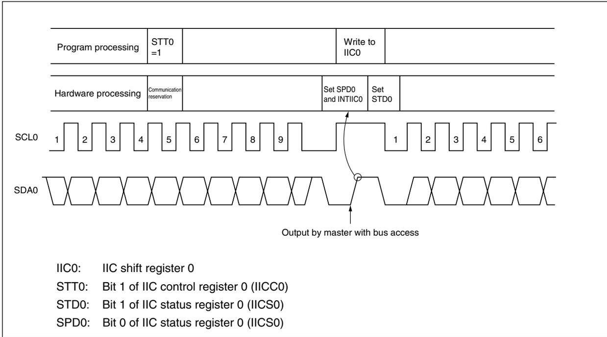
Communication reservations are accepted via the following timing. After bit 1 (STD0) of IIC status register 0 (IICS0) is set to 1, a communication reservation can be made by setting bit 1 (STT0) of IIC control register 0 (IICC0) to 1 before a stop condition is detected.
