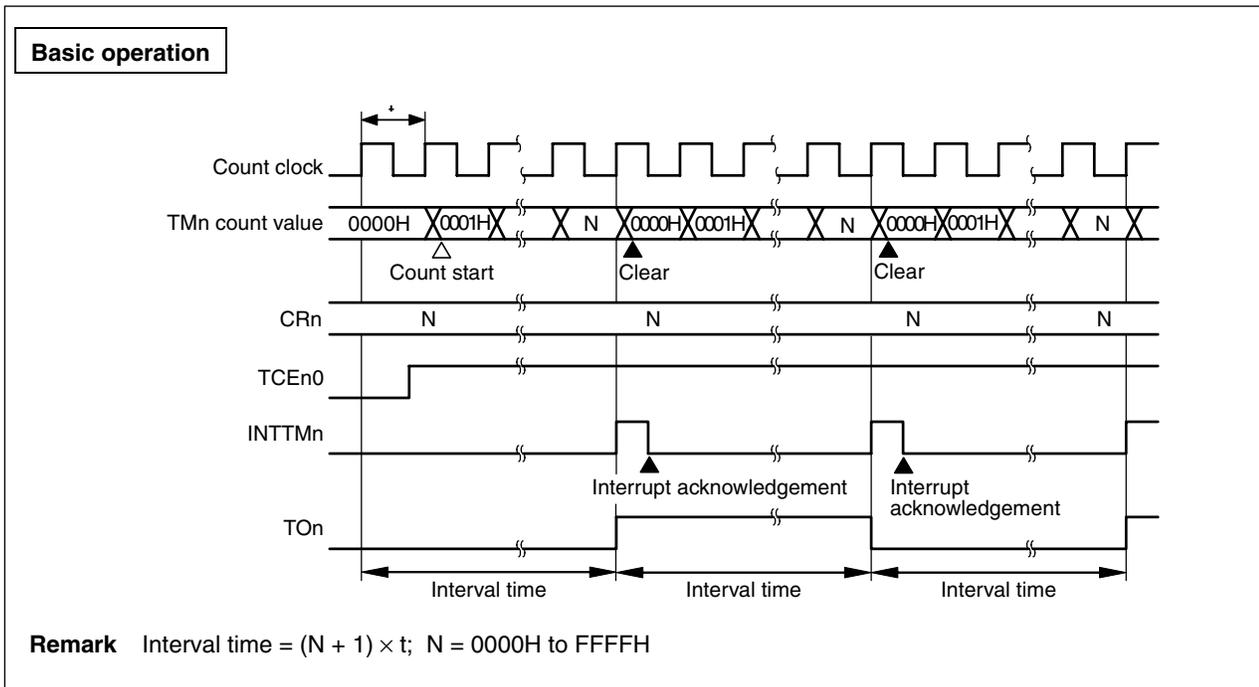
Figure 8-32. Timing of Interval Timer Operation (2/2)
