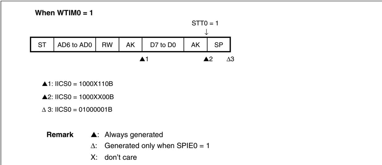
(h) When arbitration loss occurs due to low-level data when attempting to generate a stop condition
