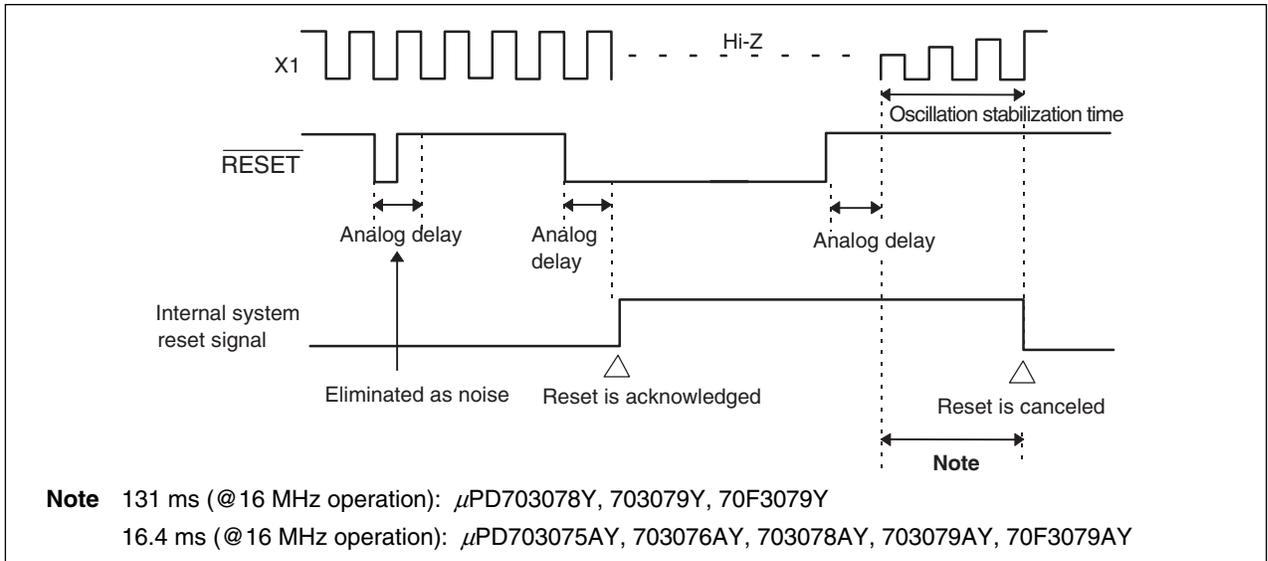
Figure 14-2. Timing of Reset by Power-on-Clear
