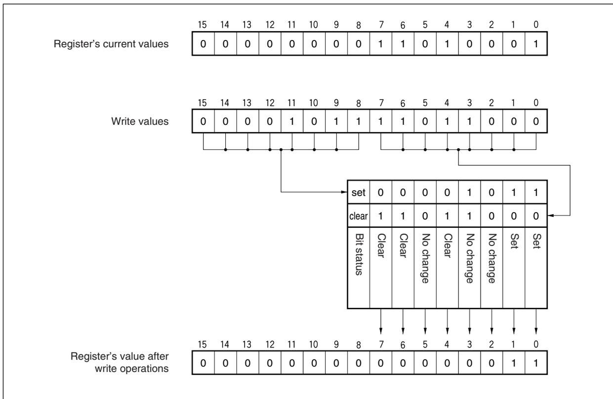
Figure 18-4. 16-Bit Data During Write Operation
