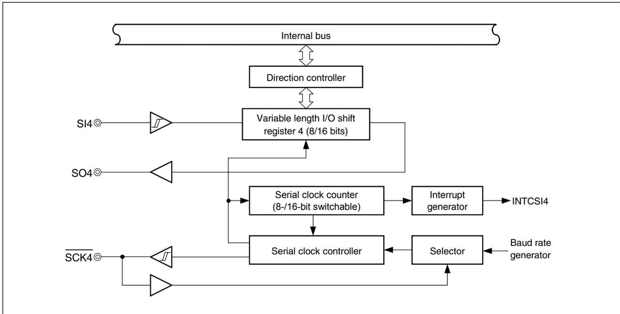
**(1) Variable-length serial I/O shift register 4 (SIO4)**
