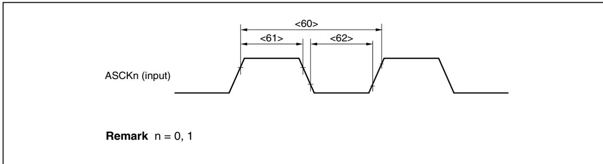
**(8) 3-wire serial interface (CSI0, CSI1, CSI3) timing**
