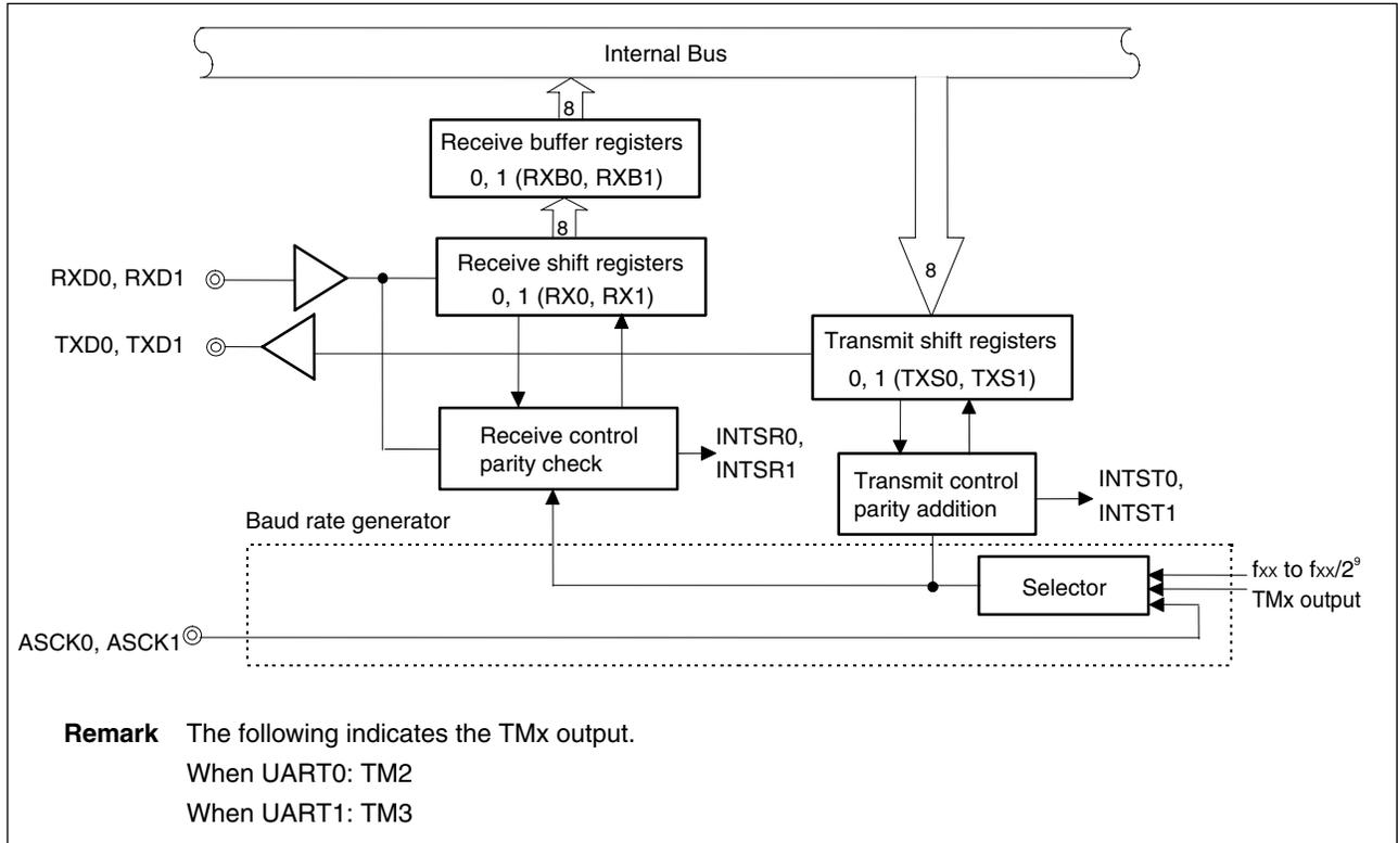
**(1) Transmit shift registers 0, 1 (TXS0, TXS1)**
