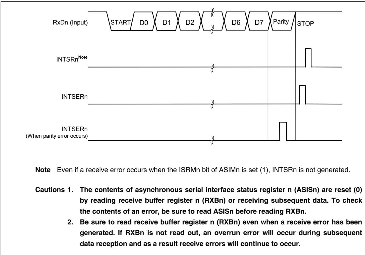
**Note** Even if a receive error occurs when the ISRMn bit of ASIMn is set (1), INTSRn is not generated.
