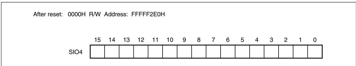
When the transfer bit length is set to other than 16 bits and data is set to the shift register, data should be aligned from the lowest bit of the shift register, regardless of whether MSB or LSB is set for the first transfer bit. Any data can be set to the unused higher bits, however, in this case the data received after a serial transfer operation becomes 0.
