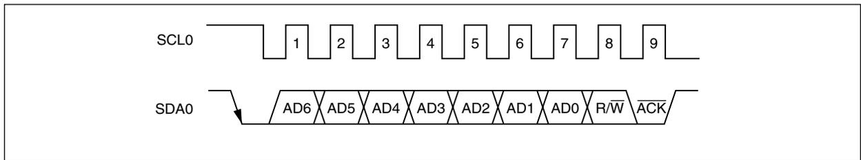
When the local address is received, an  $\overline{ACK}$  signal is automatically output in synchronization with the falling edge of the eighth clock of SCL0 regardless of the ACEK0 value. No  $\overline{ACK}$  signal is output if the received address is not a local address.
