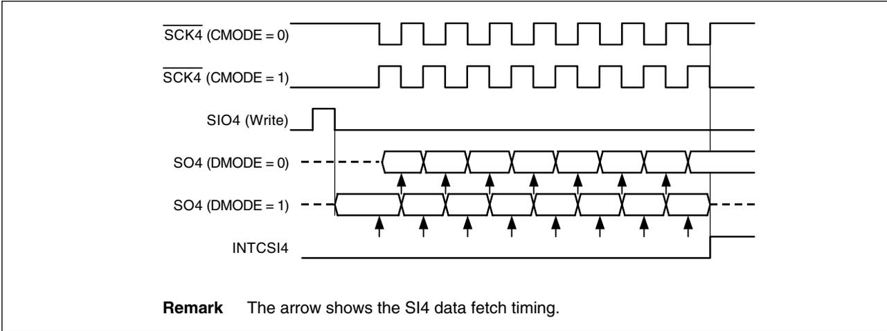
When CMODE = 0, the serial clock ( $\overline{SCK4}$ ) stops at a high level while the operation is stopped, and outputs a low level during a data transfer operation. When CMODE = 1, on the other hand,  $\overline{SCK4}$  stops at a low level while the operation is stopped and outputs a high level during a data transfer operation.
