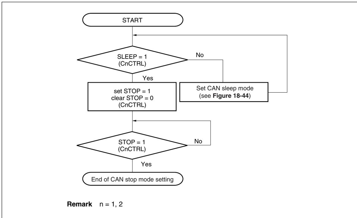
Figure 18-48. Clearing of CAN Stop Mode
