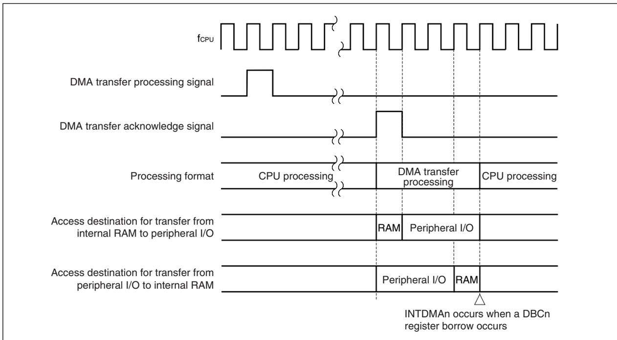
If two or more DMA transfer requests are generated simultaneously, the DMA transfer requests are executed in the following priority order: DMA0 > DMA1 > DMA2 > DMA3 > DMA4 > DMA5. While a higher priority DMA transfer request is being executed, the lower priority DMA transfer requests are held pending. After the higher priority DMA transfer ends, control always shifts to the CPU processing once, and then the lower priority DMA transfer is executed.
