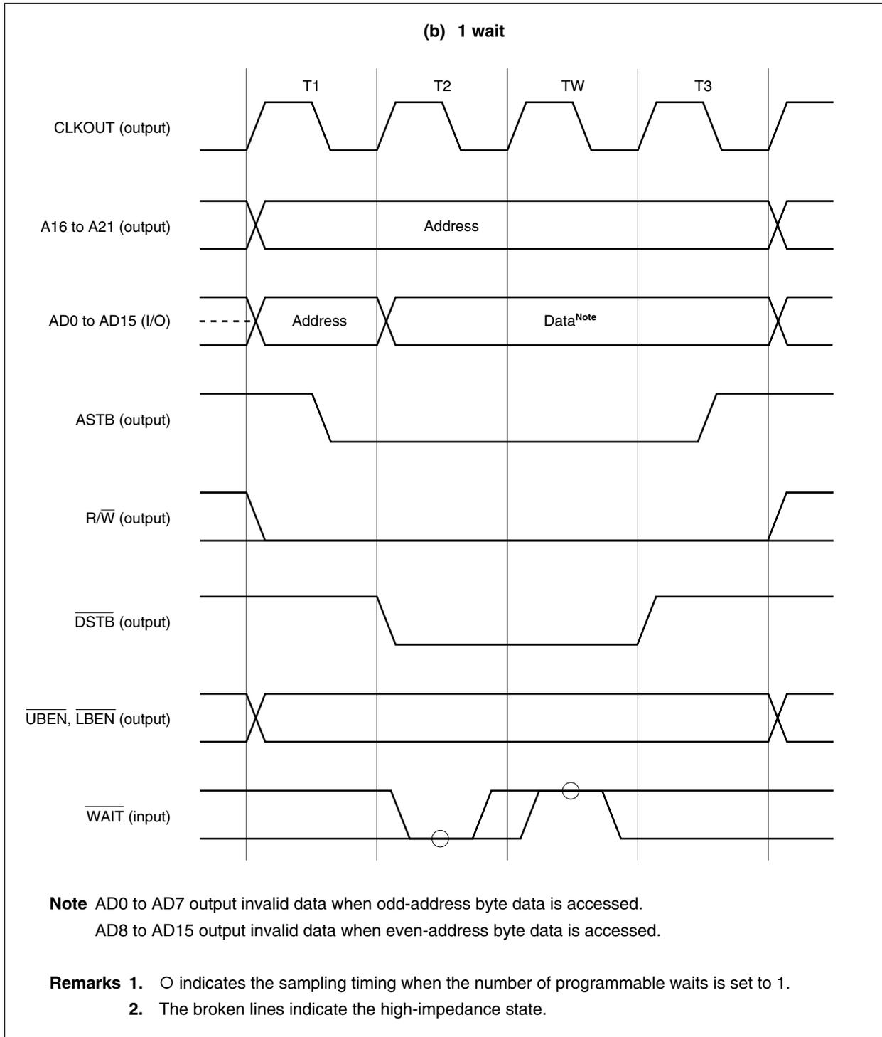
Figure 6-10. Bus Hold Timing
