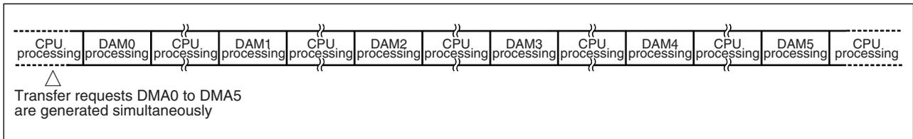
DMA operation stops only in the IDLE/STOP mode. In the HALT mode, DMA operation continues. DMA also operates during the bus hold period and after access to the external memory.
