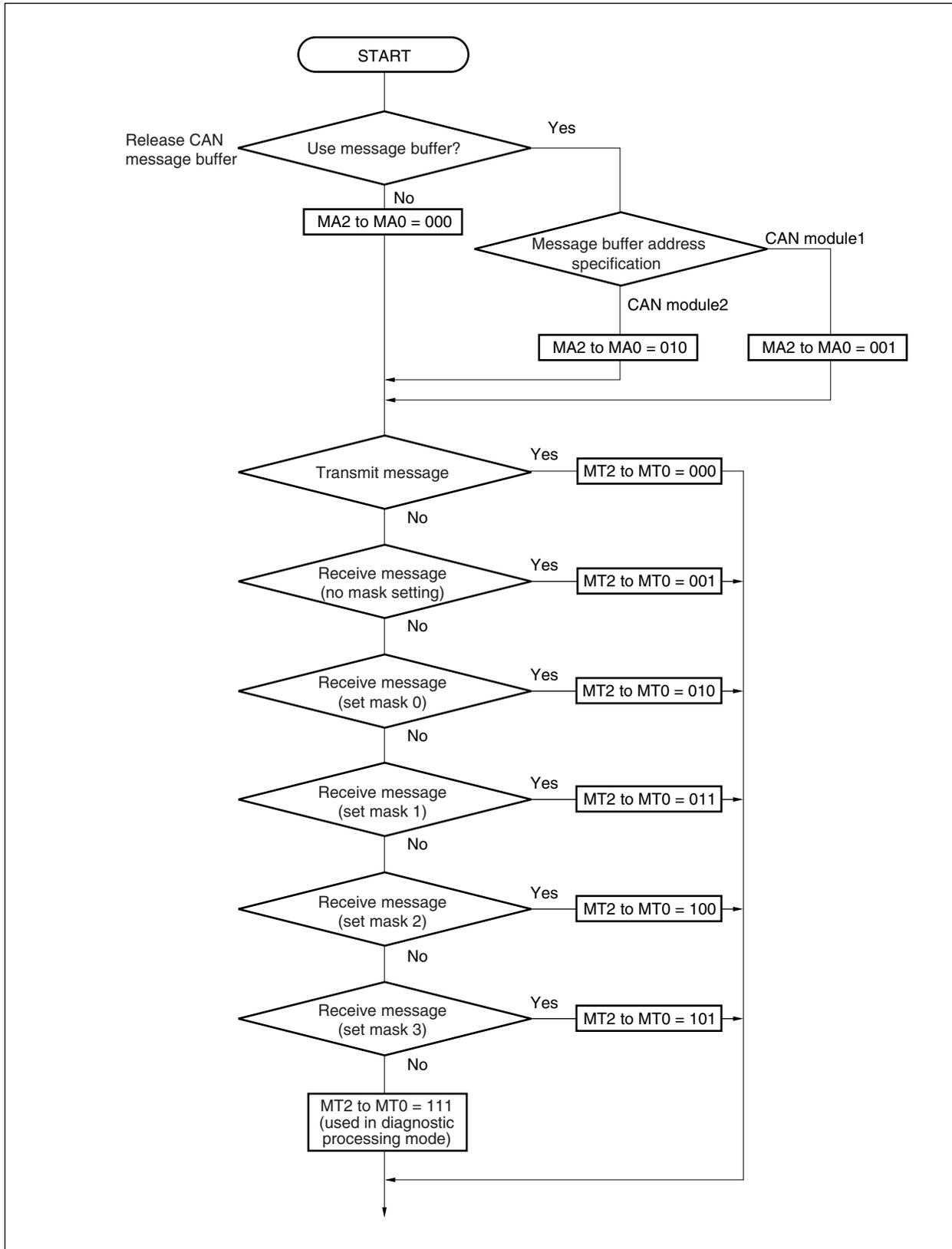
Figure 18-39. Setting of CAN Message Control Registers 00 to 31 (M\_CTRL00 to M\_CTRL31)
