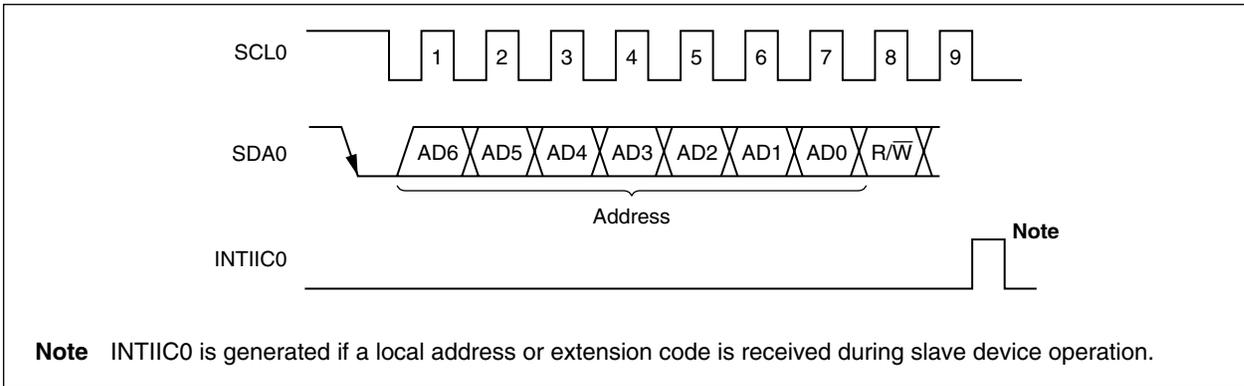
**Note** INTIIC0 is generated if a local address or extension code is received during slave device operation.
