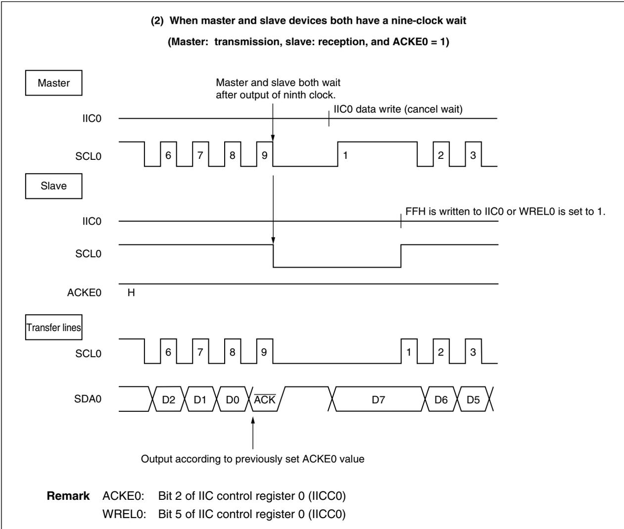
A wait may be automatically generated depending on the setting of bit 3 (WTIM0) of IIC control register 0 (IICC0). Normally, when bit 5 (WREL0) of IICC0 is set to 1 or when FFH is written to IIC shift register 0 (IIC0), the wait status is canceled and the transmitting side writes data to IIC0 to cancel the wait status. The master device can also cancel the wait status via either of the following methods.
