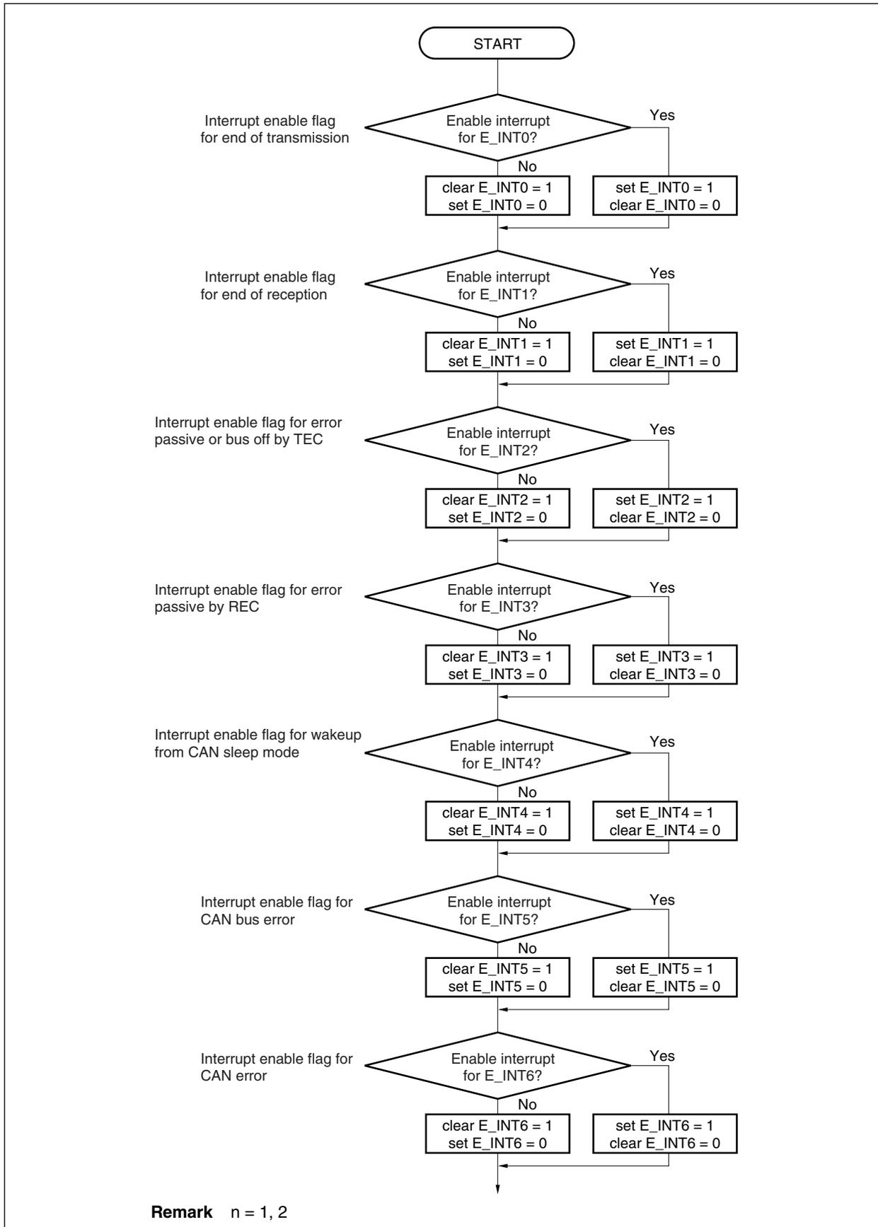
Figure 18-34. Setting of CANn Definition Register (CnDEF)
