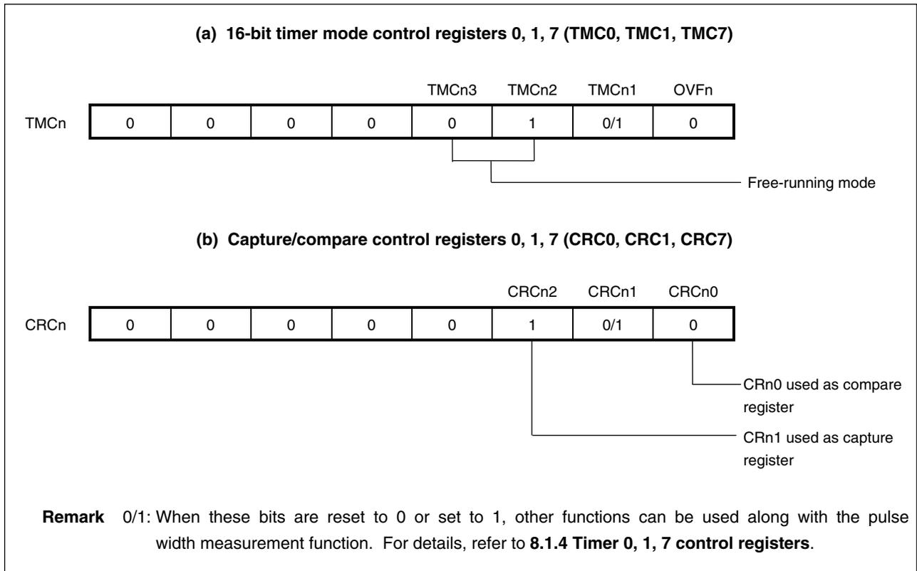
Figure 8-9. Configuration for Pulse Width Measurement with Free-Running Counter
