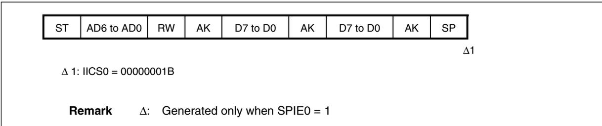
(5) Arbitration loss operation (operation as slave after arbitration loss)
