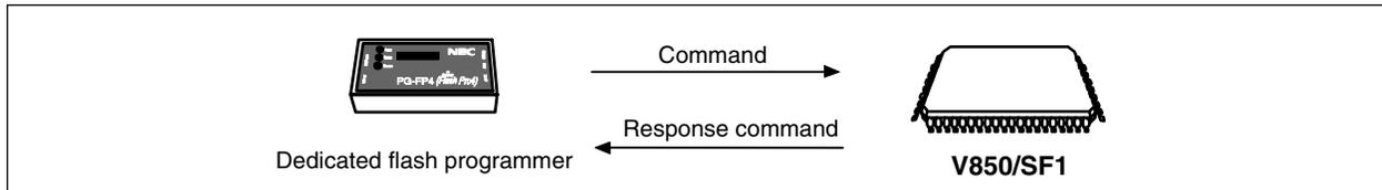
The following shows the commands for flash memory control of the V850/SF1. All of these commands are issued from the dedicated flash programmer, and the V850/SF1 performs the various processing corresponding to the commands.
