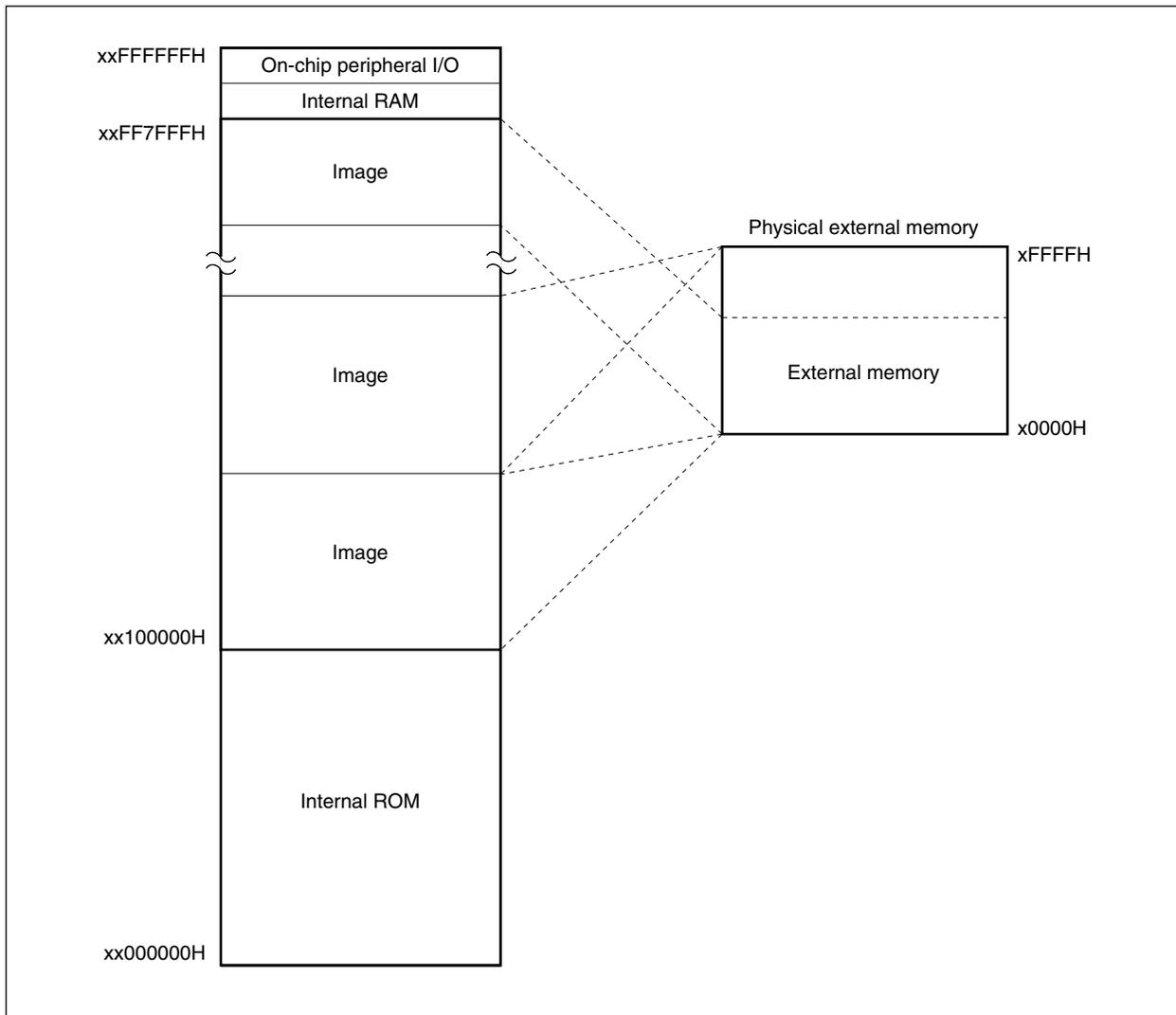
Figure 3-13. External Memory Area (When Expanded to 4 MB)
