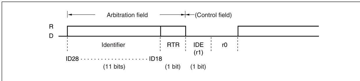
Figure 18-15. Arbitration Field (in Extended Format Mode)
