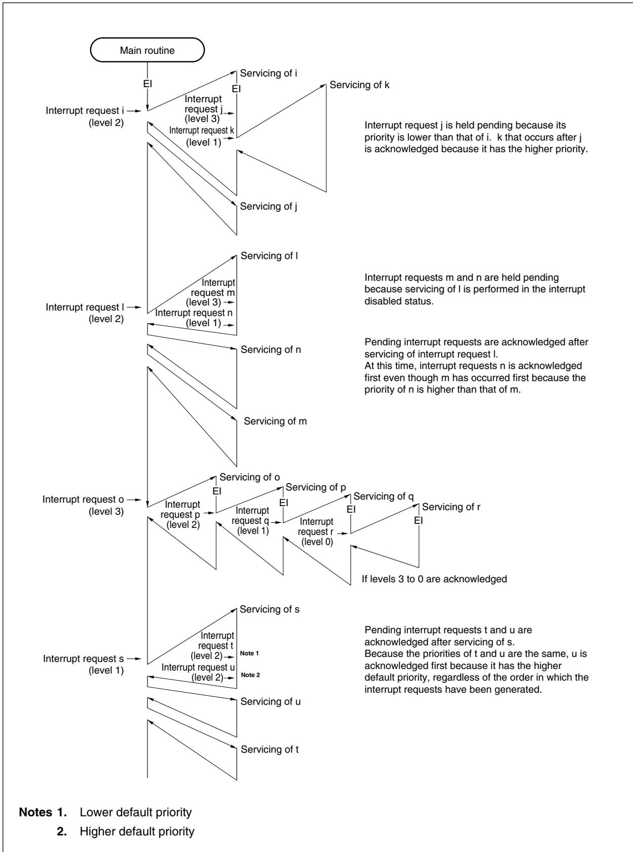
Figure 7-8. Example of Servicing Interrupt Requests Simultaneously Generated
