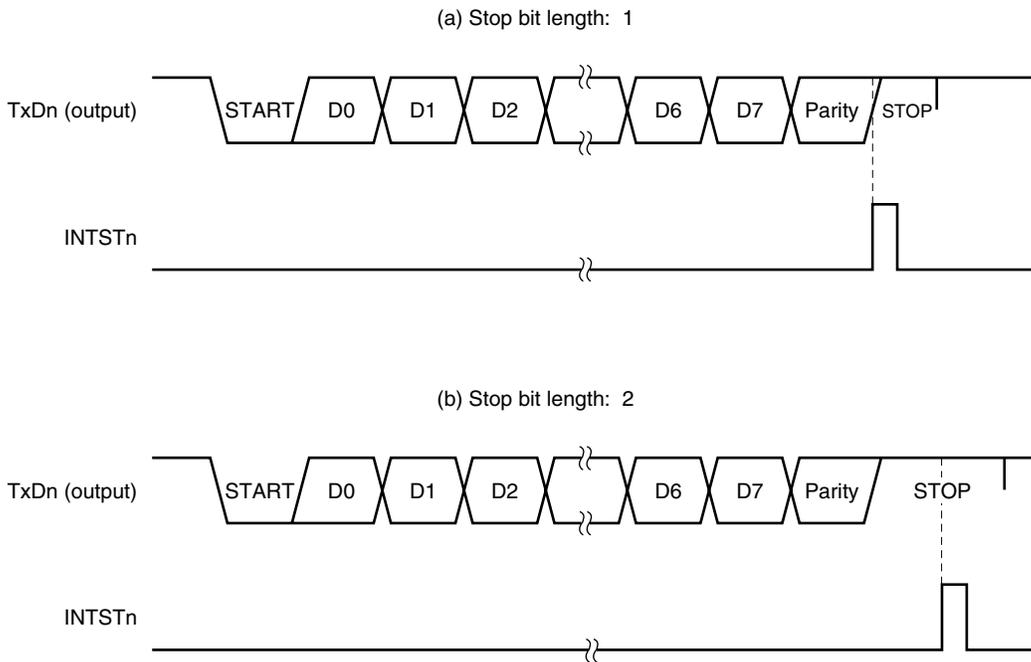
**Caution** Do not write to asynchronous serial interface mode register n (ASIMn) during a transmit operation. Writing to ASIMn during a transmit operation may disable further transmit operations (in such cases, enter a RESET to restore normal operation).
