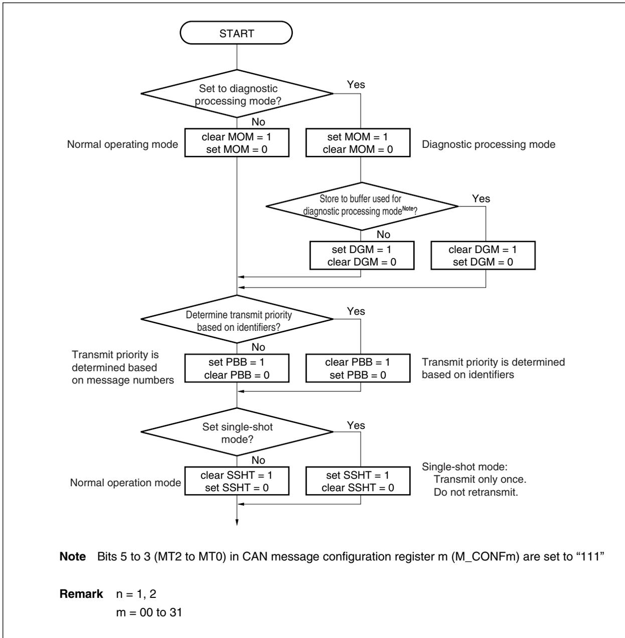
Figure 18-35. Setting of CANn Control Register (CnCTRL) (1/2)
