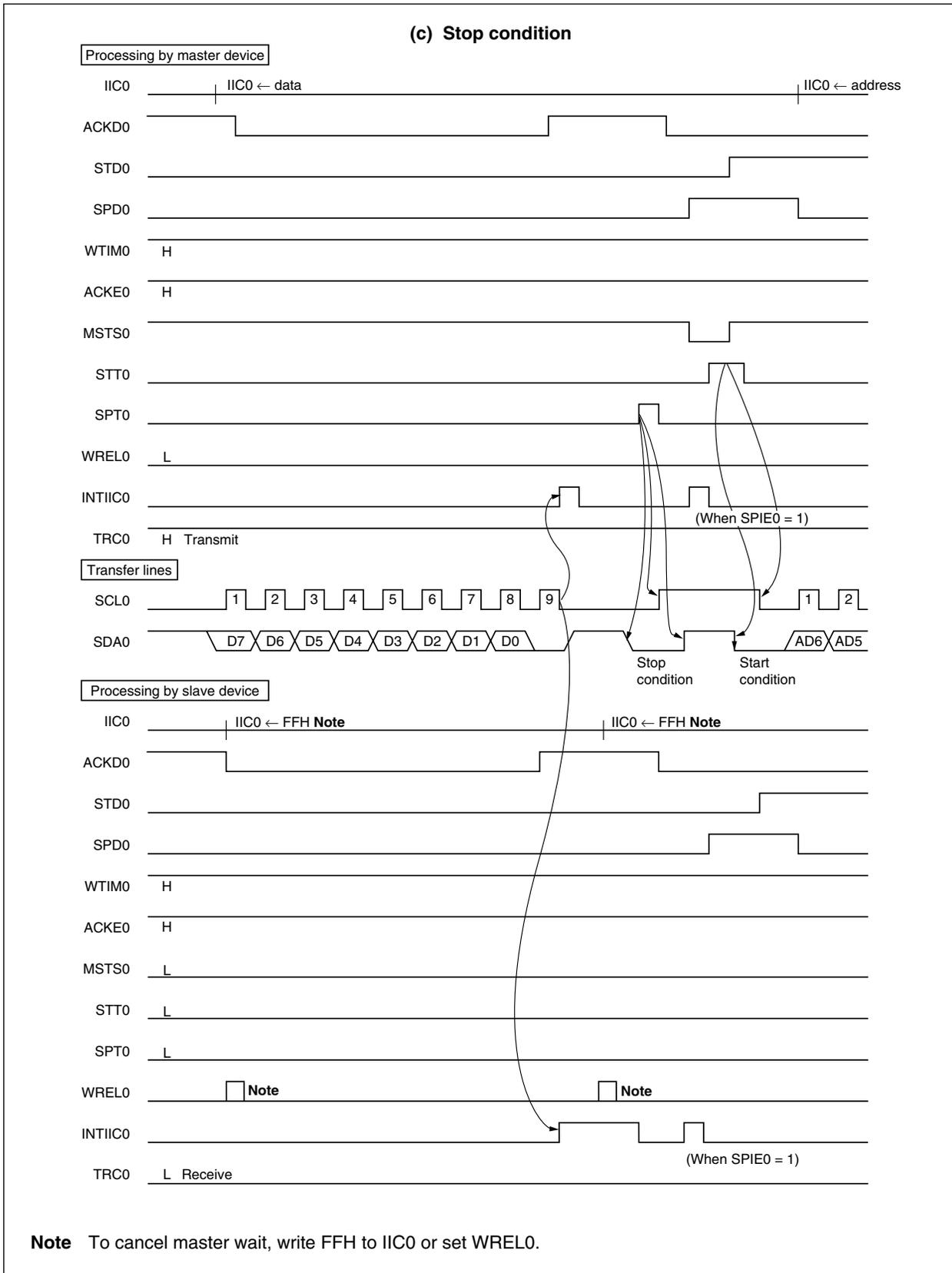
**Figure 11-23. Example of Slave to Master Communication
