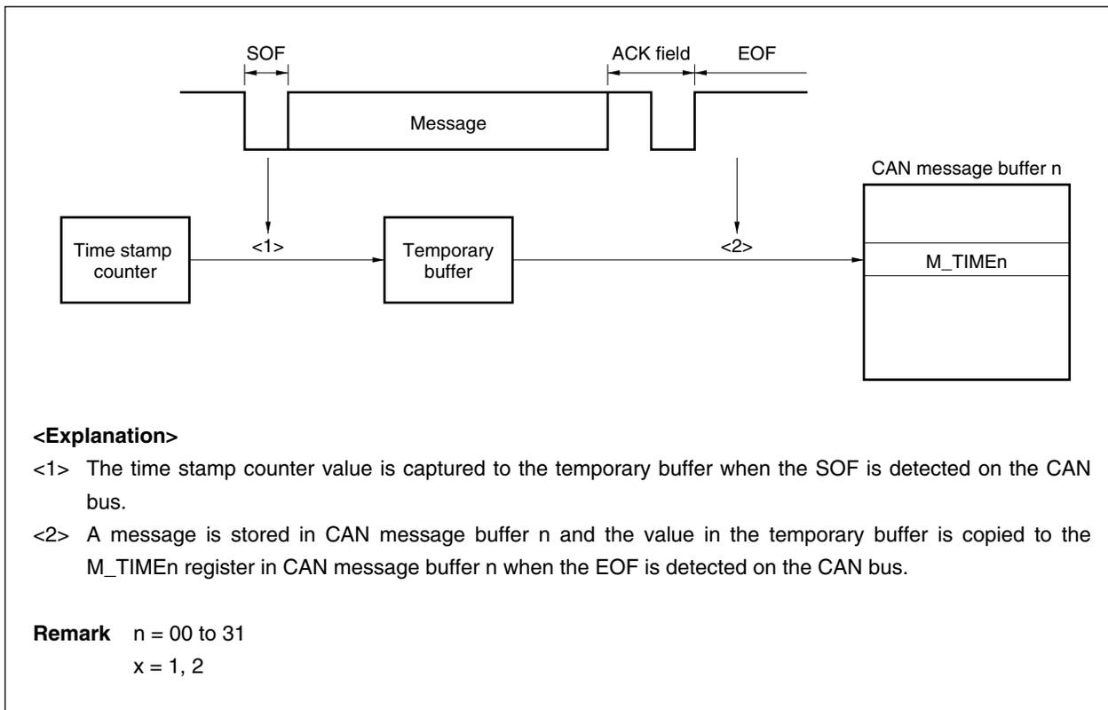
Figure 18-6. Time Stamp Function Setting for Message Reception (When CxCTRL Register's TMR Bit = 1)
