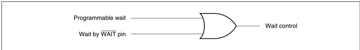
For example, if the number of programmable waits and the timing of the  $\overline{\text{WAIT}}$  pin input signal are as illustrated below, three wait states will be inserted in the bus cycle.
