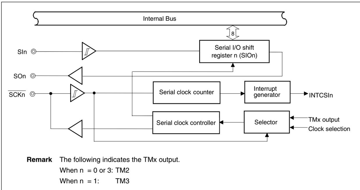
(1) Serial I/O shift register n (SIO<sub>n</sub>)
