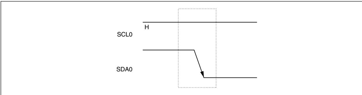
A start condition is output when bit 1 (STT0) of IIC control register 0 (IICC0) is set to 1 after a stop condition has been detected (SPD0: Bit 0 = 1 in IIC status register 0 (IICS0)). When a start condition is detected, bit 1 (STD0) of IICS0 is set to 1.
