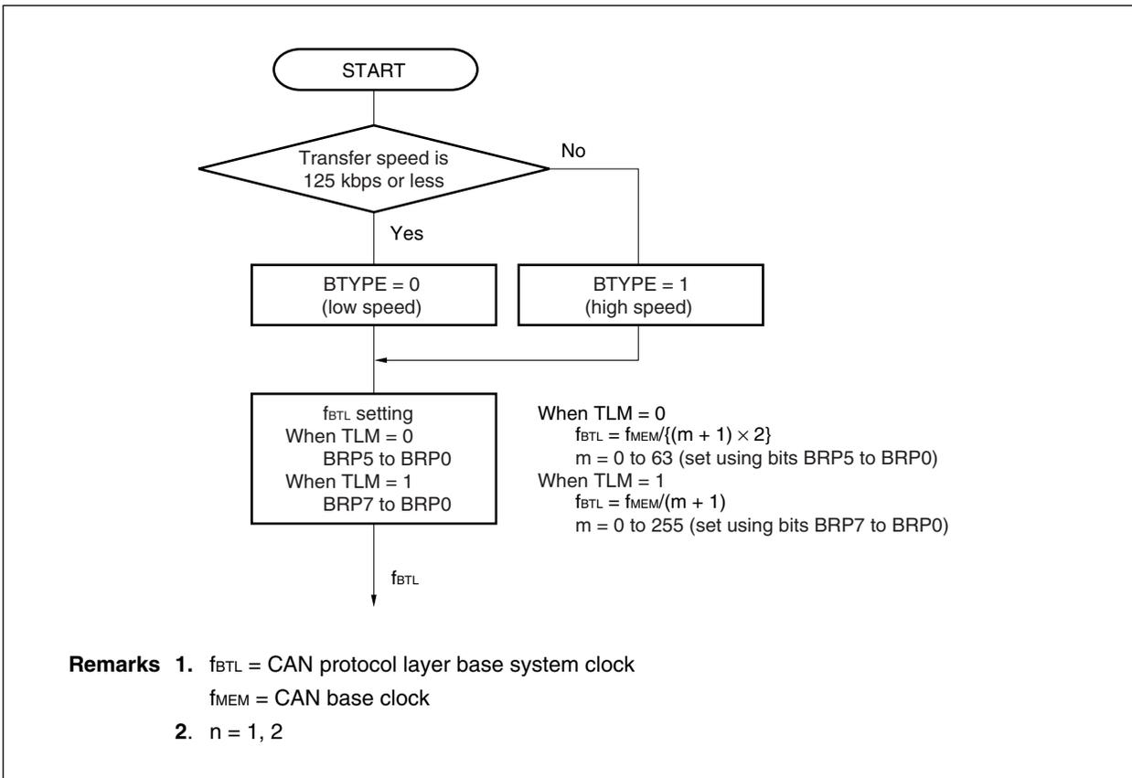
Figure 18-32. Setting of CANn Synchronization Control Register (CnSYNC)
