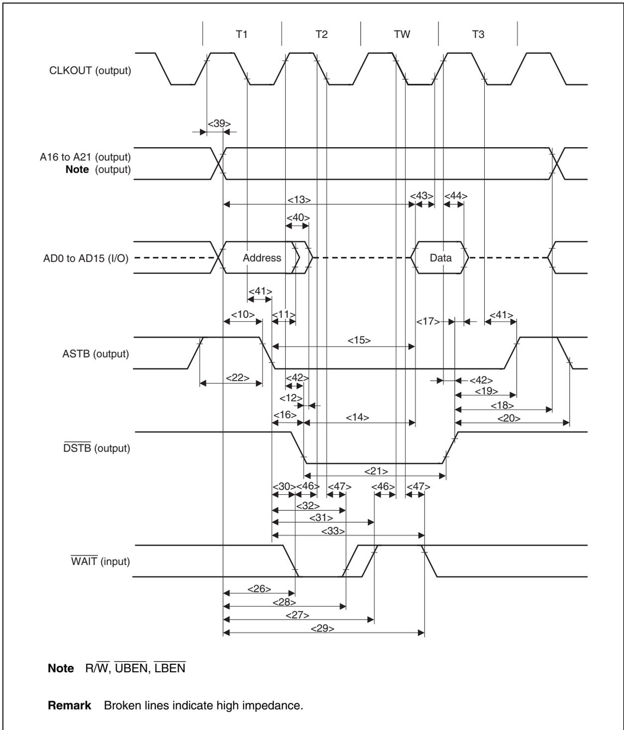
(h) Write cycle (CLKOUT synchronous/asynchronous, 1 wait)
