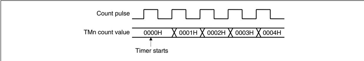
(2) 16-bit capture/compare register setting (in the clear & start mode entered on match between TMn and CRn0)
