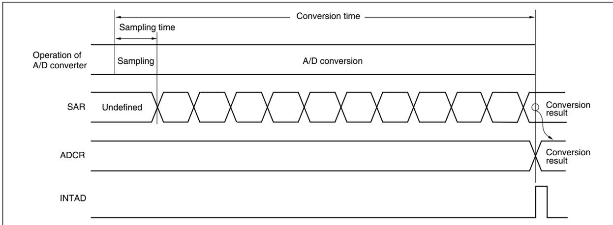
A/D conversion is successively executed until bit 7 (ADCS) of A/D converter mode register 1 (ADM1) is reset to 0 by software.
