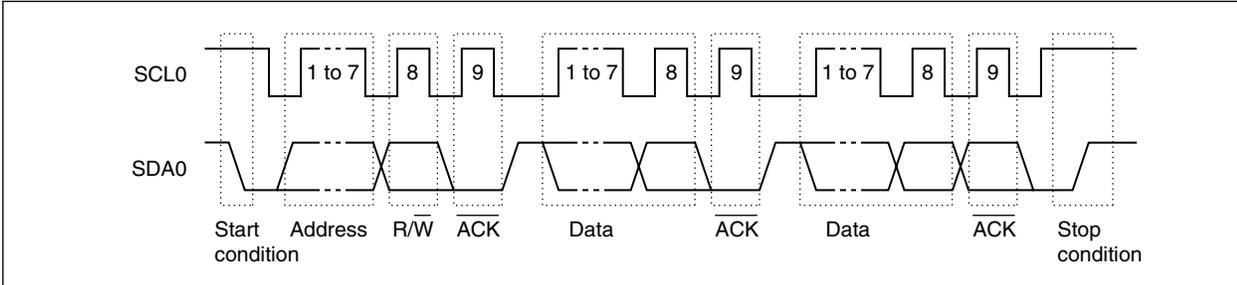
The master device outputs the start condition, slave address, and stop condition.
