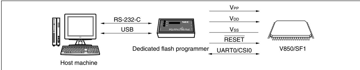
A host machine is required for controlling the dedicated flash programmer.
