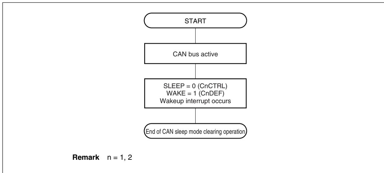
Figure 18-46. Clearing of CAN Sleep Mode by CPU
