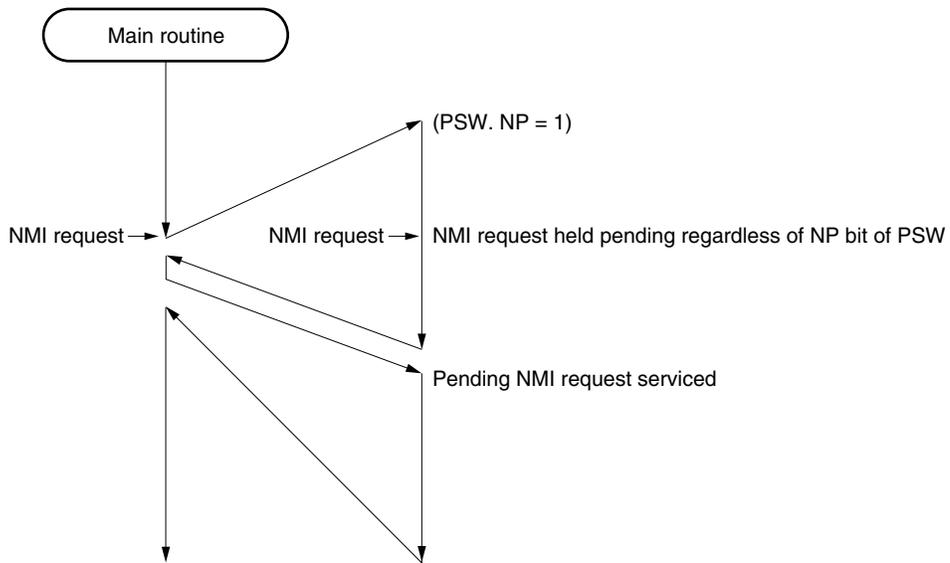
(b) If a new NMI request is generated twice while an NMI service routine is being executed
