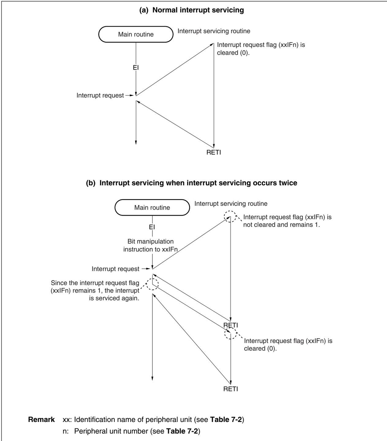
Figure 13-6. When Interrupt Servicing Occurs Twice During DMA Operation (2/2)
