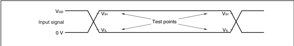
**AC Test Output Test Points** ( $V_{\text{DD}}$ :  $V_{\text{DD0}}$ ,  $\text{PORTV}_{\text{DD}}$ )
