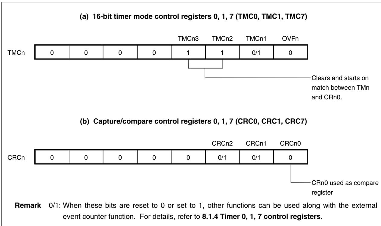
Figure 8-19. Configuration of External Event Counter
