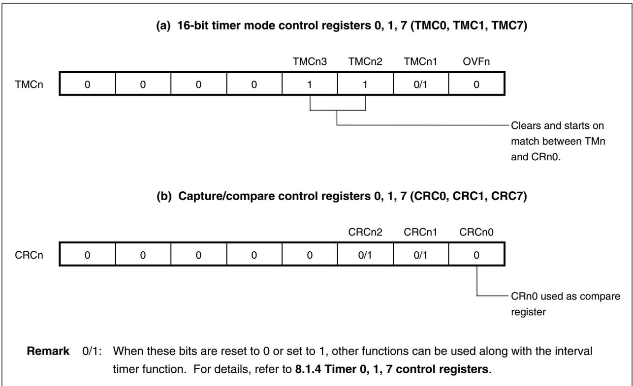
Figure 8-3. Configuration of Interval Timer
