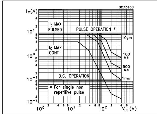
Figure 2. Derating Curve
