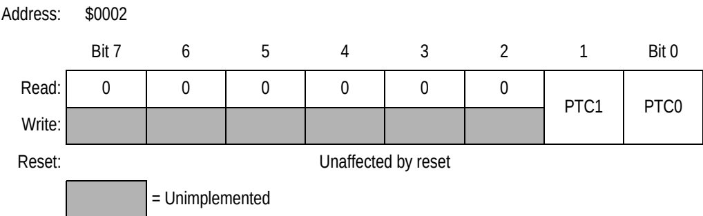
Figure 16-9. Port C Data Register (PTC)
