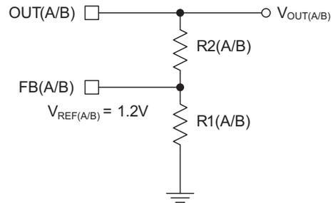
To select appropriate resistor values, first choose R1 such that the feedback network bias current is less than 10µA. Then, according to the desired  $V_{OUT}$ , calculate R2 according to the equation below. An example calculation follows.
