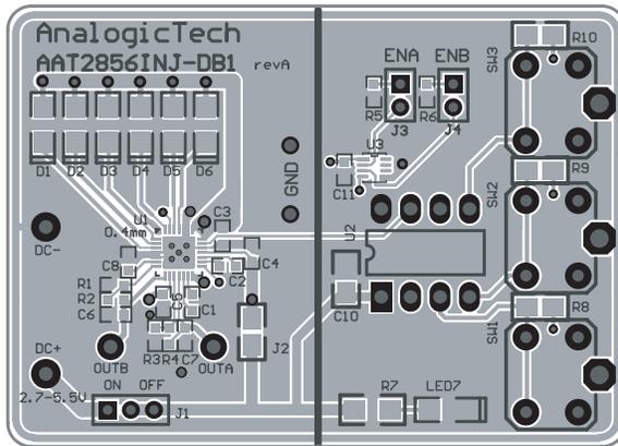
**Figure 7: AAT2856 Evaluation Board Layout Top Side.**
