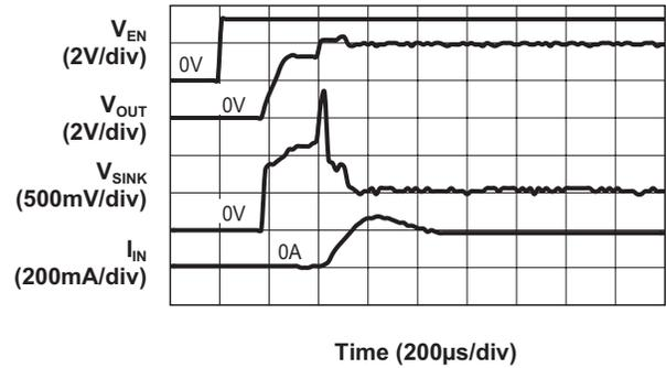
**Turn On to 2X Mode Backlight (30mA/ch; Data 1; V<sub>IN</sub> = 2.7V)**
