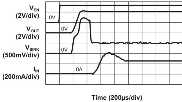
**Turn On to 1.5X Mode Backlight (30mA/ch; Data 1; V<sub>IN</sub> = 3.4V)**
