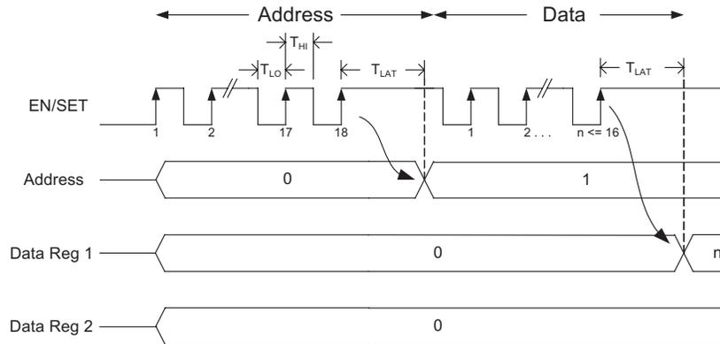
**Figure 1: AS<sup>2</sup>Cwire Serial Interface Timing.**
