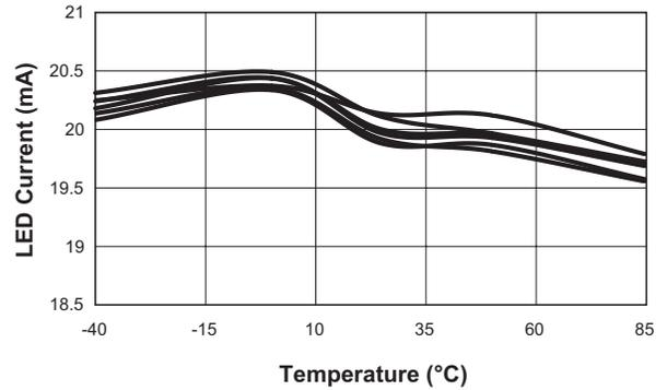
**Turn On to 1X Mode Backlight (30mA/ch; Data 1; V<sub>IN</sub> = 4.2V)**
