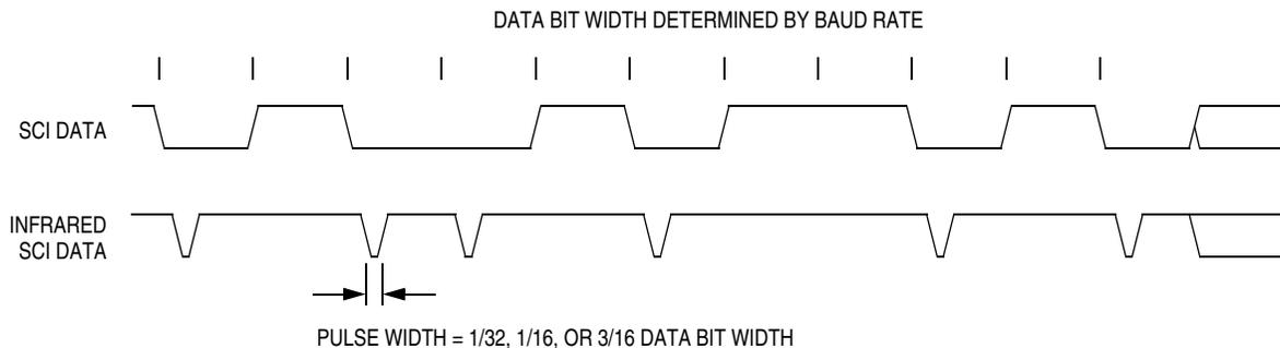
**Figure 14-4. Infrared SCI Data Example**
