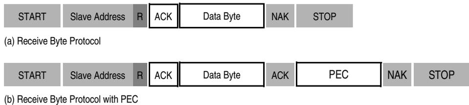
Figure 16-15. Receive Byte
