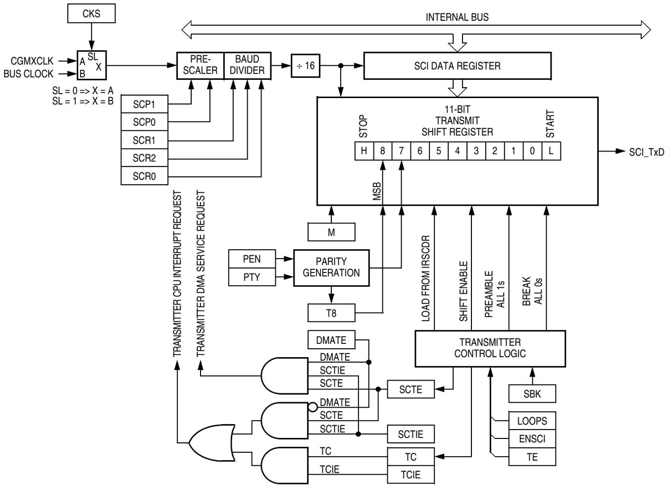
Figure 14-7. SCI Transmitter
