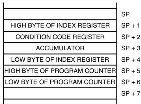
**Figure 10-7. Stack Pointer at Monitor Mode Entry**
