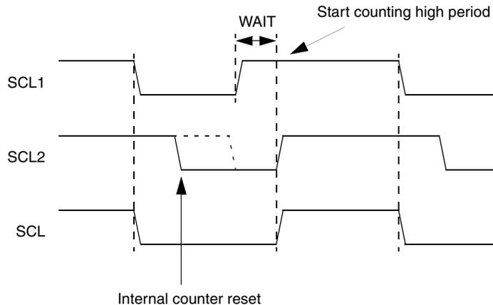
**Figure 16-3. Clock Synchronization**
