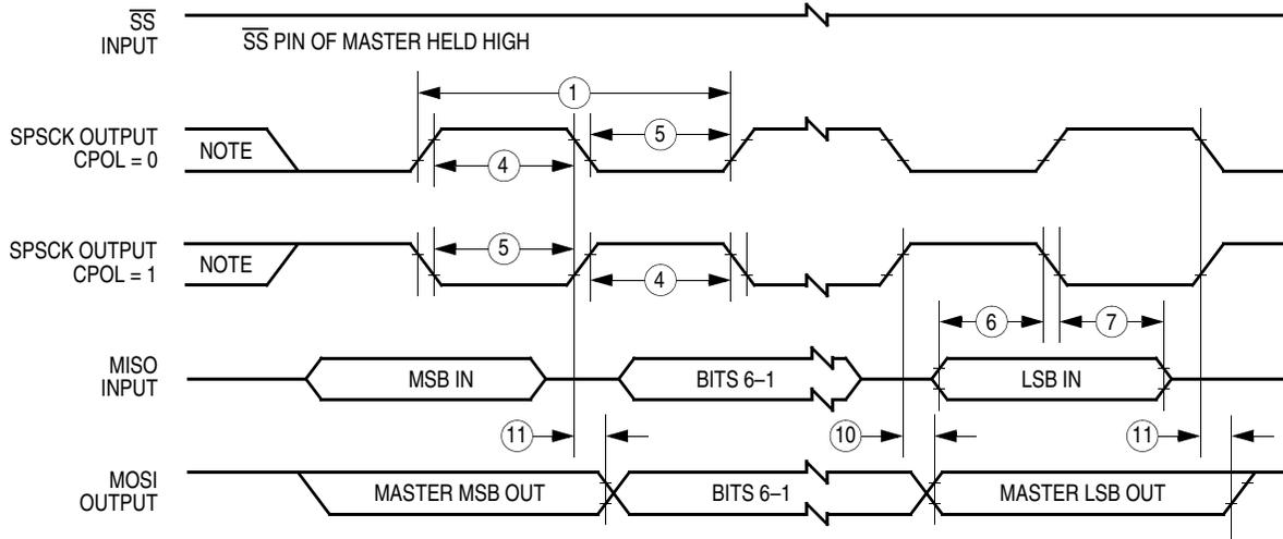
Note: This first clock edge is generated internally, but is not seen at the SPSCCK pin.
