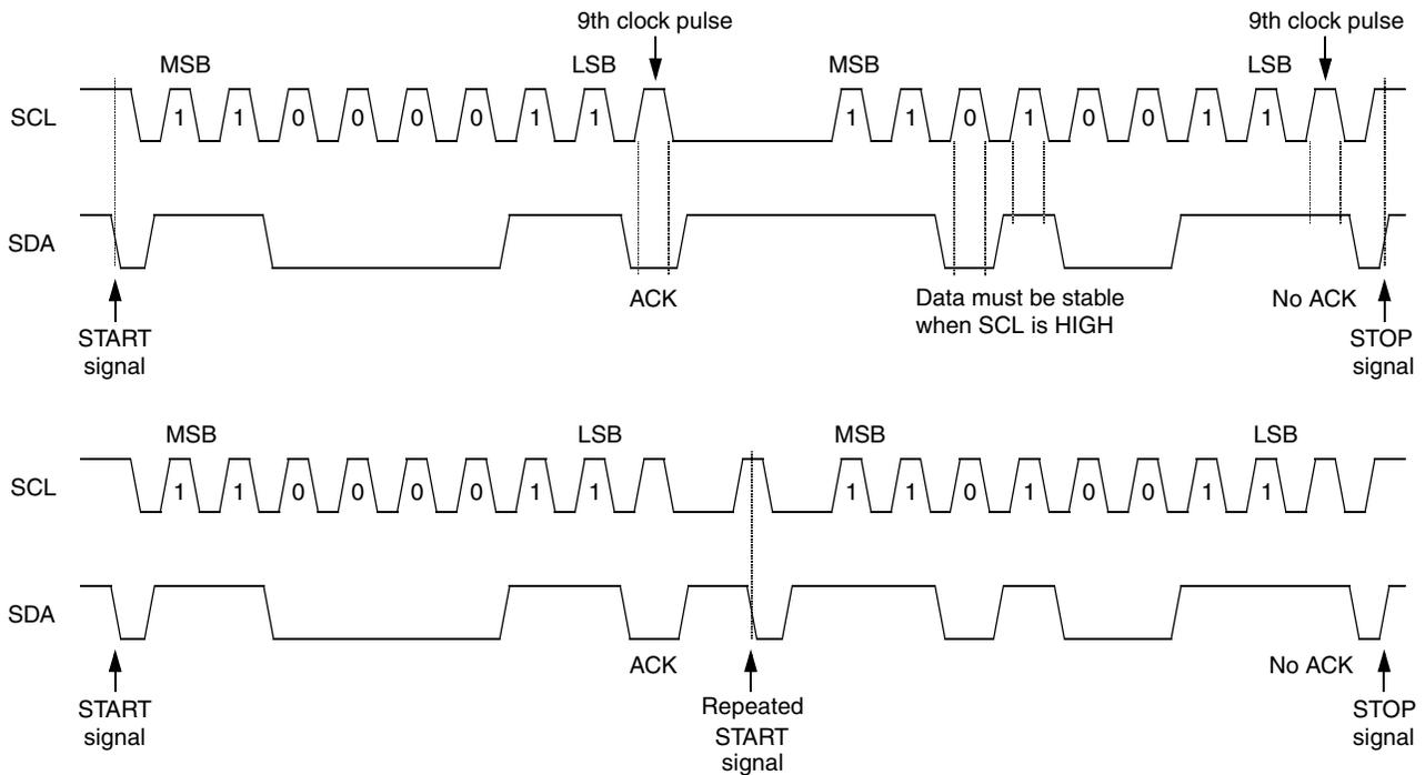
**Figure 16-2. Multi-Master IIC Bus Transmission Signal Diagram**
