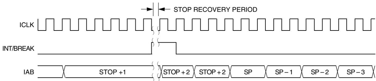
**Figure 9-19. Stop Mode Recovery from Interrupt or Break**
