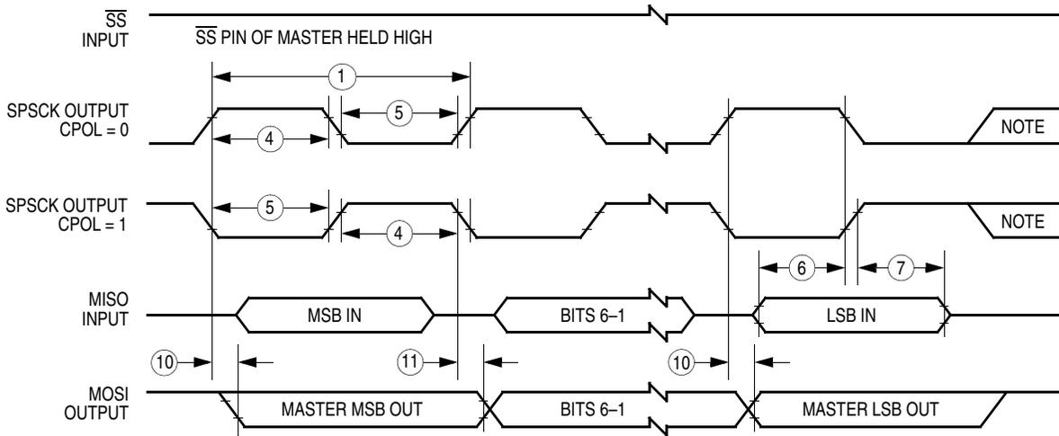
Note: This last clock edge is generated internally, but is not seen at the SPSCCK pin.
