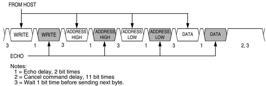
Figure 10-6. Write Transaction
