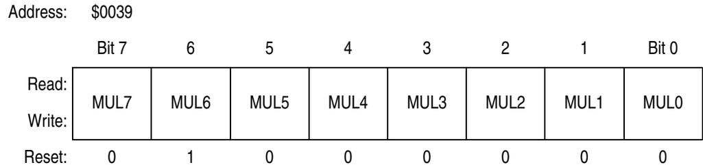
**Figure 8-7. PLL Multiplier Select Register Low (PMSL)**
