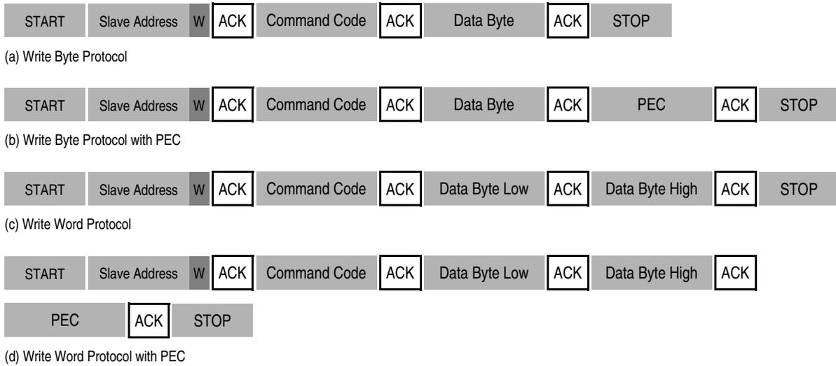
**Figure 16-16. Write Byte/Word**
