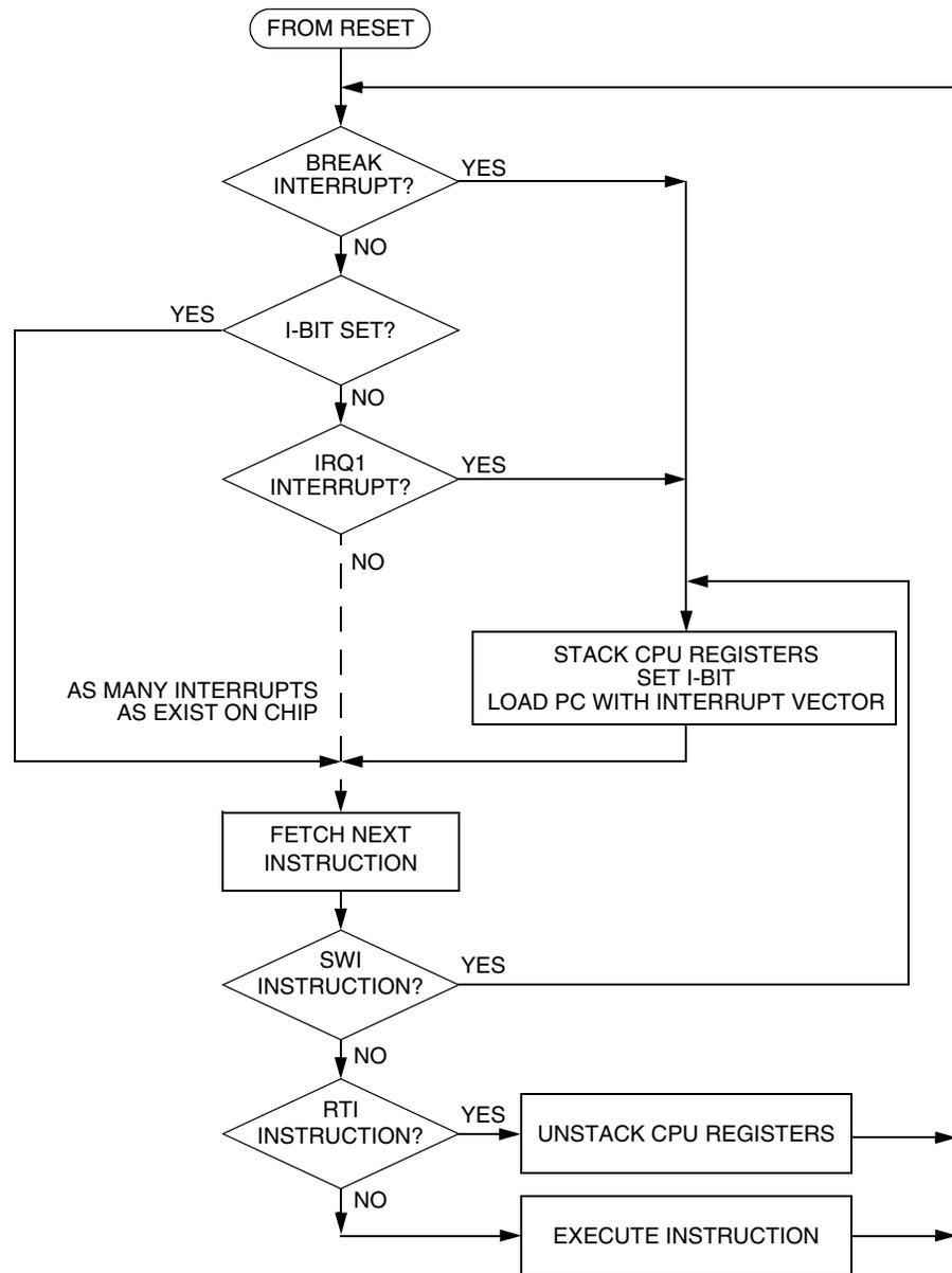
Figure 9-10. Interrupt Processing
