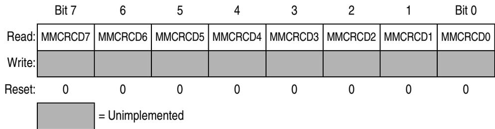
**Figure 16-10. MMIIC CRC Data Register (MMCRCDR)**
