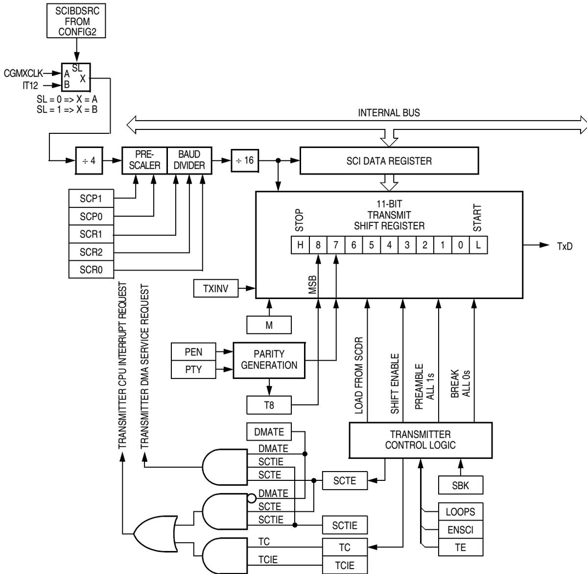
Figure 13-4. SCI Transmitter
