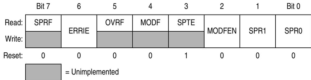
Figure 15-14. SPI Status and Control Register (SPSCR)
