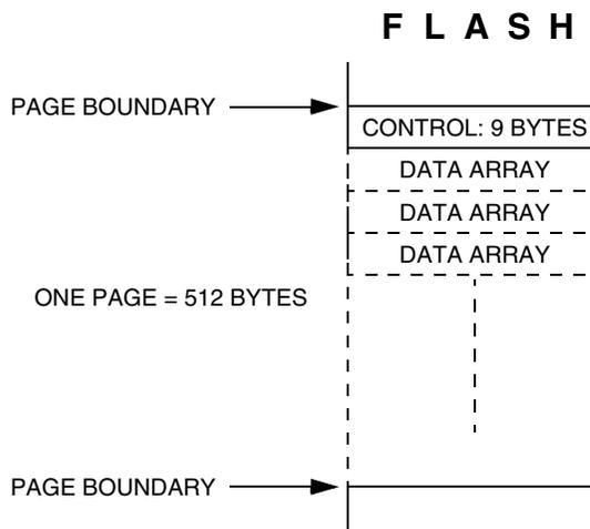
**Figure 10-10. EE\_WRITE FLASH Memory Usage**
