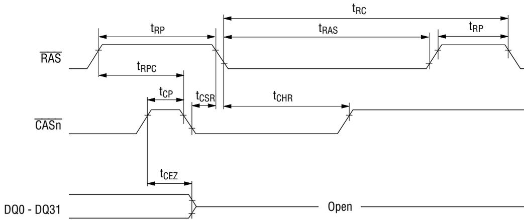
**Note:**  $\overline{\text{WE}}$ ,  $\overline{\text{OE}}$ , A0 - A8 = "H" or "L"
