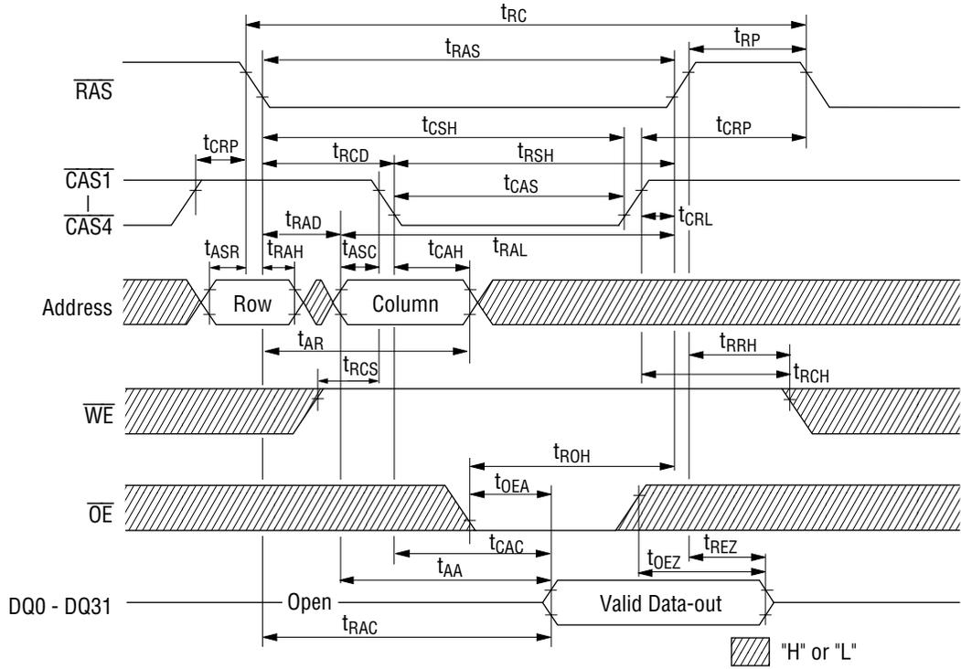
Read Cycle (Outputs Controlled by  $\overline{\text{CAS}}$ )
