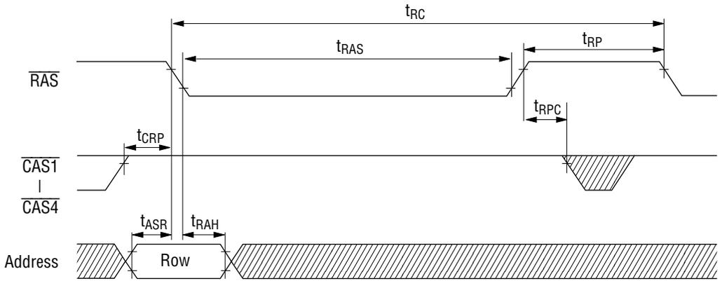
**Note:** DQs are open,  $\overline{\text{WE}}$ ,  $\overline{\text{OE}}$  = "H" or "L"
