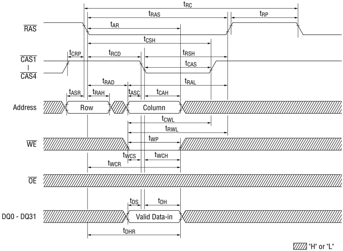
**Write Cycle ( $\overline{OE}$  Control Write)**
