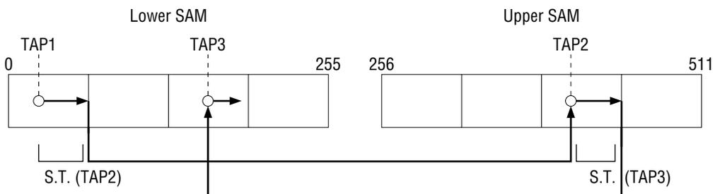
**Figure 2. Example of Boundary Split Register**
