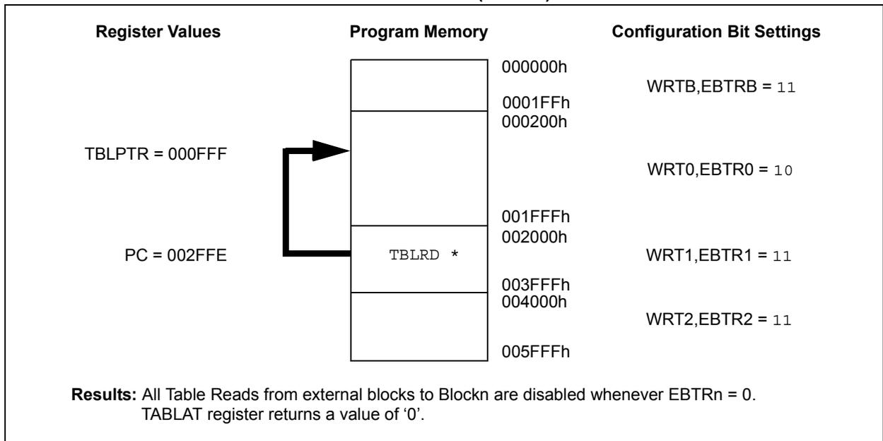
**FIGURE 20-6: EXTERNAL BLOCK TABLE READ (EBTRn) ALLOWED**
