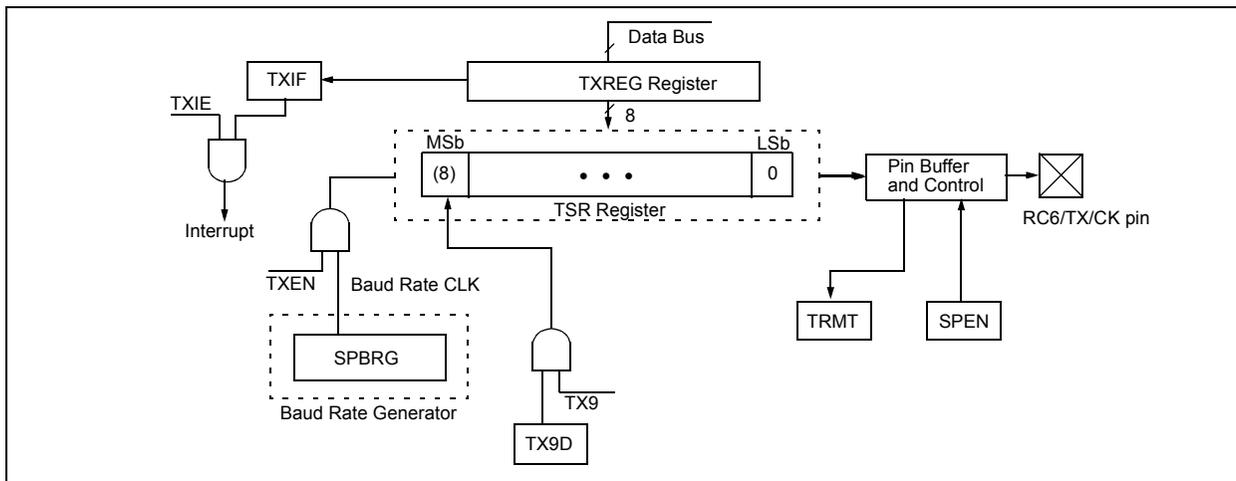
**FIGURE 17-2: ASYNCHRONOUS TRANSMISSION**
