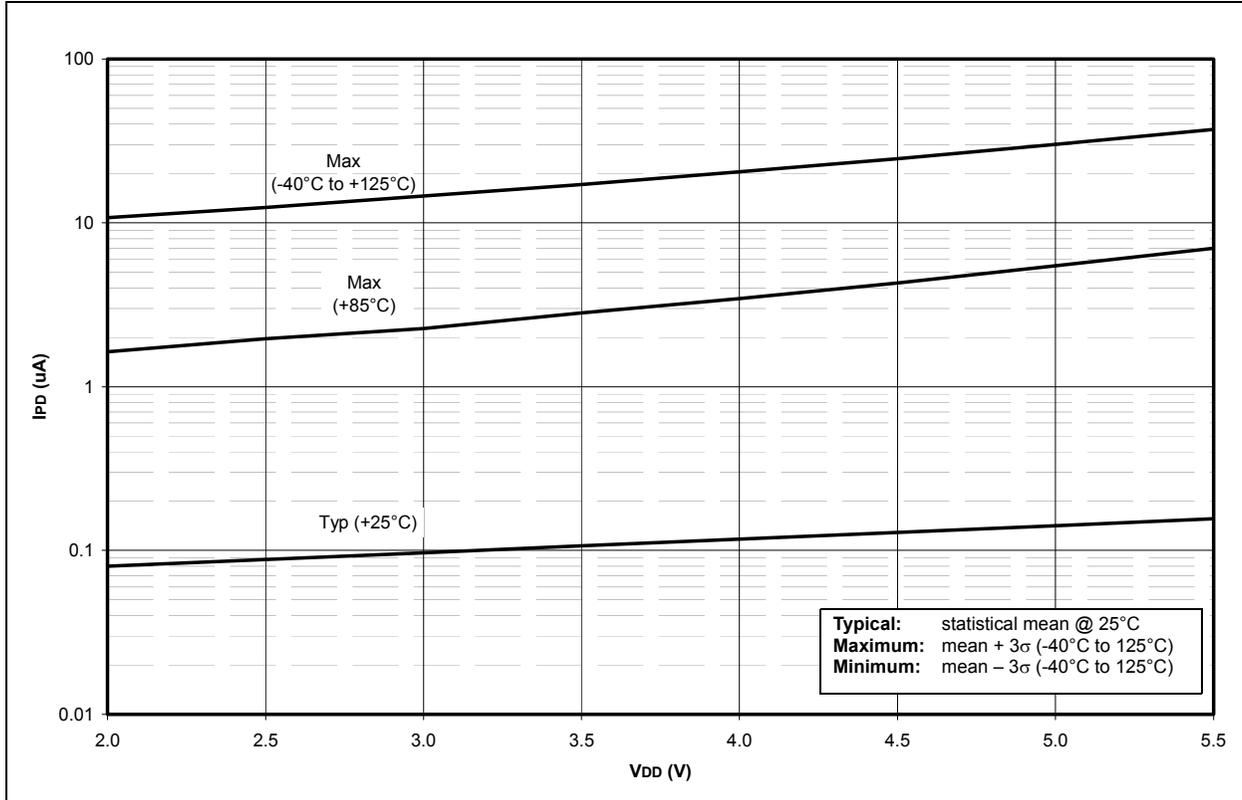
**FIGURE 24-8: ΔI<sub>BOR</sub> vs. V<sub>DD</sub> OVER TEMPERATURE (BOR ENABLED, V<sub>BOR</sub> = 2.00 - 2.16V)**
