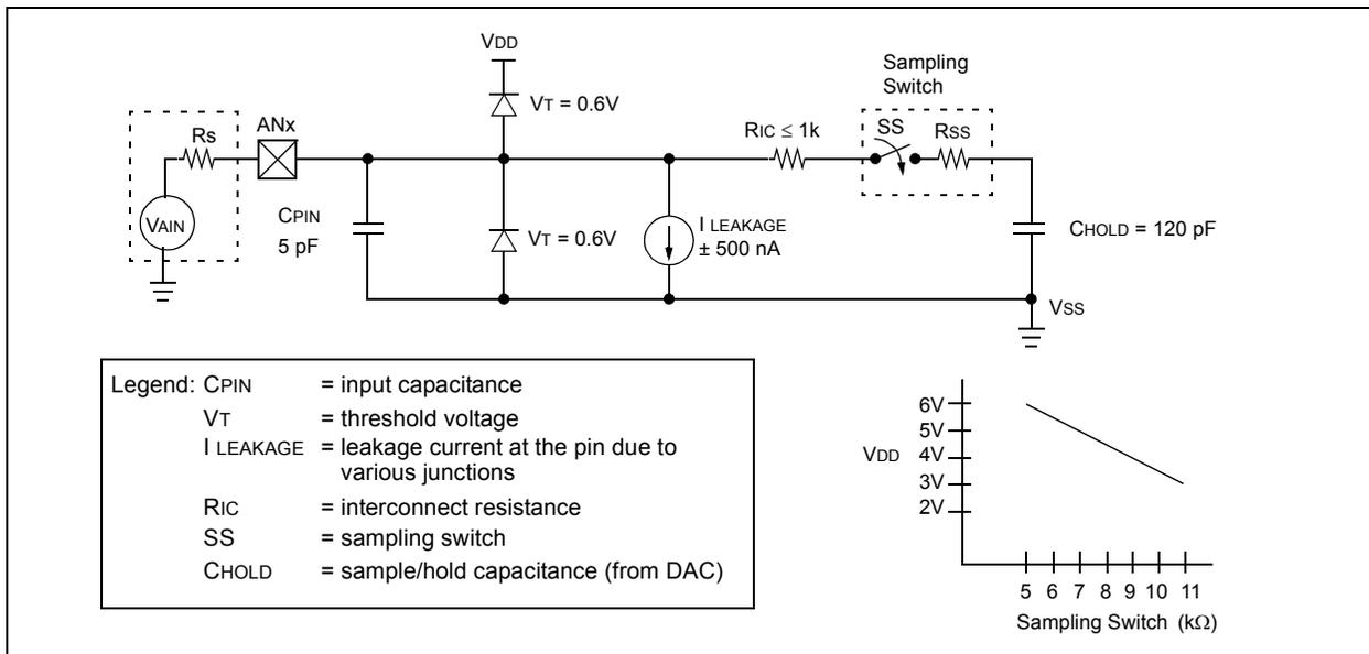
To calculate the minimum acquisition time, Equation 18-1 may be used. This equation assumes that 1/2 LSB error is used (1024 steps for the A/D). The 1/2 LSB error is the maximum error allowed for the A/D to meet its specified resolution.
