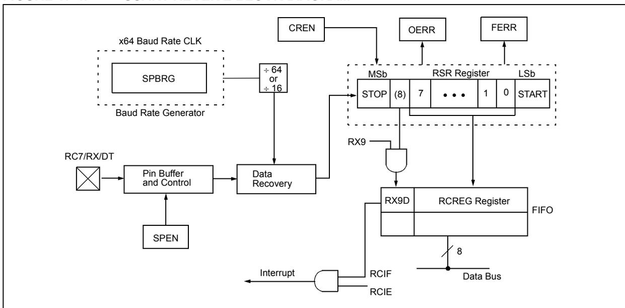
**FIGURE 17-5: ASYNCHRONOUS RECEPTION**
