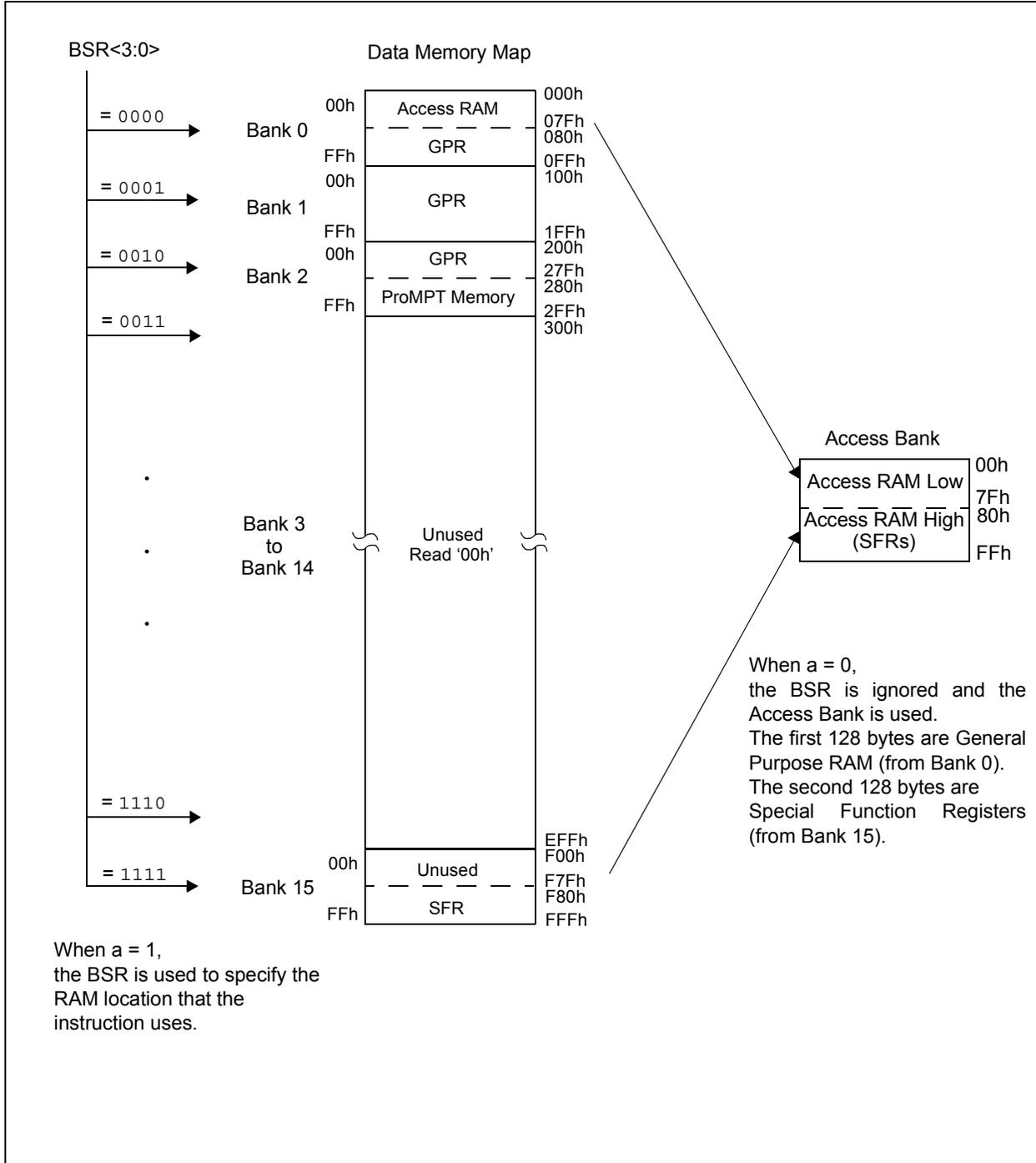
**FIGURE 4-6: DATA MEMORY MAP FOR PIC18FX539**
