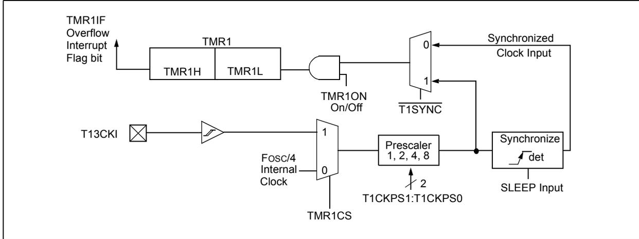
**FIGURE 11-2: TIMER1 BLOCK DIAGRAM: 16-BIT READ/WRITE MODE**
