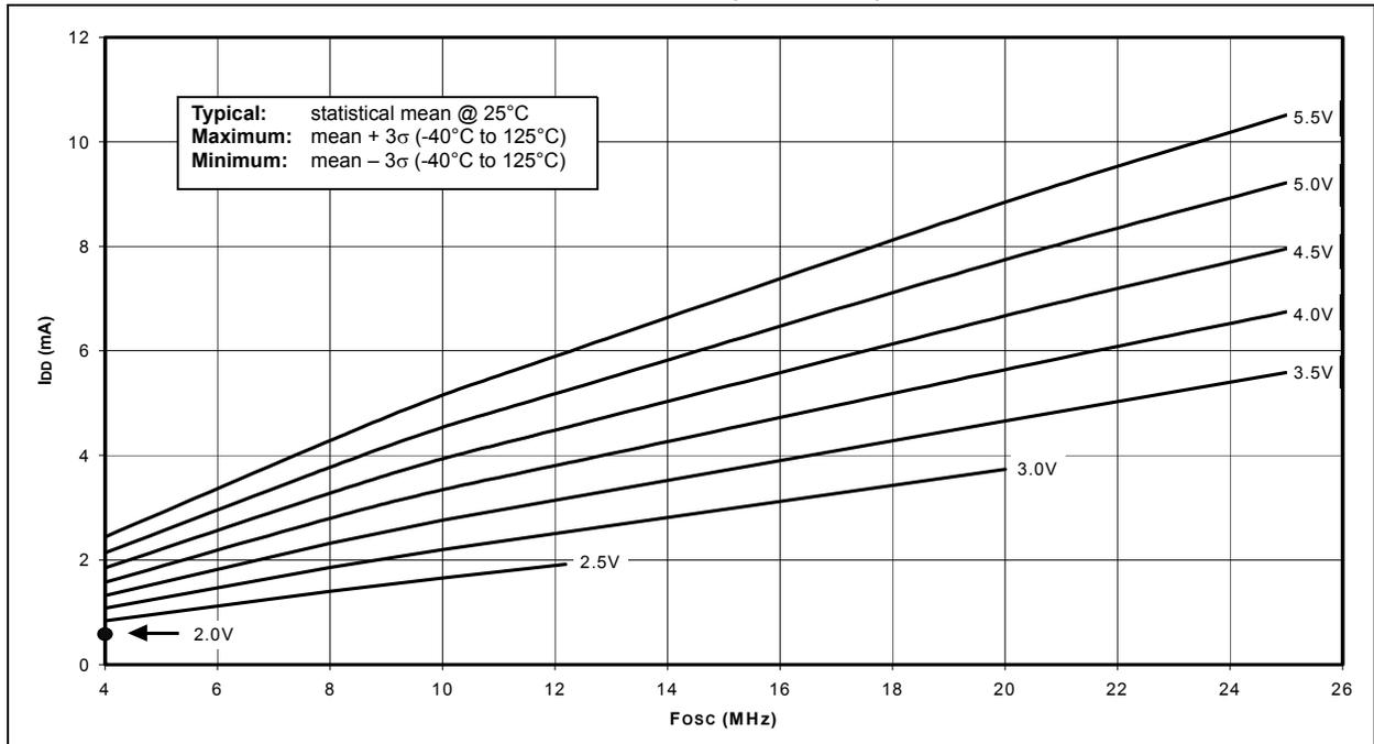
**FIGURE 24-2: MAXIMUM I<sub>DD</sub> vs. F<sub>osc</sub> OVER V<sub>DD</sub> (HS MODE)**
