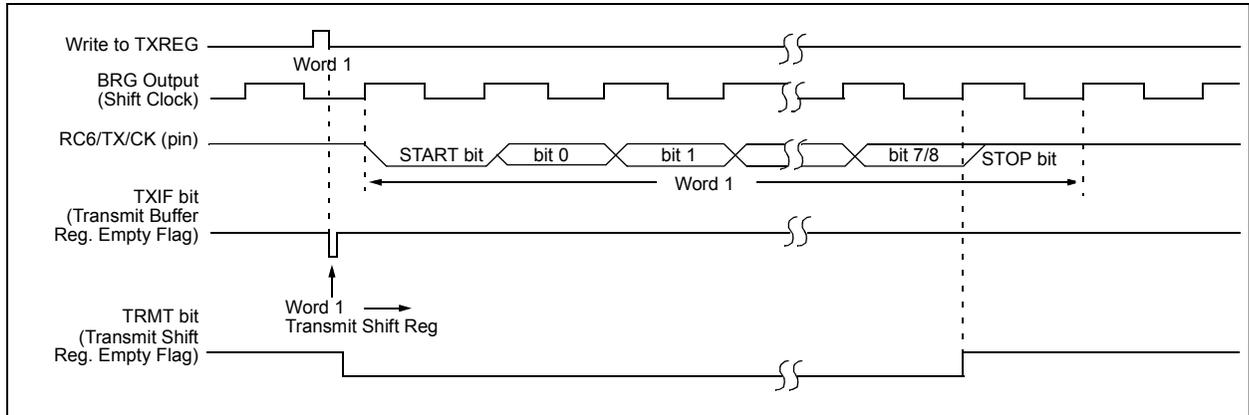
**FIGURE 17-3: ASYNCHRONOUS TRANSMISSION (BACK TO BACK)**
