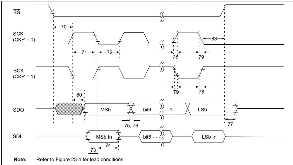
**TABLE 23-13: EXAMPLE SPI MODE REQUIREMENTS (SLAVE MODE TIMING (CKE = 0))**
