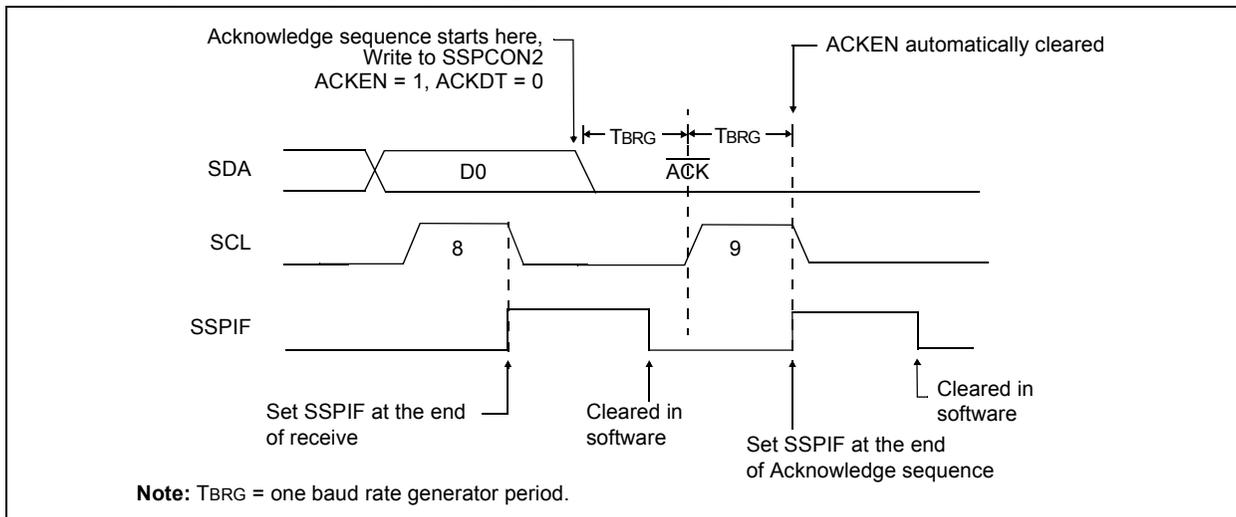
**FIGURE 16-24: STOP CONDITION RECEIVE OR TRANSMIT MODE**
