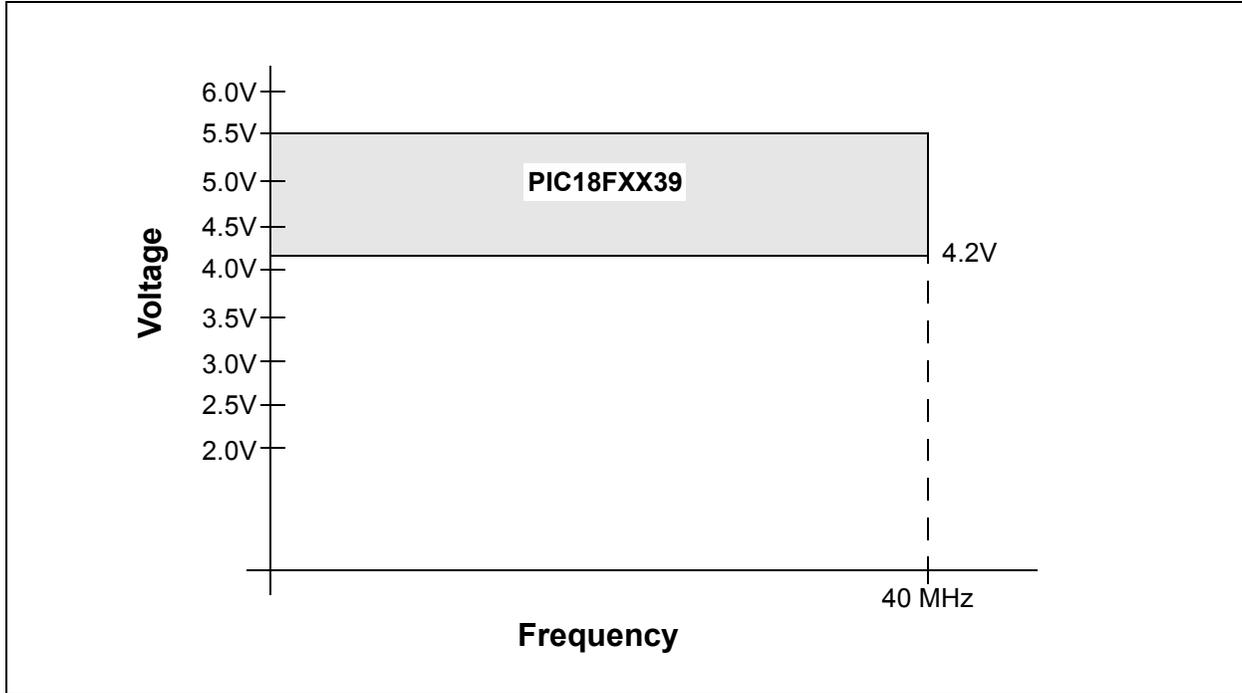
FIGURE 23-2: PIC18LFXX39 VOLTAGE-FREQUENCY GRAPH (INDUSTRIAL)
