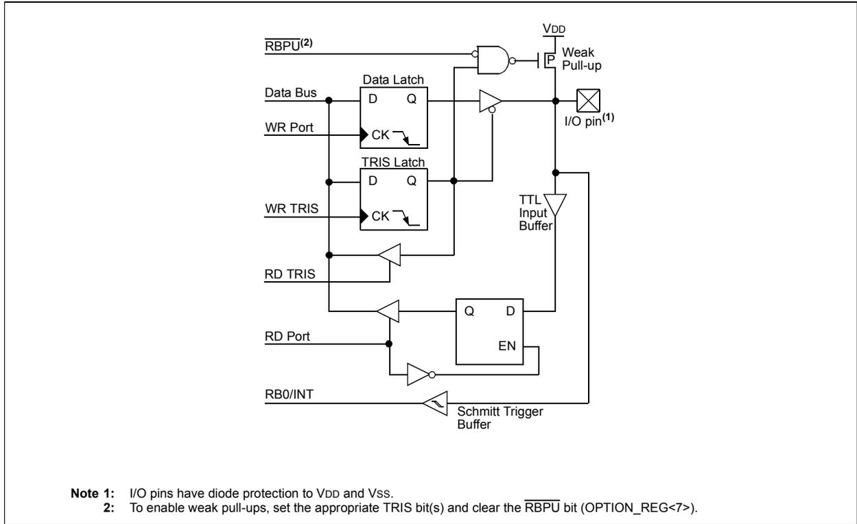
**FIGURE 9-6: BLOCK DIAGRAM OF RB3 PIN**
