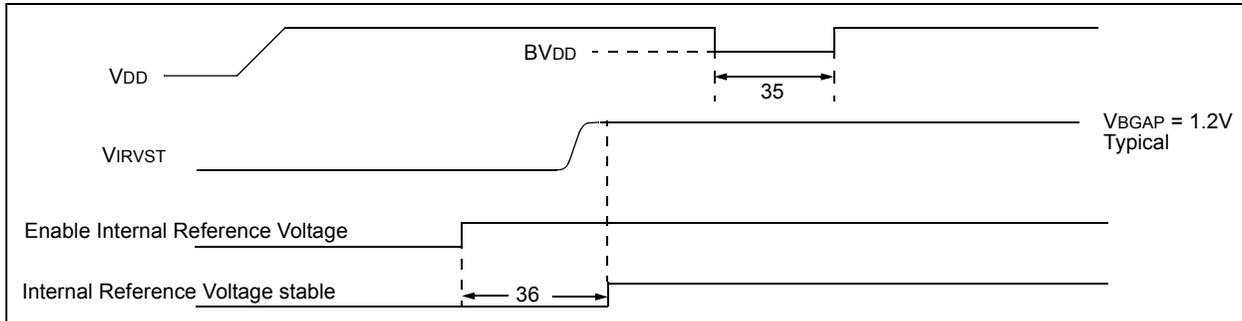
**TABLE 23-7: RESET, WATCHDOG TIMER, OSCILLATOR START-UP TIMER, POWER-UP TIMER AND BROWN-OUT RESET REQUIREMENTS**
