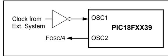
The ECIO Oscillator mode functions like the EC mode, except that the OSC2 pin becomes an additional general purpose I/O pin. The I/O pin becomes bit 6 of PORTA (RA6). Figure 2-4 shows the pin connections for the ECIO Oscillator mode.
