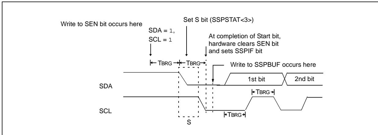
19.4.9 I<sup>2</sup>C MASTER MODE REPEATED START CONDITION TIMING
