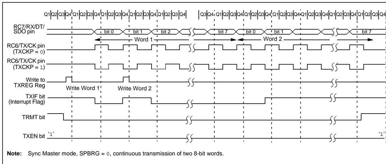
FIGURE 20-12: SYNCHRONOUS TRANSMISSION (THROUGH TXEN)
