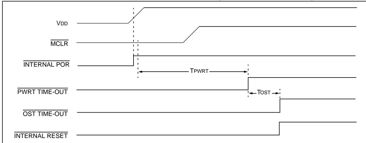
**FIGURE 4-5: TIME-OUT SEQUENCE ON POWER-UP ( $\overline{\text{MCLR}}$  NOT TIED TO  $V_{\text{DD}}$ ): CASE 2**
