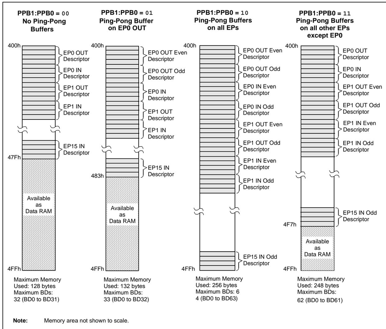
**TABLE 17-4: ASSIGNMENT OF BUFFER DESCRIPTORS FOR THE DIFFERENT BUFFERING MODES**
