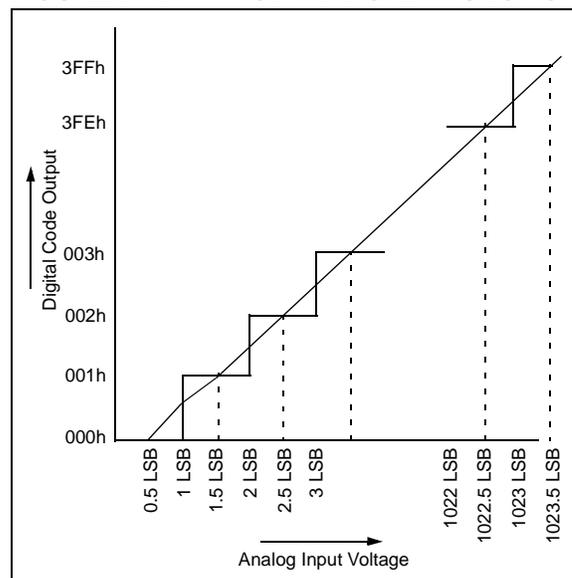
**FIGURE 21-3: ANALOG INPUT MODEL**
