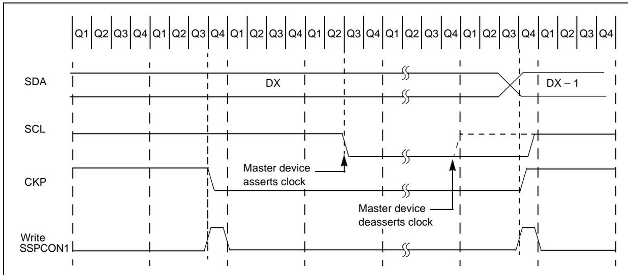
FIGURE 19-15: I<sup>2</sup>C™ SLAVE MODE TIMING WITH SEN = 1 (RECEPTION, 7-BIT ADDRESS)
