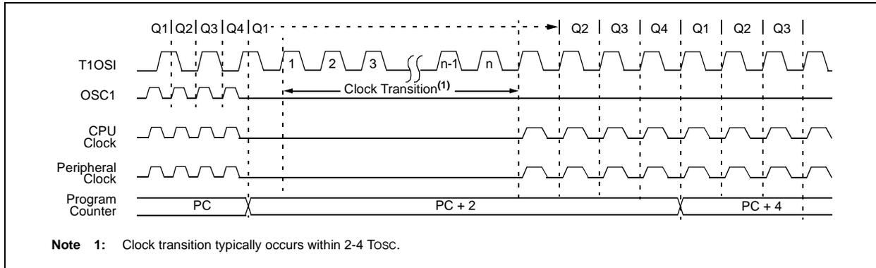
**FIGURE 3-2: TRANSITION TIMING FROM SEC\_RUN MODE TO PRI\_RUN MODE (HSPLL)**
