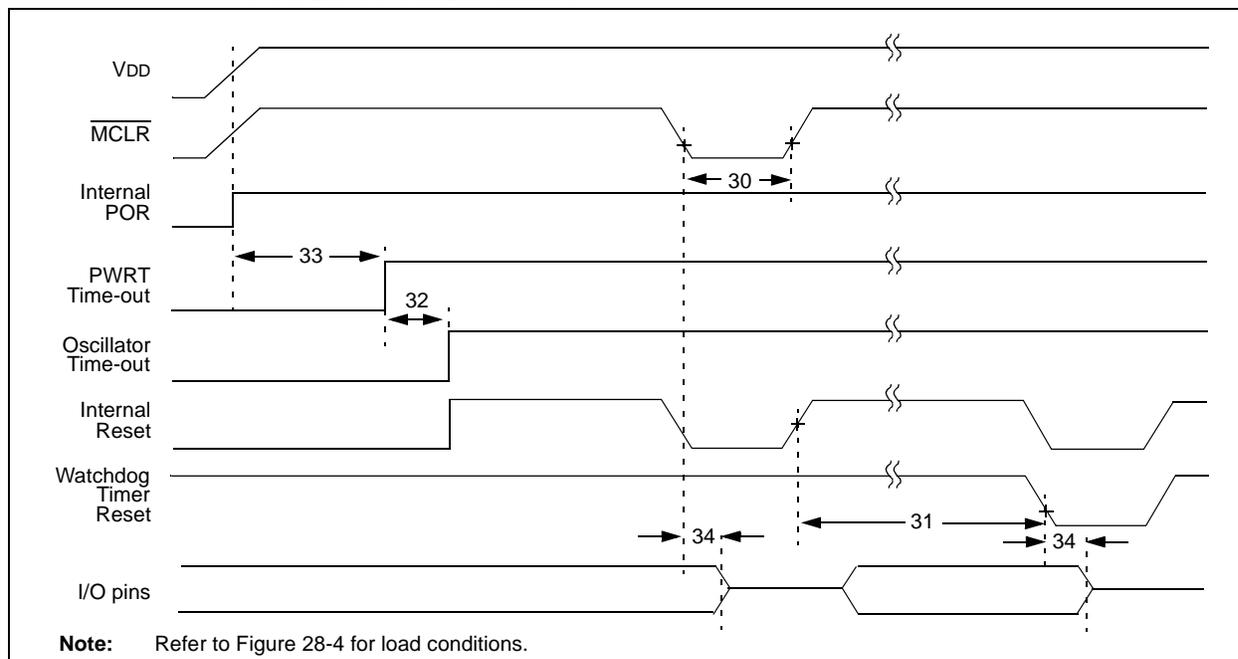
**FIGURE 28-8: BROWN-OUT RESET TIMING**
