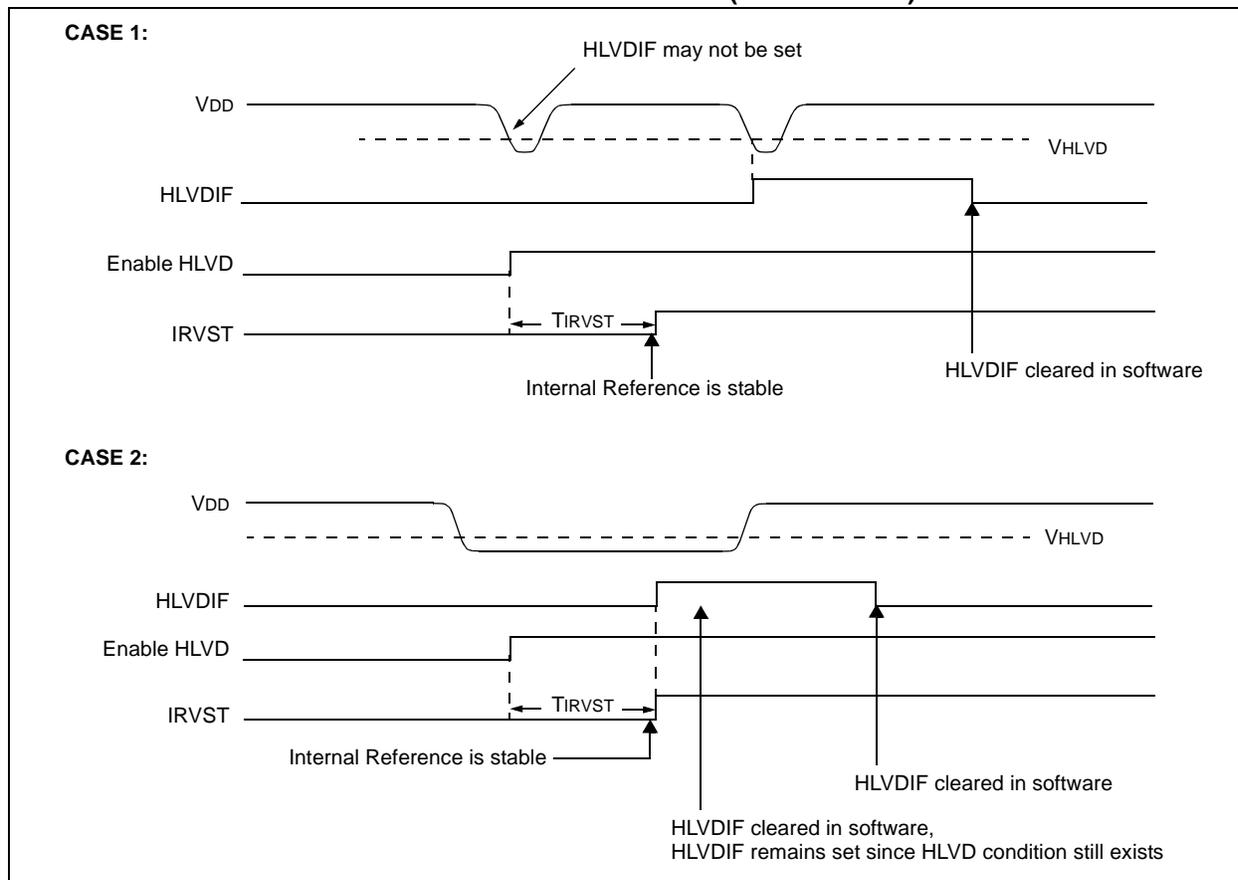
**FIGURE 24-3: HIGH-VOLTAGE DETECT OPERATION (VDIRMAG = 1)**
