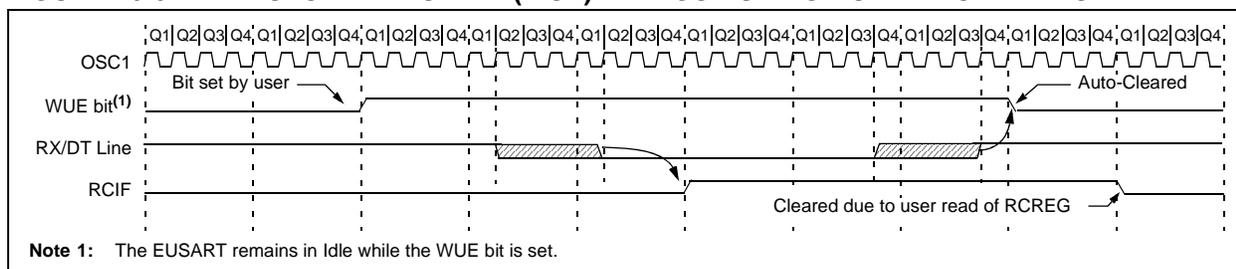
**FIGURE 20-9: AUTO-WAKE-UP BIT (WUE) TIMINGS DURING SLEEP**
