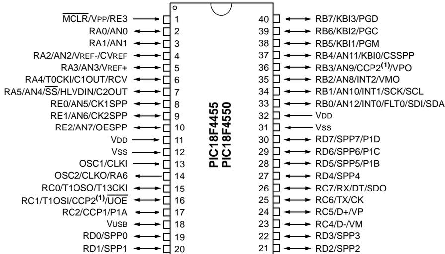
Note 1: RB3 is the alternate pin for CCP2 multiplexing.
