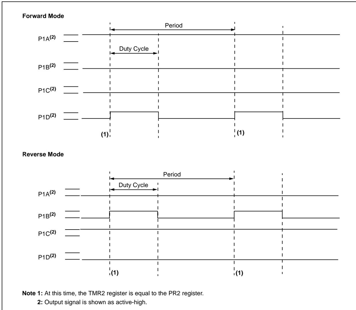
FIGURE 16-7: EXAMPLE OF FULL-BRIDGE APPLICATION
