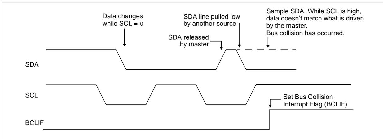
19.4.17.1 Bus Collision During a Start Condition
