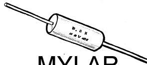
MYLAR (POLYESTER) AXIAL CAPS 125° C 10% tolerance non-polarized (more stable than aluminum electrolytics)
